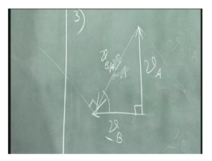
For example if I know the angle of this, I need to let's say I have the angle of this. Then I can say  $V_A$  by sine of this angle is equal to  $V_B$  by sine of this angle. This is equal to  $V_B$  with respect to A by sine 90. If I can get easily quantities that I need. Usually these are the ways in which people solve the problem.
