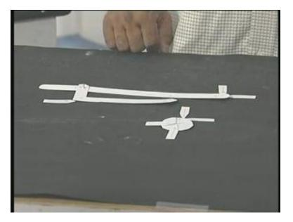
Now if you look at it, I have a force over here let me retain that force. There is another force on this. If I have to remove A E B now, I have to remove the restrain here. When I remove the restrain here, I need to add the two restrains related to that and this is the free body diagram of B C D.
