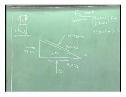
There is a resistance in terms of the normal reaction which is 21 kilo Newton's. Remaining 4 if is taken by the frictional force then the block cannot be moved by 25 kilo Newton's. I need to overcome the frictional forces in order to do that. But the frictional forces themselves account for around 18 kilo Newton's. So in which case if I have to move this, apart from this 21 adding 18, roughly I should have 40 kilo Newton force in order to move the block up.
