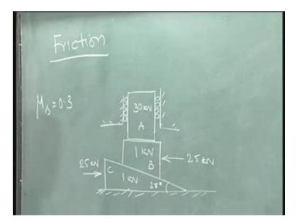
Now there are other parameters given for example the static friction coefficient between all the contact surfaces. I presume the contact surface is between A and B, B and C and C
