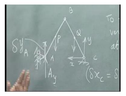
How do I find out delta  $y_P$ ? Since it is at center, I average delta  $y_A$  and delta  $y_B$ , I will get for this. I will average delta  $y_B$  and delta  $y_C$ , delta  $y_C$  is 0 and therefore delta  $y_B$  by 2 will be automatically delta  $y_Q$ . That's what I am going to do next, delta  $y_P$  is equal to, since it is midway delta  $y_A$  plus delta  $y_B$  by 2 and that is equal to delta  $y_A$  plus half of delta  $y_A$  divided by 2 and that is 3 by 4 delta  $y_A$ .
