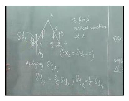
Why did we look at delta  $y_A$ , delta  $y_Q$ ? Because those are the active forces for which we need to find out. What is the direction of these? This is upward direction, this is upward direction because they are positive notions.
