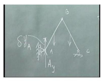
Let me give a virtual displacement here, I am going to give a direction and this is delta y at A. Now I am not done something. What is that? I have to fix the reference coordinates, I know this is a fixed frame of reference and therefore I will use this as a positive notion,
