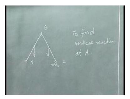
I need to now give a virtual displacement. It is not necessary I have to give a virtual displacement here, I can give virtual displacement at any point. This is a difficulty you will face, you can give it at any point, and it does not matter. You will get the same equation of equilibrium. For now let me just give a vertical displacement here and find out the appropriate virtual displacements.
