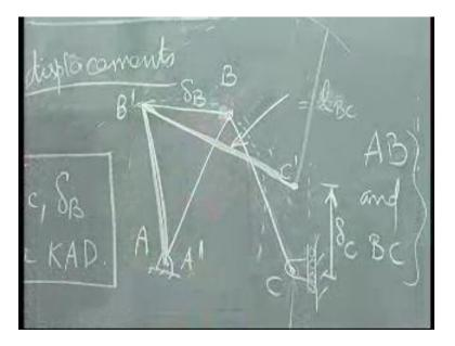
Therefore the bottom line is I need to find out the displacements at each of the salient points of the rigid bodies. Sometimes I may have a hinge, this may be extending like this. So it's better that I find out here because this is connected at this point. As long as this is clear we should be able to solve this problem.
