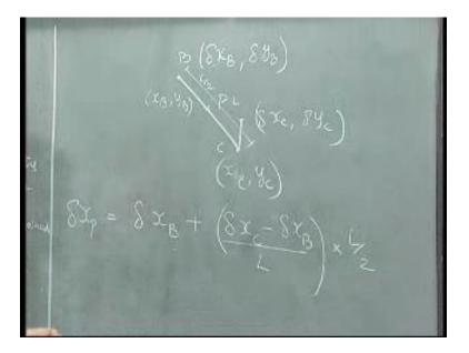
Similarly if I have to find out the virtual displacement in the y direction, I will get it to be delta  $y_B$  plus delta  $y_C$  divided by 2. Reason why I am telling you this is, it may be worth it finding out the displacements of the ends of these bars.
