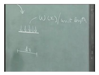
This is the external force that is acting transverse in direction. Now let's draw the bending moment, this as a negative sense like this and therefore we will have this is the positive sense of the shear force V at x and bending moment will be like this which is M at x. Since we have cut this side also, we have moment and shear force. This is M at x plus dx because I am taking dx away from this in the positive direction and this shear is V, at x plus dx.
