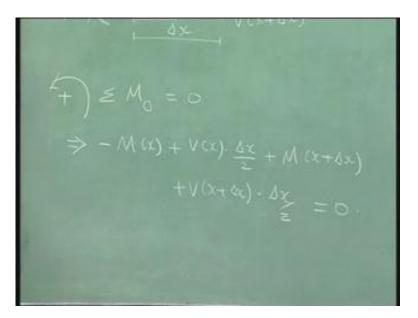
Notice that we have M of x plus delta x minus M of x. Let's write it down, M of x plus delta x minus M of x plus (V of x, V of x plus delta x) V of x plus V of x plus delta x both multiplied by delta x by 2 is equal to 0. Dividing throughout by delta x, we will have M of x plus delta x minus M of x by delta x by 2. I am going to divide by delta x by 2 is equal to, I am going to take to the right hand side minus V of x minus V of x plus delta x.
