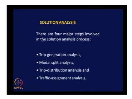
And the analysis phase involves as I mentioned 4 important steps; trip generation analysis, model spilt analysis, trip distribution analysis, and traffic assignment analysis
