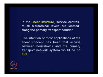
In the case of linear structure, service centres of all hierarchical levels, as all we have seen, are located along the primary transport corridor. The intention of most applications of the liner concept has been that access between households and the primary transport network system would be on foot because it is linear. It is assumed, that people can just walk and reach out to the main corridor; that, was the understanding.
