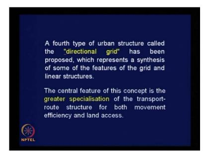
Of course, the 4th type of urban structure, called the directional grid has been proposed, which represents the synthesis of some of the features of the grid and linear structures, as we have seen earlier. And the central feature of this concept is the greater specialization of the transport route structure for both, movement efficiency and land access, as we have seen.
