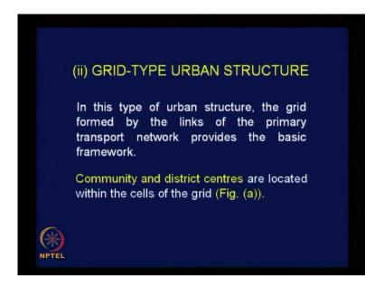
Then, the next type of urban structure namely, grid type of urban structure. As the name implies, the gird formed by the links of the primary transport network, links of the primary transport network, provides a basic frame work for the grid. You can understand the primary transport network as the links of type 1 category roads in our hierarchy, namely expressways, clear.
