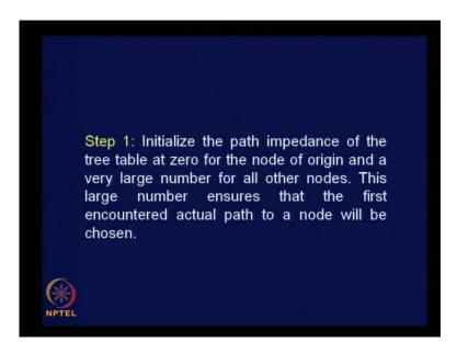
Let us again, recapitulate step 1 we are initializing the path impedance of the tree table at zero for the node of origin which is node 1 and a very large number for all other nodes. This large number ensures that the first encountered actual path to a node will be chosen.
