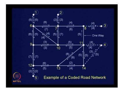
This is the network that, we are talking about nodes 1 2 3 and 4 as well as 5 are zone centroids. Other nodes are road intersections and there are two dummy links for zone centroid 4 and all other centroids have only 1 dummy link. Please try to capture this picture to understand the subsequent discussion clearly. Now our starting node is node 1 so we are trying to build minimum path tree for node 1, which is zone centroid 1.
