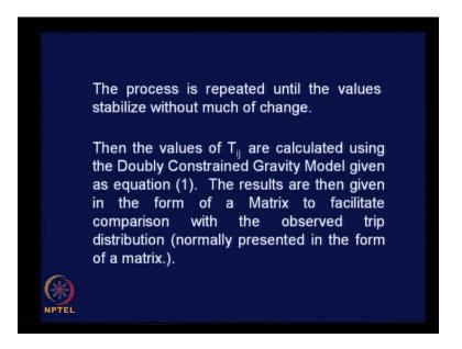
And this process is repeated until the values stabilize without much of change, when you repeatedly substitute for X i and Y j, you will find that at some point of time there is no change at all, it is stabilizing, then those values of X i and Y j are fit for substitution in the parent equation to get the value of T i j.
