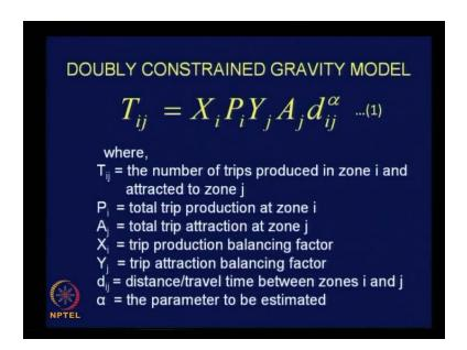
And it is possible to incorporate both the constraint at the initial stage itself and straight away do the distributions process without any iterative procedure involved in getting the trip distribution values, such a model is named as doubly constrained gravity model.
