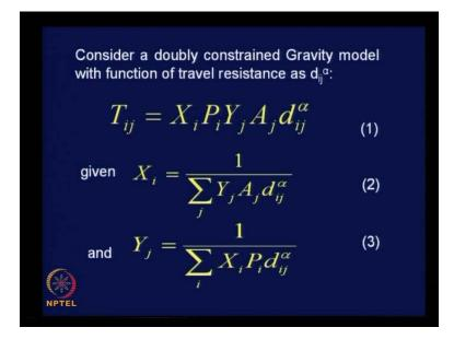
Now, let us consider a doubly constrained gravity model with function of travel resistance as d i j raise to power alpha, this is our consideration. We can consider different functional forms, in this case we just assume the frictional resistance to be following a simple polynomial form right, d i j raise to power alpha.
