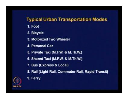
Let us try to list the different modes of transport available for urban transportation. The availability of or the categorization of modes is based on their technical as well as the level of service characteristics. Accordingly, we can classify the modes starting from Foot, Bicycle, Motorized two wheeler, Personal car, Private taxi, Shared taxi, Bus, Rail
