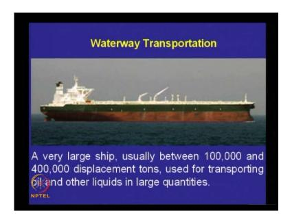
Development in water way transportation, the development is mainly in the size of the vessels that are sued for carrying fright as well as passengers. A very large ship usually between and 100 thousands and 400 thousands displacement tons, used for transporting oil and other liquids in large quantities. That is what is happening today bigger and bigger vessels to transport bulk commodities over long distance.
