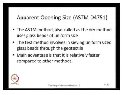
Let us look at the apparent opening size and the ASTM standard is ASTM D 4751, as noted and there are different methods for determining the opening sizes of the geotextile. The ASTM method, it recommends using glass beads of the uniform size for determining the apparent size and this is also called as the dry method basically because we do not use any water for performing this test.
