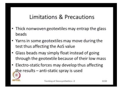
And this test is a very simple test and it does not take much time because for each size of the glass beads, it is only takes 10 minutes for this sieve shaking. And then we determine the mass of the glass beads, that are retained on the geotextile and passing through the geotextile. But, there are several limitations and we also need to take some precautions while doing the test so that, we do get consistent results.
