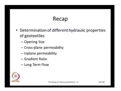
Just conclude, in this lecture we have discussed about the determination of different hydraulic properties of the geotextiles. That is, the opening size, the cross plane permeability, in plane permeability, the gradient ratio and an adaptation of this gradient ratio of long term flow. And once we have all these properties, we can properly select a geotextile for drainage and filtration applications.
