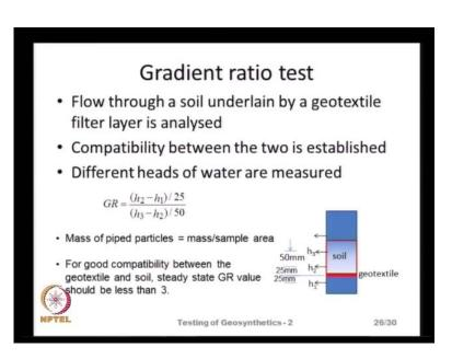
It is actually h 1, h 2, h 3 and so on and we can calculate the gradient ratio as the head difference between h 2 and h 1 divided by 25 millimeters, that is corresponding to the soil divided by h 3 minus h 2 that is, over a length of 50 millimeters in the soil and this particular formula is given assuming that, the geotextile thickness is very small. And if
