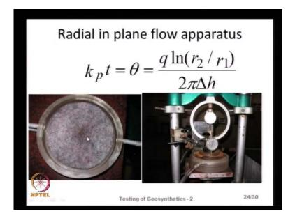
Whereas, in the case of very thick non woven geotextiles, like the one shown here, the flow could be more of radial type.
