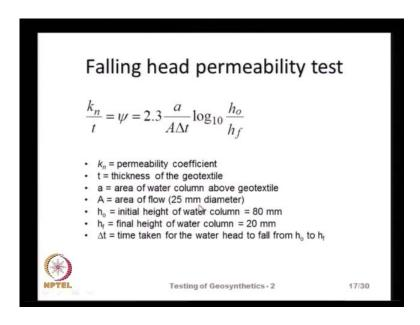
This capital A is the area of the flow that is, 25 millimeters that is corresponding to the internal diameter of the bottom shoe. And h naught is the initial height of water column that is, 80 millimeters and h f is the final height of water column that is, 20 millimeters and delta t is the time taken for the water head to fall from 80 millimeters to 20 millimeters. And based on all these values, we can determine the permeability coefficient or the permittivity site.
