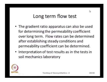
And a slight variation of the gradient ratio test is the long term flow test, it is actually here.
