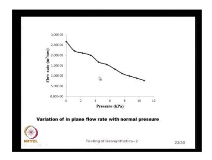
And for this particular geotextile that was used, this is how the inplane permeability coefficient changed with different pressures. When the test was repeated from 0 pressure to about 11 kPa pressure, continuously the permeability reduced and this particular one is for a jute geotextile. The Y axis, it has the flow rate and that can be converted to other properties like the k p or theta.
