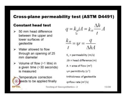
The q is the rate of flow in meter cube per second, it can be related to the permeability coefficient k n that is, the cross plane permeability coefficient multiplied by the hydraulic gradient i multiplied by the area of the flow. And the hydraulic gradient is nothing but the head difference divided by the thickness of the geotextile, because we are
