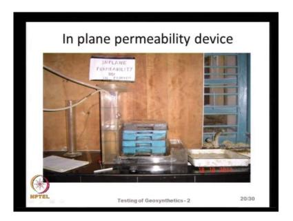
And natural operators is shown here, this is made of praspex, we have a column of water on the upstream side and then the column of water on the downstream side. And the water can freely flow out and the flowing water is collected in a pan. And we can apply the pressure on the geotextile, either through the dead white for very low normal pressures or through some other air or hydraulic actuator, in order to apply larger pressures.
