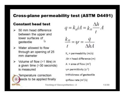
Let us now look at the permeability test and how to perform the permeability test on the geotextiles. The first one let us look at the cross plane permeability test and this is described by ASTM code D 4491 and the ASTM code recommends that, this test be done at either constant head or variable head. That is, the changing head of the flow and constant head test is performed at 50 mm head difference between the upper and a lower surface of the geotextile.
