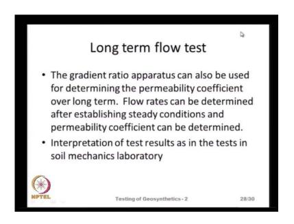
We allow the water to flow through and then we determine the rate of flow after a very long time, after the flow starts typically say, after 1 hour or 1 day or 7 days or so on. And then say, if we do the test for a very long time and if steady state conditions are established, the permeability constant that we calculate will reach a constant value. And
