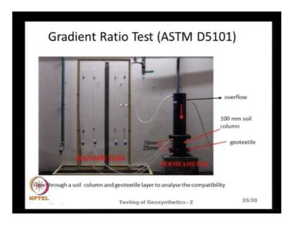
Then, another test that we perform a very important test is the gradient ratio test, originally this test was developed by the US army core of engineers. And later on, the ASTM has slightly modified and the ASTM code for performing this test is the ASTM D 5101. And the difference between the gradient ratio test and the other test is that, we employ the candidate soil where, we want to protect the, which are needs to be protected by use of geotextile in this test.
