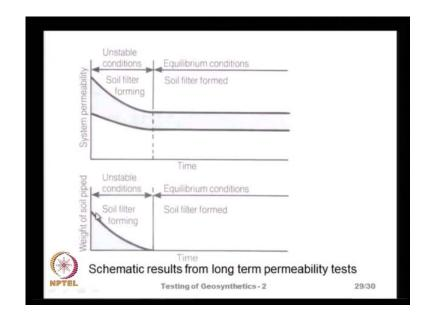
And if you plot a graph between the time and the system permeability or the weight or mass of the soil particle, piped soil particles, it is like this. Say, initially the permeability may decrease, because of the clogging of the geotextile with fine soil particles and after some time, once the steady state conditions are established. That is, when the soil filter cake is formed, the permeability remains constant or the flow rate remains constant.
