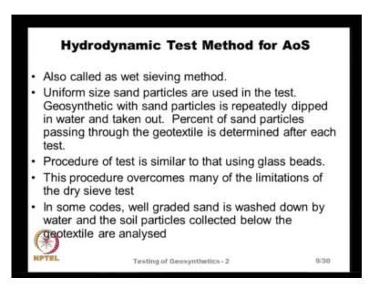
And in some codes especially, the ISO and the German codes, instead of using uniform size sand particles, they use a well graded sand, that is place on the geotextile.
