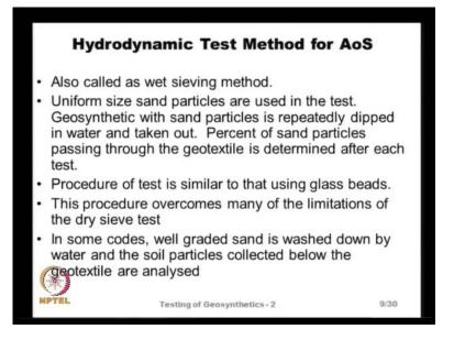
Another test method for determining he apparent size is the hydro dynamic test or the wet sieving method, just as how we do the wet sieving of the fine grain soils, we can use water and do this sieve test. And there are two methods once again, even in the hydro dynamic test, one is a procedure similar to the ASTM standard. Wherein, we use uniform sized particles and here, we sieve sand and collect uniform sized sand particles like 75 micron, 150 micron, 180 micron and then 225 micron and so on.
