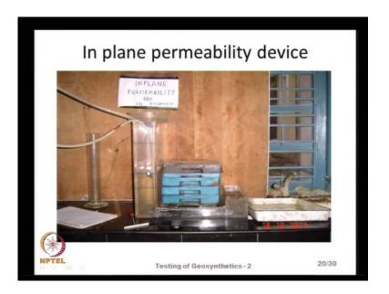
Whereas, this laminar flow operators is good for woven type geotextiles where, there is view pattern, which is continuous like there is a identifiable direction, that is the longitudinal and transverse strips and the flow is more or less along fixed paths, longitudinal and transverse.
