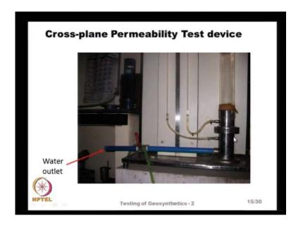
Another close up is here and the water is allow to flow out and we collect the quantity of water in a bucket in a given time and let us look, how to interpret the test result.
