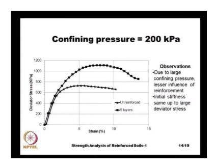
And now, let us look at the same data when the test was performed at much higher confining pressure 200 kPa. And here, just for illustration purpose I am showing only two graphs, one corresponding to the reinforced soil and the one other corresponding to five layers. And here, the one thing that we notice is that, the slope of the unreinforced soil and the reinforced soil with five layers is almost the same upto nearly 600 kPa pressure.
