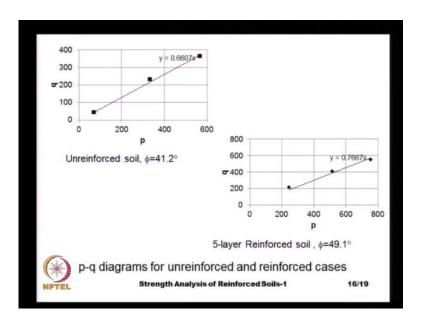
Because, as we see here, this is a regression line and this regression can be either done in a computer program or even now a days, even in the small calculators also, we can do the regression and the interpretation of the p q diagram is slightly different.
