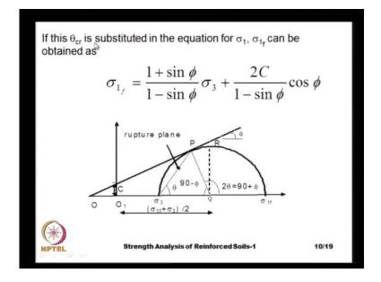
So, and if this theta c r is substituted in the equation for sigma 1 that is, if we substitute this theta c r in this equation for sigma 1 and simplify, we get a relation that, sigma 1 failure or sigma 1 maximum is 1 plus sine phi by 1 minus sine phi sigma 3 plus 2 C by 1 minus sine phi cosine phi. And here, the point P actually has the maximum obliquity, see in this Mohr circle, the maximum shear stress is QR and at point P, the shear stress is less than this but then, the failure happens here.
