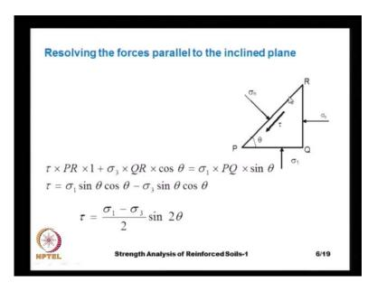
And by resolving the forces parallel to the inclined plane PR, we get the tau times PR times 1 plus sigma 3 because that is acting in the direction of the tau, sigma 3 times QR times cosine theta that is equal to sigma 1. That is the major principle stress multiplied by PQ, the length on which the stress is acting multiplied by sin theta. To resolve it
