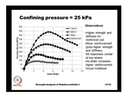
That is, in this case, when the test was done at 25 kPa and the difference between the unreinforced soil and the reinforced soil is say, here the unreinforced soil is failed at a deviator pressure of nearly 90 kPa and the reinforced soil with five layers, it has failed at
