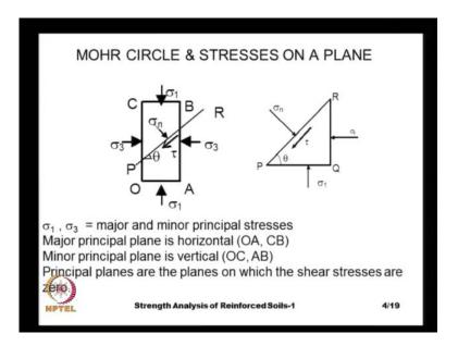
And let us take some arbitrary plane PR, that is inclined at an angle of theta to the major principle plane. And let us determine the sigma n, that is the normal stress acting on this plane and the shear stress tau, that is acting along the length of this shear plane.
