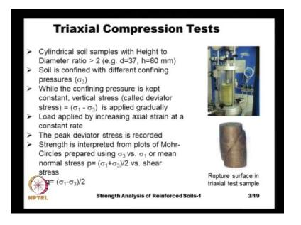
Because, we know that, we have seen earlier that, the failure happens along a particular plane, on which the maximum obliquity between the shear stress that is acting on that plane and the normal stress happens.
