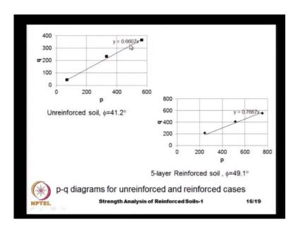
It is actually here, we see the p q diagram that is, the p is the mean normal stress on the x axis and the q is the shear stress on the y axis. And here, just for simplicity, I am showing only three data points corresponding to confining pressures of 25, 100 and 200, and the slope of this line is 0.66 and the friction angle, the phi is sin inverse of this. And it is actually, this line is forced to go through the origin because we have used basically dry sand, which has no cohesive strength.
