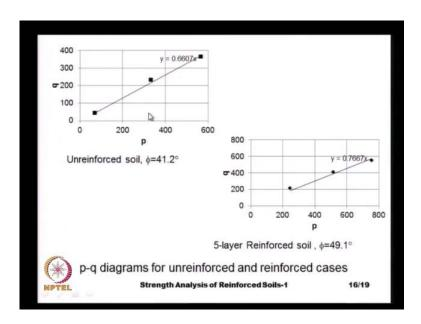
And here, we have only interpreted by drawing the p q diagrams for simplicity and now, we see that, the friction angle of the unreinforced soil is 41 degrees and the friction angle of the reinforced soil is 49 degrees.
