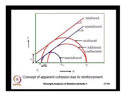
The internal reinforcement layers, they support the soil and because of that, the confinement pressure sigma 3 has increased to sigma 3 plus delta sigma 3 and that leads to a higher sigma 1 that is, the higher axial stress. So, we get a larger Mohr circle or other way of looking at it is, you assume that, the sigma 3 remains constant but then, there is some apparent cohesion the C, because of that which the axial stress increases to to sigma 1.
