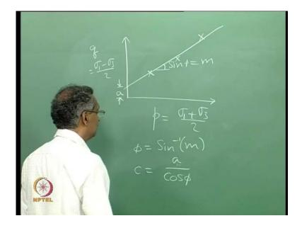
Let us say that, we have some test data and we can always do some regression and plot a best fitting line through all the data points. And they intercept is a and this slope is sin phi say, if this slope of the line is m, the phi can be interpreted as sin inverse of m. And if a is the intercept, this c is a by cosine phi, these theoretical relations can be derived from the fundamentals by drawing the p q line or the Mohr circles.
