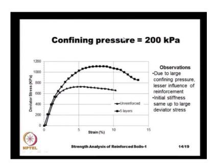
And then, at some stage, the peak stress has developed and in this case, the difference between the peak stress of the unreinforced soil and the reinforced soil is not as much lesser as compared to the earlier case.
