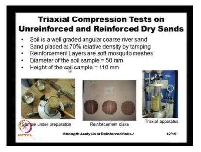
Let us look at some triaxial compression test data and both unreinforced and reinforced dry sands because here we use dry sands because typically in the reinforced soil structures, we use soils that are very well draining. That means, that we have to use coarse grained soils like sand or some aggregate or gravel and so on. And in this particular case, just for demonstration, we have used dry sand and the particular soil that is used is a river sand.
