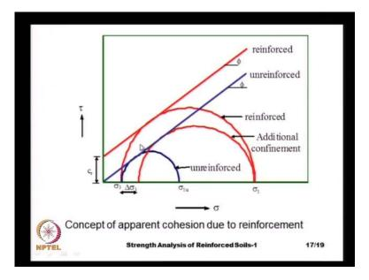
And now, let us do some analysis on this increased strength, this blue circle is the Mohr circle for unreinforced soil and this red circle is for the reinforced soil, which has failed at a much higher axial stress sigma 1. And we can also think of the increased axial stress, as because of the increase in the confinement pressure. And there are different concepts
