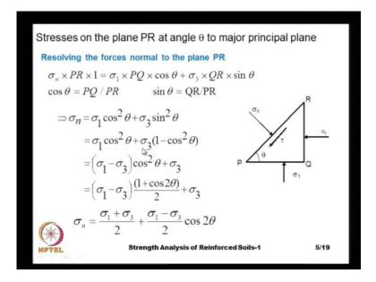
And this particular wedge, it has the forces or the stress sigma 1, sigma 3 and then, the tau and sigma n and by resolving the forces normal to the plane of the PR that is, in the direction of the normal stress sigma n. And by considering a unit length in the perpendicular direction to the plane of the analysis, sigma n multiplied by PR, that is the
