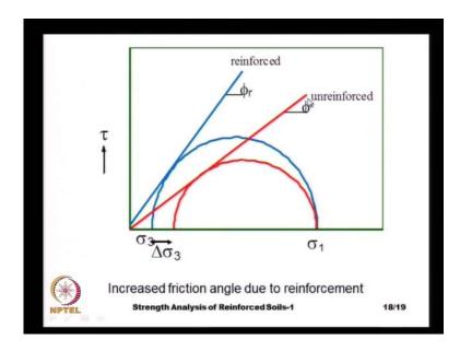
The other way of interpreting this result is like this, the phi that is the strength of the unreinforced soil and the increased slope is the slope of the reinforced sand, that is with a friction angle of phi r. And see these actually, what we do is, we assume that the reinforcement is increasing the confinement pressures, just as what happens when we construct an external retaining wall that laterally supports the soil.
