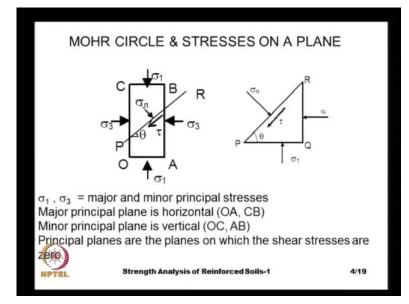
Before we actually analyze, let us look at the Mohr circle and the stresses that are acting on the cylindrical sample and on any arbitrary plane, that we have. And here, the stresses that are acting are the sigma 3 that is, we call it as a minor principal stress because that is smaller than the vertical stress that we apply. And then, the other one is the sigma 1, that we call as the major principle stress or the vertical stress.
