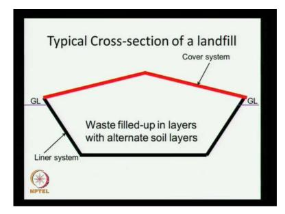
A typical transaction of landfills is like this, it is a highly simplified pictorial representation it does not include all the components, but that we will see later on. Let us say that, we have a ground level somewhere here we execute we make a depression. In this picture, I have just shown one single slope, but depending on the depth of execution we could have multiple slopes like with several burns, so that it is easy for the transport vehicle to move on these slopes.
