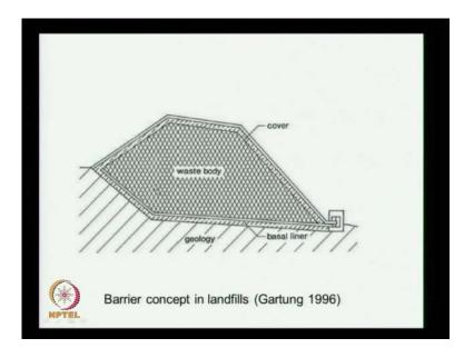
So, the typical construction is shown here, we have the waste body and we have the barrier and a liner system and the geological medium of the original soil here. Above the waste body, we need a cover system to prevent the odors from escaping into the environment or we need a system to collect all the gases that are produced, and safely dispose them off. Here, I will show you in a moment all the components of the landfills.
