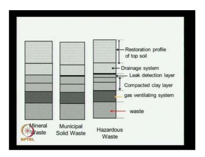
This picture shows different types of lining systems that we can have for the mineral waste for municipal solid waste and hazardous waste is actually the main components of all these landfills, we need a drainage system. We need a membrane and we need a compacted clay liner it acts as barrier. Sometimes, we can have a leak detection system especially when we are storing highly toxic waste, we need to detect any leakage, so that we can take some remedial action.
