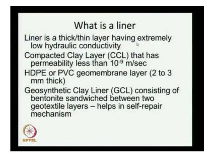
So, liner is a very important component of any landfill a liner is a thick layer that is if it is a clay layer it is thick and a thin layer, if it is a membrane or a geomembrane. The gallium usually about two and half millimeters thick or maximum 3 millimeters thick, and clay layer could be anywhere from half a meter to 1 meter thick compacted clay layer. This compacted clay layer should have a permeable to less than 10 to the power of minus 9 meters per second is highly impermeable.
