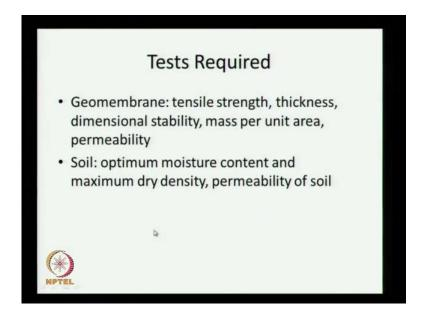
Some, of the tests that are required on the geomembrane are the tensile strength thickness dimensional stability, especially at high temperatures then the mass per unit area. The permeability of water and gases and on the soil we require optimum moisture content and a maximum dry density, the permeability of the soil and of course, the other properties like the grain size distribution and so on.
