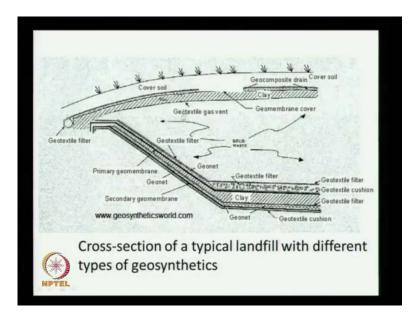
In this picture, we see a typical transaction of a landfill that has both liner and also has a cover. This particular one is downloaded from this web site and here, we see a typical landfill with cover and the cover is provided on top of this the waste. It consist of a cover soil so that we can grow some vegetation and then we could have a geocomposite drain, so that any surface water that enters it can be lead safely into some collection points.
