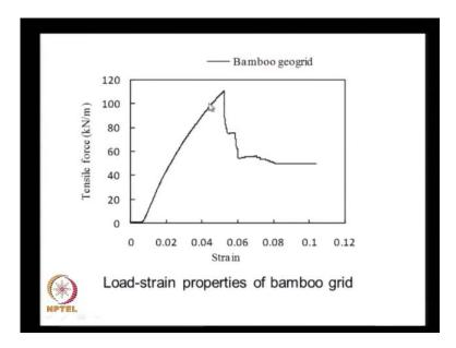
The tensile property of this bamboo geogrid is about 5 percent strain, it develops a force of about 110 kilo Newton's per meter. And it is a fairly good strength developed at relatively low strain and the result of encasement is quite substantial.
