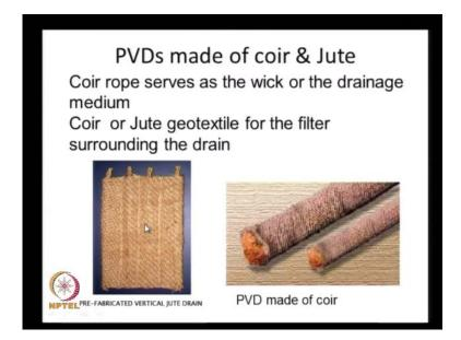
And the coir and the jute they can be employed for several applications. And here we see some products made for use in the pre-consolidation of soils and the PVDs prefabricated vertical drains. Here we see PVD made up of jute and coir is actual the coir wick is there that can transmit water and the jute filter cloth is surrounding this the drainage core to act as a filter.
