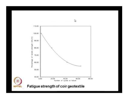
And the particular geotextile that we have it is susceptible to repeated load applications, and the strength reduces from 100 percent to almost 55 percent after about 60 load
