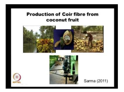
And the entire process is shown here, the coir fibre is obtained from coconut. And this is looks like this, husk surrounding the coconut fruit is the one that gives us the coir. It is mechanically the husk is removed and then by soaking in water that we call as retting process for about 6 months to 1 year period. The fibres separate out and then by some mechanical and labour intensive process the fibre is separated.
