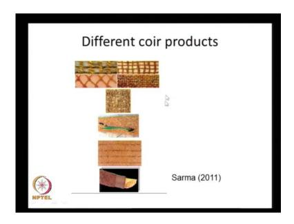
And some of the different coir products we can have nets or we can have a textile. This is a cocolog, this is a nonwoven textile and this is a pre-fabricated vertical drain.
