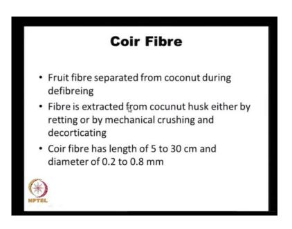
The coir and jute they are very important for the Indian economy because India is the largest producer of both coir and jute. And coir fibre itself is obtained from the coconut by defibreing operations and the fibre is extracted from coconut husk either by retting, or by mechanical crushing and then decorticating process. And the coir fibre can have lengths anywhere from 5 to 30 centimeters and diameter 0. 2 to 0.8 millimeters.
