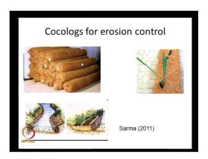
Cocologs is one of the more recent product. It is made in the form of a log, this entire log is made of coconut fibre and nonwoven or woven geotextile. And it floats in water and it can be employed in this systematic matter for river bank protection. If you provide it along the length of the river bank because of their flexible nature, they can take the shape of the river bank and absorb the way forces or water forces.
