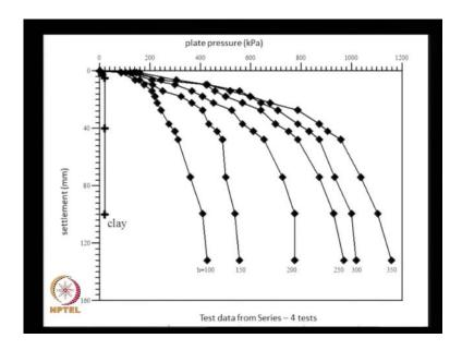
And this is the result from series 4 that is with 2 layers of enforcement.
