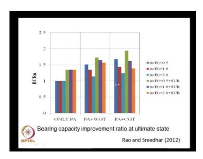
But if we see at the ultimate state where the retting is much higher, the coir geotextiles they have a higher bearing capacity improvement ratio as compared to the polymeric product. That is because at higher rut depths, the coir geotextiles is able to produce higher force because of better interaction it has with the surrounding medium.
