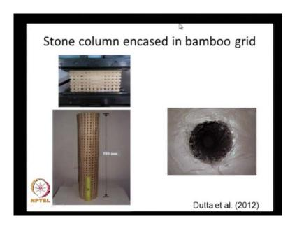
And another form of natural product is the bamboo. Recently there were some studies on the use of bamboo as a reinforcement. And here we see tensile testing of a bamboo geonet and here we see a tube that is made of bamboo net. This picture shows the reinforcement of a soft clay soil using a bamboo grid that is filled with stones, and this is similar to geosynthetics encased stone columns. Here we have a bamboo net that is encasing the stone column to improve its performance.
