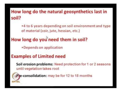
See one question that we need to ask ourselves is, our natural geosynthetics like the jute and the coir they have a limited life. They cannot stay in this soil for ever unlike, our synthetics counterparts like the geogrids and geotextiles made of say polyester or polypropylene or polyethylene, they can last for hundreds of years without any degradation whereas, the natural geosynthetics they have a limited life.
