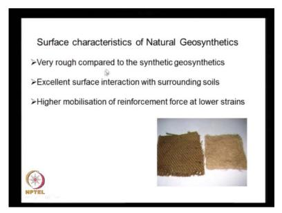
So, another characteristic of the natural geosynthetics that we can take good use of the surface character. The surface of most of the natural geosynthetics is very rough compared to their synthetic counterpart. And because of this roughness they have excellent surface interaction with surrounding soils, and that means that they can mobilize higher reinforcement force at a lower strain.
