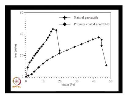
And this natural geotextile ((Refer Time: 27:25)) the geotextile, it is relatively soft textile. It provides or it develops maximum tensile force of about 36 to 37 kilo Newton per meter at a very large strain of nearly 40 percent, 42 percent and when it is treated with some polymer coating, we can make it stiffer. The strength as marginal increased to about 43 kilo Newton per meter and the strain at the peak load is about 16 percent.
