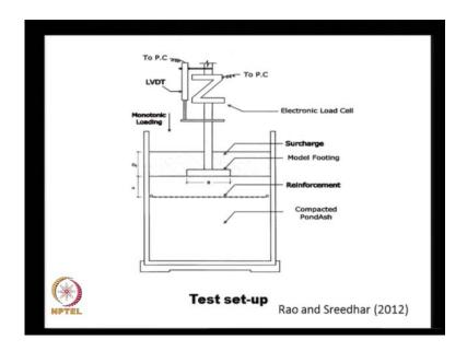
They have done a lot of laboratory test by using a compacted Pondash as the sub grid soil. And by placing the reinforcement at different depths, they have done this test.
