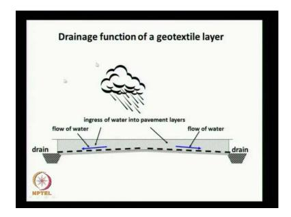
And typical illustration of the drainage function is shown here. Let us say that we have a highway pavement, and in spite of the fact that the surface is treated well with ashfault or bethermen, there could be some leakage through which the water can find its way into the pavement layer. And if we allow the water to propagate further, it will enter the sub drain and it
