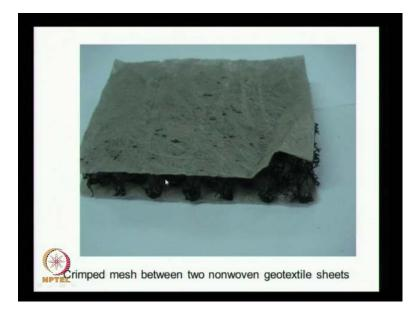
Here we have a another drainage material that is consisting of a crimped mesh as an inner core and geotextile layers surrounding it that act as a filter medium.
