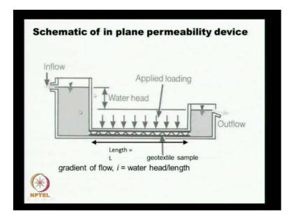
The capacity of our drainage medium is tested in the laboratory using in plane permeability device. In plane permeability device looks something like this. We have two water tanks that can provide some gradient hydraulic gradient. We provide or we place the drainage medium either a
