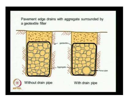
Another form of the paver drains are shown like this. We could have an aggregate fill and that is covered entirely with a geotextile filter so that the drainage medium is not contaminated or fill with fine aggregate or the fine soil particles. We can also have a porous pipe or perforated pipe. So, these are two different possibilities this is without a drain pipe and this is with a drain pipe.
