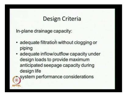
So, how do we design these drainage medium. See they should have adequate filtration capacity that will prevent the drain from clogging. In the earlier lecture, we have seen some requirements and what is a good filter and how to design it. And similar principles we can use even for designing the filters around a drainage medium. These drainage media should have adequate inflow and outflow capacity and the design loads, to provide for maximum anticipated seepage capacity during the design life.
