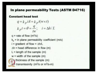
We can collect the water that comes out and we have a standard equation to estimate the flow capacity that is shown here. The ASTM test standard is ASTM D4716 that is to calculate the plane permeability or the permittivity of the geotextile or drainage medium. The q is the flow capacity, the K p that is the permeability tends i is the gradient or the hydraulic gradient multiplied by the flow area a, that is the width of the sample times the thickness and the K p times t is defined as theta.
