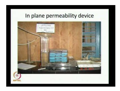
Here we see a photograph of the same apparatus. Here we have two water tanks and the geotextiles sample is placed inside. And if we have a small pressure to be applied, we can just simply use dead weights. If we want to apply very large pressure let us say 100 or 200 Kpa, we can have a pneumatic system. And we can place this entire apparatus in a loading device and apply higher pressures.
