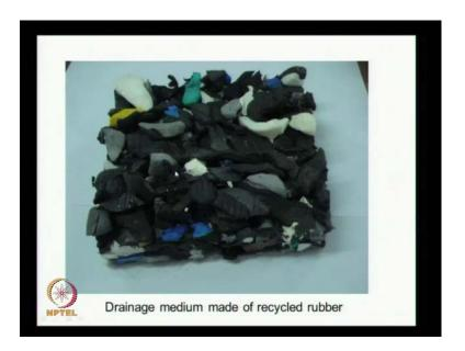
Here we see the recycled rubber being used as a drainage medium. These are all crimped or cut pieces of rubber which are joined together loosely, so that they have a very large void space and any water that enters here can easily flow because there is a large void space.
