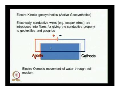
So, here the application is given like this and we have a new type of geosynthetics which are called as electro-kinetic geosynthetics. In some literature they are also called as active geosynthetics because they are doing some work. They are just not simply supporting the load passively, but they are actively doing some work by passing by passing current and by treating the soil. And similar to the woven fabrics and other fabrics we have electrically conducting geosynthetics.
