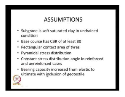
Some of the assumptions are the subgrade soil is saturated in undrained condition, and the base course aggregate has a CBR of at least 80, and rectangular contact area of the tyres, because they have considered the dual wheel configuration. And they assume that this rectangular contact area of 1 by b, just for simplifying the analysis.
