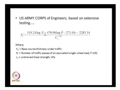
And here we have two more parameters N that is the number of traffic passes of a standard equivalent wheel loads, and then the P is the wheel load, and r is rut depth that is a given in terms of millimeters or centimeters and then the C u is the undrained cohesive strength of the subgrade soil. Either C u or CBR both are linearly related to each other. The C u is approximately 30 times the CBR in so many kilo Pascal units.
