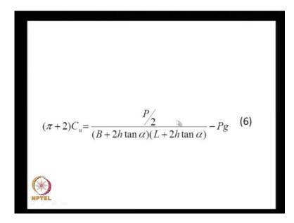
And by equating these two equations 4 and 5, we can get this equation the pi plus 2 C u is p by 2 times this whole quantity minus P g, where P g is the additional support that we get because of the provision of reinforcement.
