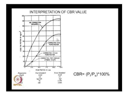
And we get a curve something like this. On the x axis, we have the penetration in millimeters, y axis the load in so many kilograms per centimeter square. And if you get a
