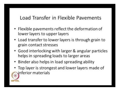
Well let us look at the load transfer in the flexible pavements. And the use of geosynthetics is more or a predominant use of geosynthetics is in the case of flexible pavements, because in the case of rigid pavements like reinforce concrete pavements, we may not require any geosynthetics. So, these flexible pavements, they reflect the deformation of the lower layers to the upper layers. That is because they do not have any flexural stiffness.
