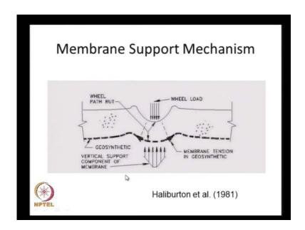
And another mechanism is the membrane support mechanism. When there is good rutting, the geosynthetic is subjected to some tension and vertical component of this tension force directly opposes the wheel load and that reduces the pressures, that are transferred into the subgrade soil; hereby increasing our long term performance.
