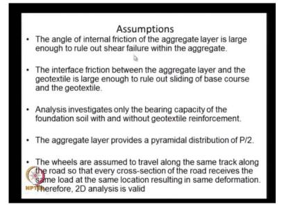
The other assumptions are that the only failure that they have considered is within the subgrade soil. The friction angle of the aggregate layer is assumed to be large enough to rule out any shear failure within the aggregate layer. And the interface friction between the aggregate layer and the geogrid or geotextile is large enough to rule out any sliding failure of the base.
