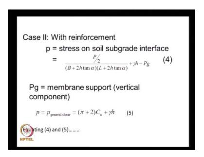
And the case two is with reinforcement. And here the pressure that is transferred into the subgrade soil is P by 2 by B plus 2 h tan alpha times 1 plus 2 h tan alpha plus gamma hits minus Pg, that is the membrane support that is given by the reinforcement. This is the vertical component and here now we assume general shear failure so that is 2 plus pi times C u that is our bearing capacity.
