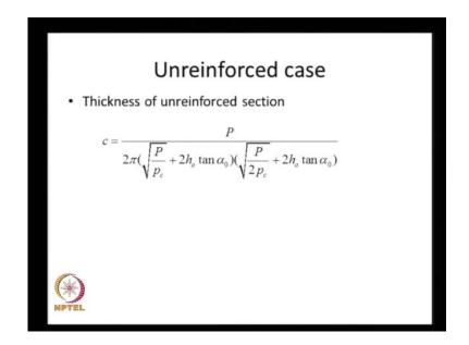
So, this same relation written in a slightly different form and here if we know the c that is the cohesive strength of the subgrade soil and the wheel load P, we can calculate h naught. (Refer Slide Time: 33:27)
