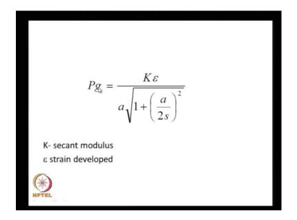
And this P g is the membrane support is related to the strain that is developed and the secant modulus like this. The strain developed is also a function of several other factors that we will see in a minute. The P g is written as k times epsilon by a times Square root of 1 plus a by 2 s times square.
