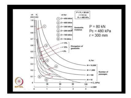
And Giroud and Noiray what they have done is, they have gone through this equation and they have developed a standard design slot, that gives the x axis the CBR value. The y axis the h naught prime, and the delta h for standard axle load of 80 kilo Newtons, and rut depth of 300 millimeters. The tyre pressure of 480 k P a for different modulus values of the reinforcement layers ranging from 10 all the way to 480 kilo Newtons per meter.
