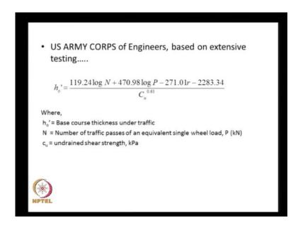
And by combining these equations, we can get a more generalized formula for calculating the thickness of the aggregate layer is h naught prime is equal to 119.24 log of N plus 470.98 log P minus 271.01 r minus 2283.34 divided by C u to the power 0.063 where, h naught prime is the base course thickness for so many numbers of passes and N is the number of traffic passes of axle load and then the C u is the undrained shear strength.
