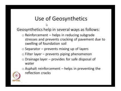
Let us now look at how we can use the geosynthetics in the case of flexible pavements. The geosynthetics we can use them in several ways, one is as a reinforcement layer. If we use as very stiff and strong reinforcement layer, it can help in reducing this subgrade stiffness and prevents the cracking of pavements due to swelling of the foundation soil. In case we have a highly swelling subgrade soil is going to undergo a lot of volume changes either heaving or shrinking.
