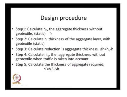
And the design procedure is very simple; we need to calculate h naught that is the aggregate thickness from one of the governing equations relating the stress, that is transferred into the subgrade soil by load dispersion through a height of h naught. And step two is to calculate the thickness of the aggregate layer with geotextile or the geosynthetic.
