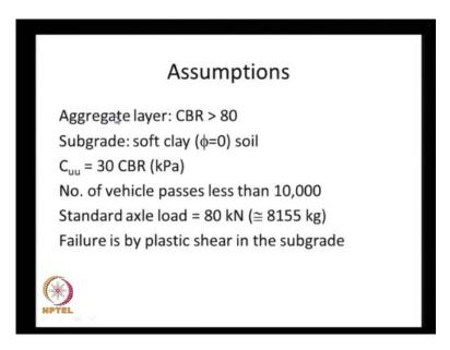
And some of the assumptions, the aggregate layer is assumed to have very high CBR value, that is CBR of more than 80 percent. Usually, the granular sub base material that
