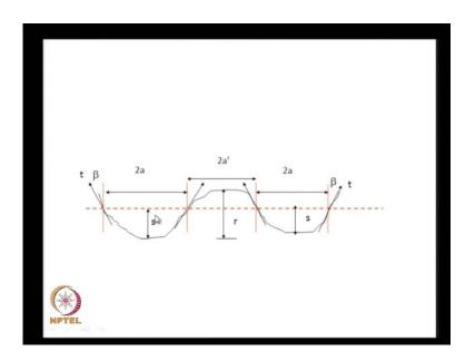
Where the s is the settlement below the wheels, and a and a prime these are just the curved length of the surface rutting.
