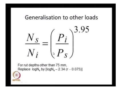
The Webster and his co workers, they have given an extra palation for other wheel loads and for any other load of P i, the number of load passes N i is related like this N s by N i is P i by P s to the power 3.95. Where, P s is the standard axle load of 80 kilo Newtons, P i is any other axle load and N i is the equivalent number of load passes as compared to N s.
