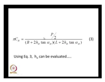
And by equating these two, we can get an equation in terms of the C u and the wheel load and h naught and by solving this h naught, we can get the thickness that we require. So, that the pressure that is transferred into the subgrade is less than the allowable bearing capacity of the soil.
