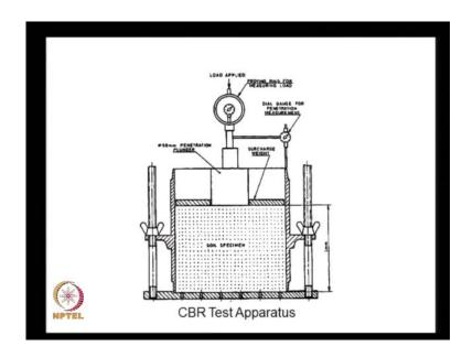
The design of the pavements is based on the CBR value, the California Bared Ratio and what you are looking at is the apparatus to perform the CBR test. We take a soil specimen compactor to the desired density at an optimum moisture contact, as we do it in site and then there is a standard way of applying the loads. And we have put some standard surcharge weight and then we apply the loading at a standard rate of loading.
