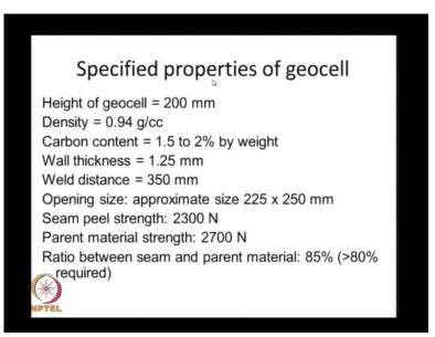
And the properties that are recommended for the geocell. The height of the geocell used was 200 millimeters. This is made of high density poly ethylene having a density of 0.94 the carbon content as about 1 and half to 2 percent. And the wall thickness is 1.25 millimeters and the weld distance 350 mm. These geocells they are made by cutting certain height of this geomembrane type of material. Then they are lied on top of each other and then they are ultrasonically welded at certain distances.
