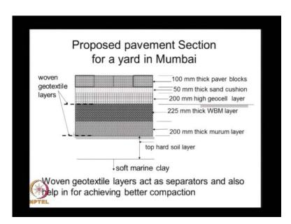
And this is the typical cross section that was proposed, the total pavement thickness that was pro provided was 1.5 meters out of that the top about 1 to 1 and half meters hard layer was used as part of the pavement. Then one woven geotextile layer was spread on top of the existing soil. And then 200 millimeters thick murum layer was compacted. And this particular geotextile layer here was provided not only to act as a separator, but also we need a good base so that we get a good compaction.
