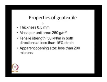
The properties of the geotextile that were recommended is thickness of half a millimeter and mass per unit area 250 grams per meters square. And the tensile strength 50 kilo Newtons per meter in both the directions at a strain less than 15 percent. And then the apparent opening size is less than 200 microns. So, that it can act as a good separator.
