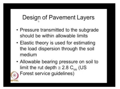
What is the philosophy that we use for designing the thickness of the pavement. The same thing just as how we have discussed earlier for the design of pavements below the roads, the same principle applies even for the container yard pavements, that the pressure that we transmit in to the sub grade soil should be with the allowable bearing pressure.
