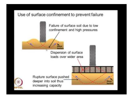
And the principle is very simple let us imagine that we apply some tire load on the surface, and immediately this results in failure of the surface soil because there is no confinement, there is significant heaven, and then we form the rapture surfaces. The failure happens because the surface soil has very low confinement at it is same time there is a very high pressure applied from the wheel from the tires.
