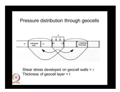
Let us say that this is our geocell layer and we apply the pressure. And there is a skin friction force that is developed on the cell walls, and because of that the pressure reduces and that is illustrated in the next slide like this.
