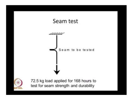
And the seam that is in the geocell is tested as per the ASTM standards. It should be apply to a static load of 72.5 k g that is for a width of 200 millimeters. This load should be kept constant for one week, that is 168 hours. And within that time this seam should not peel off. And that shows that the ultrasonic welding is of good quality. The geocell that we have is durable because some of the material that we have tested they have just
