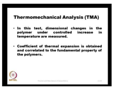
Thermomechancial analysis in this test, the dimensional changes in the polymer under controlled temperature increase is measured and the coefficient of thermal expansion is obtained and correlated to the fundamental property of polymers. Because, this coefficient of thermal expansion is a different for different type of polymers and by measuring this coefficient in this T M A, we can identify the polymer.
