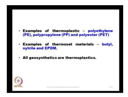
And some examples of the thermoplastics or the polyethylene, polypropylene and polyester and some examples of the thermoset materials are butyl nytrile, and EPDM and as I mentioned earlier all the geosynthetics are made of thermoplastic polymers.
