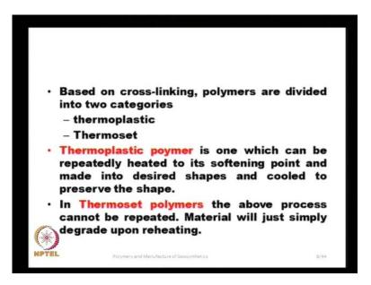
And based on the way the different monomers, they are linked together the cross-linking the polymers are divided into 2 fundamental categories, these are thermoplastic and thermoset. The thermoplastic polymer is the one in which this polymer can be repeatedly heated to its softening point and made into desired shapes and cooled to preserve the shape.
