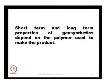
Why do we need to study about the polymers? Reason is both the short term and the long term properties of the geosynthetics depend very much on the type of polymer used for the manufacture of geosynthetics, and the manufacturing process that is used for fabricating the geosynthetic.
