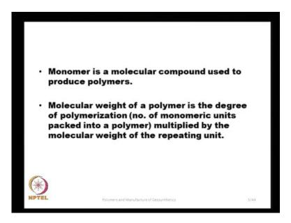
The monomer is a molecular compound is actually, it is basically the basic unit to produce polymer and the molecular weight of a polymer is the degree of polymerization. Is actually, the degree of polymerization is the number of monomeric units packed into one unit of a polymer. And the molecular weight is the degree of polymerization multiplied by the molecular weight of each of these single repeating units.
