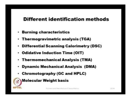
There are varieties of methods for identifying the type of polymer some of them are listed here by looking at the burning characteristics, thermogravimetric analysis differential scanning calorimetry oxidative induction time thermomechanical analysis, dynamic mechanical analysis, chromotography and molecular weight basis.
