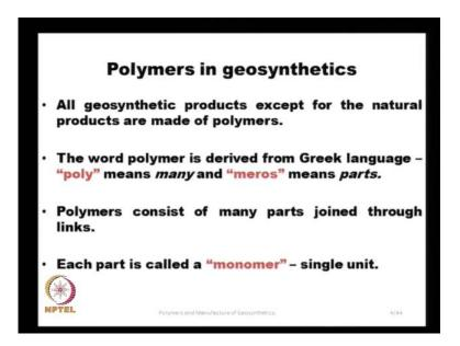
Well all the geosynthetics except for the natural products are made of polymers as we have seen the natural products are the coir and the jute and apart from these 2 varieties all others are made of polymers. And the word polymer itself is derived from Greek
