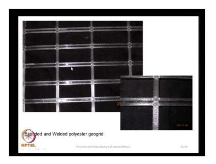
And some examples of the welded polyester geogrid is shown here, we take strips of this polyester strips and actually, these polyester strips, they are extruded. So, that they have good strength stiffness and long term stability and they are welded together at these junctions to fabricate this type of geogrid.
