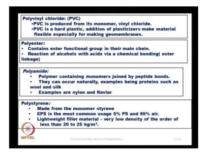
Poly let us look at the different types of these polymers, the polyvinyl chloride the P V C is produced from it is monomer, vinyl chloride. And P V C is actually, it is a hard plastic addition of plasticizes makes the material flexible, especially for making geomembranes the P V C, we see them in the form of electrical conjudes so on, we use them for domestic purposes.
