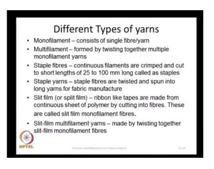
Well the different types of yarns, yarn is basically the long fiber that is used for manufacture of textiles monofilaments consists of single fiber or single yarn and multifilament, it is formed by twisting together multiple monofilaments yarns. And the other form of this the fibers is a stable fiber, it is we take a continues filament and we crimp it and cut it to short lengths 25 to 100 millimeters long.
