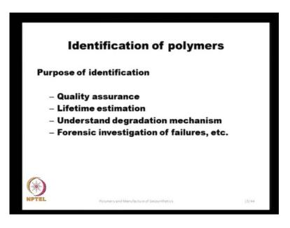
Well how do we identify a given polymer the purpose of identification is several fold, one is the quality assurance and then the lifetime estimation, because different polymers, they have different lifetimes. And we also need to understand their degradation mechanism once there installed in the in the soil and for investigating any failures the cause for any failure and so on. So, we need to identify, the type of polymer for all these purposes.
