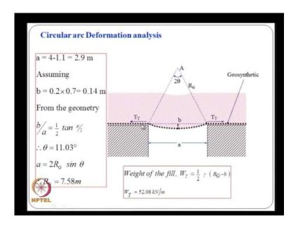
And from the geometry of this deformation, we can calculate the strain in the reinforcement.
