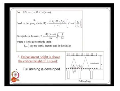
And for shallow height embankments the pressure that is transferred to the geosynthetic is written like this, s times some factor partial factor times gamma H plus some partial factor times surcharge gamma H is the self weight load and the W z is the is the surcharge load. And these are the 2 partial factors this divided by s square minus a square multiplied by s square minus a square p c by sigma v, where sigma v is the vertical stress that is nothing but gamma H plus W.
