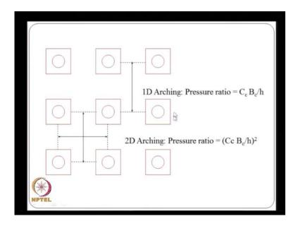
And we can use one dimensional arching theory or 2 dimensional arching theory, the if you use 1 D arching theory, the pressure concentration ratio C c B c by h whereas, in the 2 d arching, this gets squared C c B by h square.
