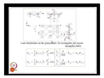
And these are some of the mechanisms, that were outlined by Kempfert, where we can calculate the force, that is transferred into the piles through these equations.
