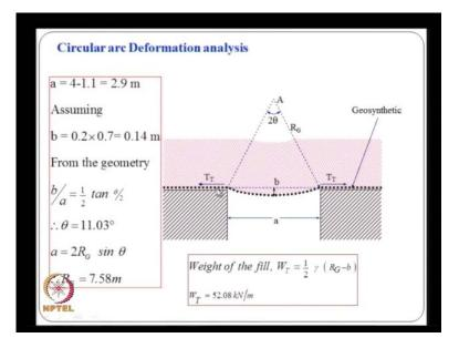
And lets say that, because of the placement of the geosynthetic pile system our settlements are only 20 percent of the settlements of the untreated ground is about the maximum settlement is about 140 millimeters. And if you assume that, between the 2 supports the geosynthetic undergoes a circular arcs type deformation, we can just construct this geometry.
