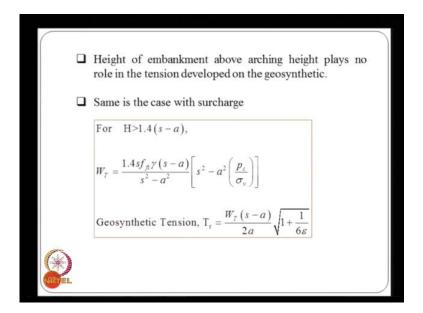
And if the full arching is developed, it is assume the height of the embankment above the critical height does not increase the geosynthetic tensions all that additional load is directly transferred into the piles, our load on the geosynthetic is a given by this. And the geosynthetic tension is given like this.
