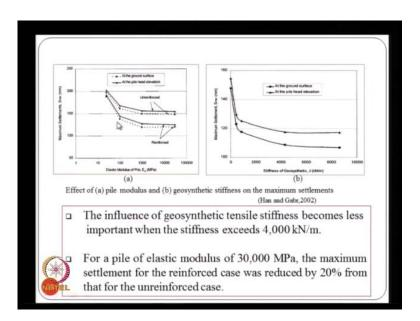
And some of their findings are like this and they have shown the relation between the elastic module of pile and then the maximum settlement, the foor unreinforced case and for the reinforced case and with reinforced settlements are found to be lower. And the settlements shown with the dashed line, these are at the ground surface, that is at the top of the embankment whereas, the solid lines, they show the settlements at the pile head or the foundation soil level.
