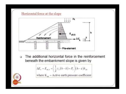
And once again, even the german code, they also recommend that additional force, that is generated in the reinforcement, because of this lateral thrust is considered.
