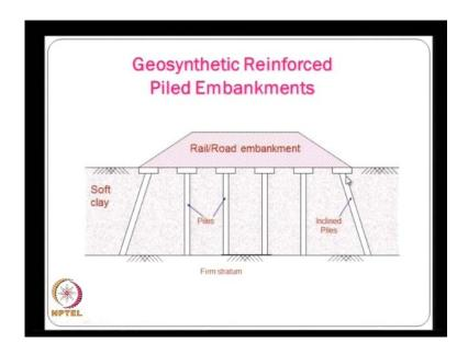
Especially, the pile raking is something at the end of the embankments, we give the inclined piles to take care of the lateral thrust from the high embankments. And because the provision of horizontal of layers of reinforcement all the lateral load is taken by the reinforcement, and because of that the lateral loads transferred into the piles or much smaller or very low and so we can just think of providing vertical piles.
