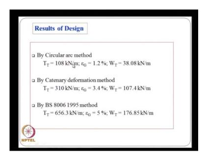
And the comparison in the results between the different methods, where is circular arc method, the tensile force in the reinforcement is 108 kilo Newton per meter whereas, the catenary deformation method. It shows 310 whereas, the B S code, it shows much higher force of 656, which is very high and the level of the stress mobilized are also very different 1.2 percent by the circular arc theory whereas, the other one is almost 5 percent strain.
