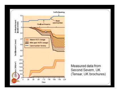
And the performance and the monitored performance is excellent as shown here and the bottom part, we see the stress and the top part, we have the settlement is actually the with time. The construction of embankment took place for constructing about 10 meters high embankment, it took almost 220 days is about 7 and half months, which is relatively past. And these are the settlements is actually above the V C C this red lines, they show
