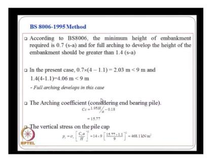
And the same design by using B S code is it is like this, we can and our embankment is 9 meters size, which is more than the critical height, we can estimate that, the arching is fully developed, the arching coefficient for embearing piles is 15.77 by substituting all the values here, then the vertical piles of the pile cap is this.
