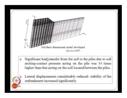
By considering the solid elements and they found, that the significant load transfer happens from the soil to the piles, because in soil arching. And their contact pressures predicted from full 3 dimensional analysis are about 40 times higher than the tacting on the soil located between the piles.
