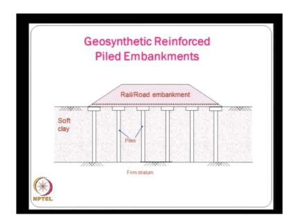
Basically, because these piles, they extend into the firm stratum and because of that the expected settlements both total and differential or very small with this type of constructions.
