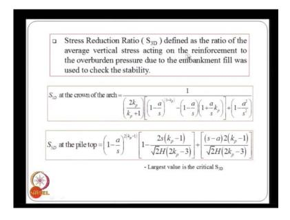
And the stress reduction ratio is defined as the ratio of the average vertical stress acting on the reinforcement to the overburden pressure. And they have developed some equations for the stress that at the crown of the arch and then the pressure, that is transferred into the piles and this is our including the stress intensity factor.
