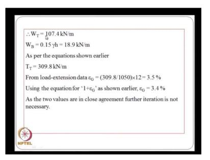
And the weight acting on the reinforcement is 107 kilo Newtons per meter and the tensile force, we can calculate as 309 kilo Newtons per meter using the previous equations. And the from the load extension data, this load of 309 kilo newton per meter corresponds to a strain of 3.5 percent and the geometry of data assumed deformation shows strain of 3.4 percent. So, which are in a very close to each other, so this design is valid.
