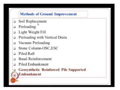
And we have already seen that, there are several options, that are available for construction on a soft clays, that is the easiest one is the soil replacement, if the thickness of the clay soil is very small. We can think of replacing or the preloading that we have
