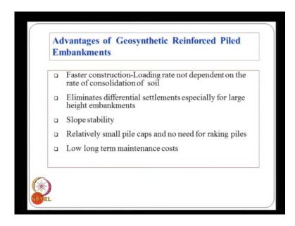
And is also, we will have very low maintenance costs, because the differential settlements on the total settlements, that are expected from the systems are small.
