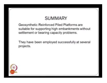
So, just to summarize the geosynthetic pile embankments are successfully applied for all for all the constructions of very high embankments, some resting on soft clay foundation.
