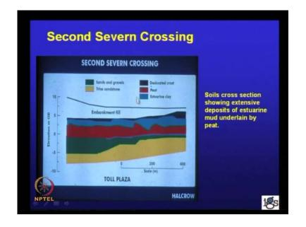
And the second severn crossing, it is once again through a very highly marshy area and we can see the soil deposit is actually it is a thick layer of P T soil peat and then estuarine clay with both of them are very very soft. And so the any construction of this is the embankment construction and if it passes through that type of a soil, we should expect very large settlements and then the problems, because of lateral flows.
