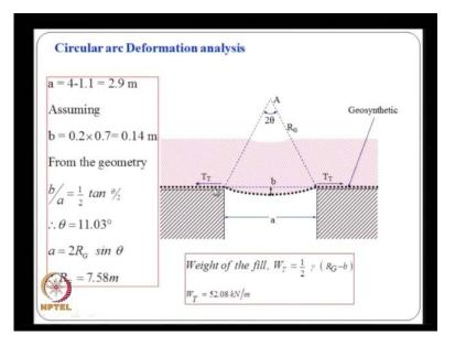
And is actually, we can assume different geometries for this deformed shape and we have assumed that.
