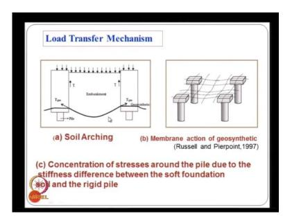
And the load transfer mechanism is very simple, in the absence of any reinforcement all the load is transferred directly into the foundation soil, but because of some friction that is there, because of our inclusions the form of piles and other things. The soil arching may take place that is the concentration of soil pressure the surcharge pressure at some locations where, there is no vertical moment and lesser deformation and lesser pressures are some other places.
