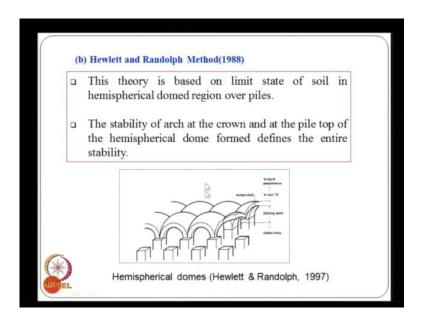
The same arching theory was modified by hewlett and randolph and they considered a spherical type of arched surface, where as terazaghi is considered planar surfaces, they have considered spherical surface. And the they have come out with some other theory to estimate the limit state of soil and then the pressures. And this is how there assumed surface is the deformed as soil surface
