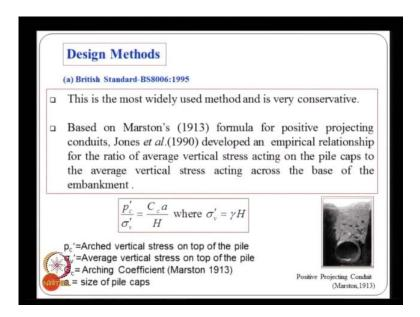
And all the design methods, they relay on the soil arching principles and the one of the most popular design codes is the B S 8006, that is the british standard code, that we have seen earlier and this is the most widely used. And it is also found to be the most conservative among all the different design theories. Jones in 1990, he used the methodology proposed by Marston for the case of positive projecting conduits for
