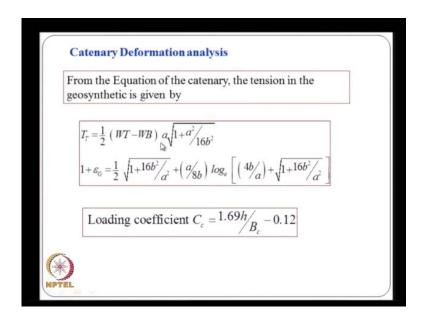
And we can also assume different shapes the catenary type of deformation and we can calculate under this is the archong coefficient.
