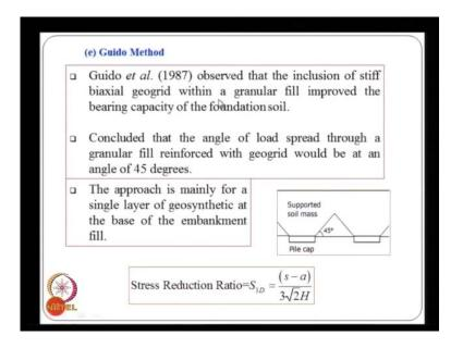
And guido et al in 1987, they also proposed some theory, wherein they assumed that instead of domed surface, we can assume this arched portion as a triangular portion, which is at 45 degrees, they observed that the inclusion of stiff biaxial geogrid improve the bearing capacity of the foundation soil. And the we can assume that, the load is filled through the granular fill at an angle of 45 degrees, that is a simplified form of the assumptions.
