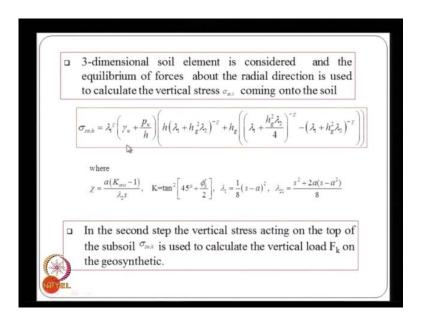
And these are the pressures, that are calculated based on this based on this approach, basically the pressure that is transferred on to the geosynthetic and the soil their functions of the unit weight. And then the applied loading and all other factors like the factors related to the spacing between the piles and so on.
