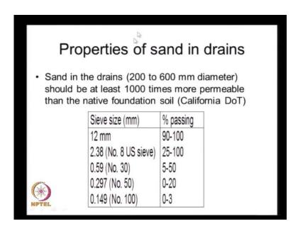
These sand drains or sand columns are typically 200 to 600 millimeters in diameter and the empirical experience shown that the sand in the sand drains should be at least 1,000 times more permeable than the native foundation soil. To achieve a very high permeability, we require the sand that is placed in the sand drains to meet a certain gradation requirements. One of the earliest to recommend this type of recommendations
