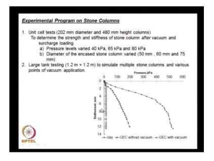
Here, we see the application of vacuum, the result of that vacuum and stone column if we draw the pressure settlement graph, this is the response of the soft clay soil and this is the response of the stone column, which is not treated with a vacuum. The same stone column after the vacuum treatment behaves very stiff and also much stronger, that is the main advantage of the vacuum treatment because it can increase the strength.
