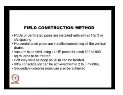
Both of them can be illustrated, I will show you the pictures later, some of the pre consolidation by vacuum or like this the PVD's or the perforated pipes installed vertically at 1 to 3 meters centre to centre spacing. Initially, when the technique came in, the companies have used perforated vertical pipes to suck the water or to apply the vacuum distribute the vacuum into the soil. Later on, once the PVD's coming to the market PVD's are used to distribute the vacuum.
