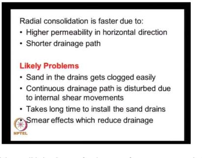
Then, our radial consolidation is very fast because of two reasons; one is because of higher permeability in the horizontal direction. We all know that most of the clay soils there highly an isotropic and they have different properties and different directions and because their direction of deposition is in the vertical direction, they have an easy flow path in the horizontal direction as compared to vertical direction.
