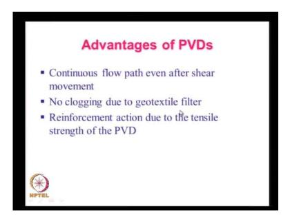
Some of the advantages that are claimed for a pre fabricated vertical drains are like this. The continuous flow path is ensured even after shear deformations because these PVD's are highly flexible. They can be bent or they can be twisted without rupturing because both the core and the cover that is filter are highly flexible and they can be strained up about 20 percent without rupturing.
