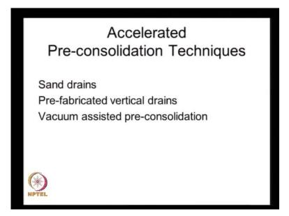
I have improved these techniques a lot and some of the techniques that we can use, for accelerating the pre consolidation of the clay soils or the sand drains. Historically, the sand drains have been used for a very long term, right from 1920 up to probably mid 1970s. After that we have the pre fabricated vertical drains made of geosynthetics and then more recently the vacuum assisted pre consolidation.
