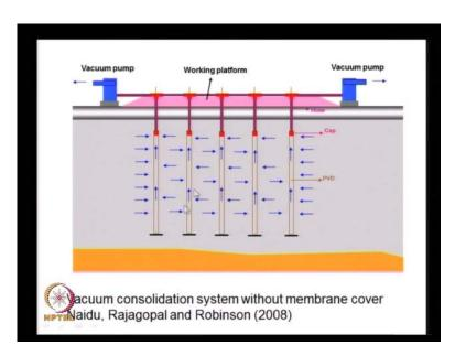
The system without any membrane is shown here, if we have a natural thin clay crust, we can take advantage of it, otherwise we can we can place a place a mat of clay soil to isolate the area of treatment from the rest of the soil medium. Once again, we connect these vertical PVD's into the drain pipes or the horizontal pipes, through which the vacuum is applied.
