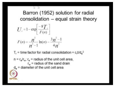
The radial consolidation theory has been solved by several researchers, Barron in 1952, he has proposed the solutions for two types of field analysis, one is the freed free strain case, where in we apply flexible loading and the settlement is non uniform. The other theory is equal strength area, the rigid loading where in our settlements are equal all through and in variably the equal strain theory is more applicable because our foundation structures.
