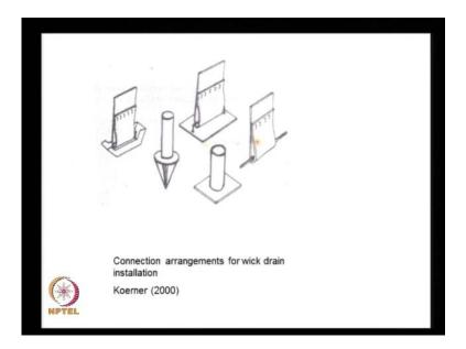
These are the different types of connector plates for connecting the PVD and these connector plates are the ones that are rigid. They can be pushed because the PVD's themselves are highly flexible and they cannot be directly pushed in to the soil. This particular picture is taken from Koerner text books on geosynthetics.
