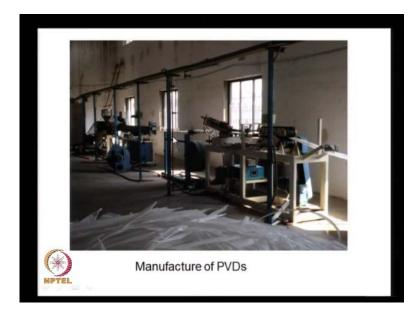
Here, we see a picture of the PVD being manufactured; these are all the plastic cores that are put inside the PVD. They are all joined together by welding process, by heat bonding and then these plastic cores are covered with a geotextile, in this particular case it is a oven geotextile.
