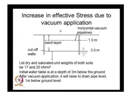
Now, let us let me illustrate how the removal of the atmospheric pressure from the soil increases the effective stresses. Let us take a case where we have the top 3 meters is a sand layer and then below this we have a clay layer. Let us say that initially the water table is at the depth of 3 meters and we have installed our vacuum pipelines at a depth of 1 meter below the ground level.
