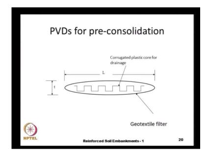
And here is a schematic of the pre-fabricated vertical drain it consists of a inner core, and then an outer textile that acts like a filter.
