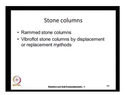
Some of these ground improvement methods are very briefly stone column is one method; there are different types the rammed stone columns, and the vibroflot stone columns, that can be formed either by soil displacement or by soil replacement this also we will see a bit later on in some other lecture.
