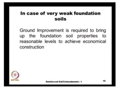
Well, in the case of very weak foundation soils we go for an ground improvement. So, that we can improve this soil properties to some reasonable level where in we can have economical solutions otherwise the treatment could be. So, expensive the construction could be, so expensive. So, the requirement of very large amount of reinforcement the plane the in the form of geogrids or the geocells, and so on.
