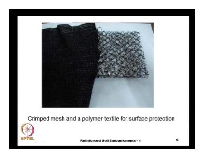
And here is an example of of a a crimped mesh, and a polymeric textile that can be used to to protect the surface of this slopes.
