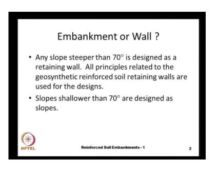
And what are the design approaches and especially when it comes to definition what is an embankment, and what is a wall slopes that are steeper than seventy degrees designed as a retaining walls. And the slopes that are shallower than seventy degrees are designed as slopes, and the we will see some of the principles applicable for these for the design of slopes in in the lectures to follow.
