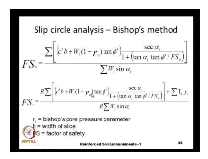
And more accurate way of a doing the design calculations is through the bishop's equation the bishop's equation is given like this, which is a very similar to earlier one except that we have the factor of safety. And both left hand side, and the right hand side is actually it is an implacity equation we we need to do some trial and error like we first assume some factor of safety based on the felonious analysis. And then substitute that
