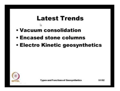
So, some of the latest trends that, we have in the geosynthetics, they are the applications of the geosynthetics for vacuum consolidation of soft clays and then of course, encased stone columns and the electro kinetic geosynthetics in here, we employ some copper wires along with a geotextiles or geogrids. So, that we can change the fundamental properties of the soft clays by polarizing the soil, because these techniques, we will see in some future lectures.
