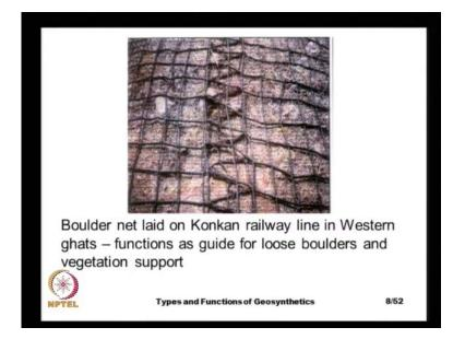
Here is a good application of a geonet is actually, this geonet is made of polymeric rope and this is called as a boulder net and this is used in the konkan railway in the western ghats. And the main function of this geonet is to act as a boulder and as a guide for the loose boulders.
