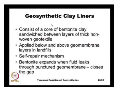
Another product geosynthetic product that, we have is geosynthetic clay liner is actually, this geosynthetic clay liner is an additional protection member that, we can that, we have
