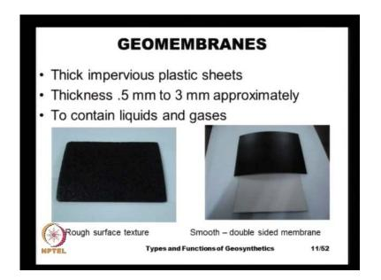
The other geosynthetic product is geomembrane, which is very commonly used for construction of landfills or for lining the canals or for lining some other water retaining structures. And these geomembranes, these are nothing but thick impervious plastic sheets and typically, their thickness can vary anywhere from 0.5 millimeters to almost 3 millimeters.
