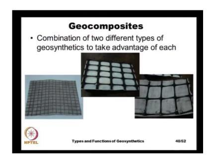
And another type of geosynthetics, they are geocomposites, we have several varieties of geocomposites. In fact, the prefabricated vertical grain is an example of a geocomposite
