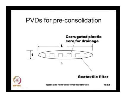
And in cross section a pre-fabricated vertical drain consist of an outer core of a geotextile that acts as a filter and there is an inner core that acts like the drainage medium. And this inner core could be made of in the simple P V D's, it could be just corrugated plastic sheet, plastic core or in more complicated systems, we could have a geonet in as a core and at the outside, we could have a thick geotextile, that acts as a filter.
