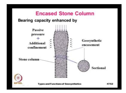
And one recent application of geosynthetics is in the form of encased stone columns. The stone columns are traditionally employed by geotechnical engineers for supporting of flexible structures like oil storage tanks or road way embankments and so on. And these stone columns, if they are constructed in a extremely soft clays, the main problem is it is difficult to form the stone column.
