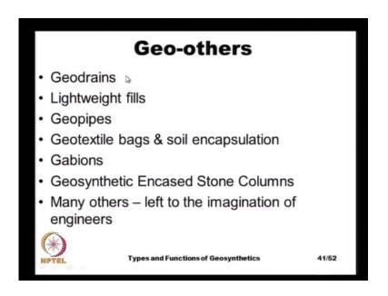
And there are several other geocomposites or water known as geo others, geodrains geodrain is nothing but a plastic pipe with perforations, once they are buried in the soil they can act as drains. Because, through the through this perforations in the pipe the rain water or the water in the soil can be collected and then it can be, it can flow through the
