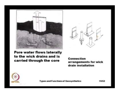
The concept is like this see, we introduce the pre-fabricated vertical drain into the ground by pushing, it by attaching it to some anchor like this and then we just simply push it and then allow the water to come out. And here, we see a schematically station of the water flowing through the geotextile filter and once it enters the core, because the core is highly permeable, the water comes out very fast.
