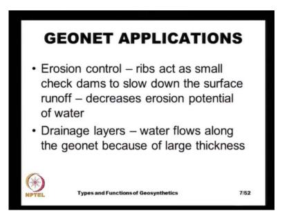
These geonet applications, they are mainly used for erosion control, because these ribs, because they are very thick, they act as small check dams to slow down the surface runoff. And once the rain water surface runoff is slow down, it reduces the erosion
