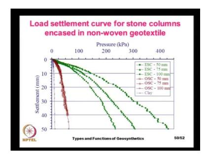
And here we see some test data from laboratory tests on encased stone columns, the pressures settlement data of the soft clay is like this.
