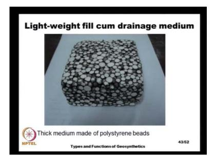
And we have number of light weight fills and these light weight fills, if they are made of small beads of polystyrene, they can also be made to act as good drainage medium and here, we see an example of a lightweight fill made by polystyrene beads. And the typical unit weight of these light weight materials is of order of the 0.3 to 0.4 kilo newtons per cubic meter comparatively, the weight of a soil typical soil could be anywhere from 18 to 20 kilo newtons per cubic meter.
