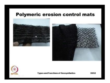
A some of the erosion control products are shown here is actually these are the trimped mesh the to once it is spread on the ground, it slows down the flow of water. And it prevents the erosion of soil, because it once it confines to the soil some extent, then it slows down the speed of the rain water on a slope. And once the rain water at the surface runoff is slowed down, it is erosion potential is reduced and then the soil is more stable.
