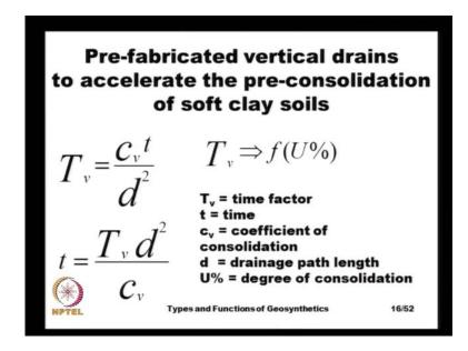
And another major application of the of the geosynthetic season, the form of a prefabricated vertical drain, that is used for accelerating the consolidation of a soft soils. Is actually, on the left hand side, I have given the equation for the time factor is a function of the coefficient of consolidation and the drainage path length d.
