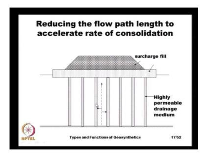
And here is a typical manner in, which we can apply the these drains and let us say that, we have a thick clay soil and if we do not put in anything the water has to travel this much length to escape from this soil. And it takes a very long time to consolidate the soil. And the other hand, if you introduce some highly permeable a members either sand columns or the pre-fabricated vertical drains and the length of the drainage path.
