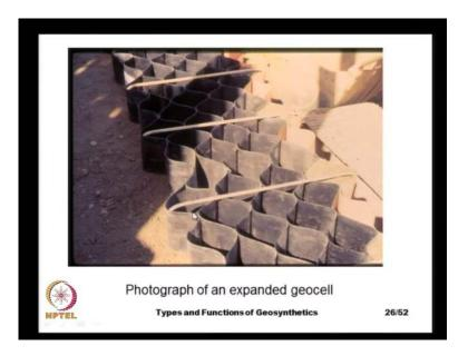
The expanded geocell is a something like this when the geocells first came into the market. This the geocells are made of plane plastic sheets like very similar to your geomembrane without any openings or without any rough surface. And now the more recent geocells, they are made with a either corrugated surface.
