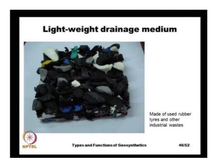
And there are other products, that have made of used rubber tires and other industrial waste products, which are all cut to pieces and bounded together. So, that we provide some thick mass, some thick medium, that is highly porous and slightly compressible. So, that it can act as a cushion and also it acts, it can act as a drainage medium and behind retaining walls, if these are applied, they can be made to act as a as drainage
