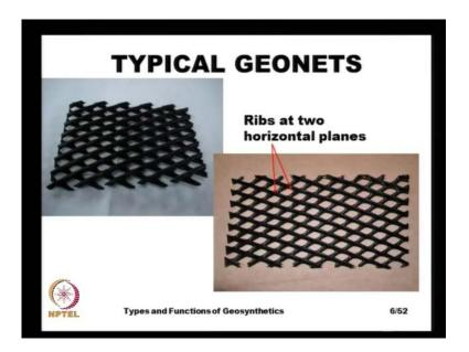
And these slide it shows typical geonets and we see that, the ribs or in 2 different planes and then the thickness of each of these ribs is very large, compared to that of a geogrid. And here, you see the close-up of the same thing, the ribs in 2 different directions and the aperture openings, they are more of diamond shaped and not square or rectangular.
