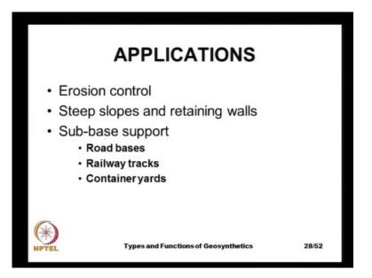
And some of the typical applications the apart from the load carrying functions, it can also be used as a erosion control product or for construction of steep slopes and retaining walls. And as a sub-base support it is an very excellent product, it can be used in road bases or it can be used in the railway tracks or it can be used for construction of the container yards and so on.
