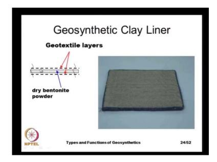
And Schematically G C L is something like this, we have a core of dry bentonite powder that is sandwiched between 2 thick geotextile layers. And the right hand side, we see a product of the G C L is actually, it is the same thing shown on the left hand side, we have a thick geotextile layer and the inside, we have the bentonite powder.
