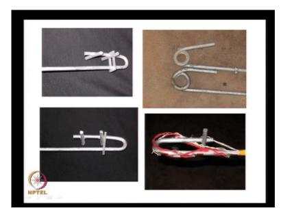
And when, we have steel measures, we can have different type of connection to the panels and through the hooks, and through the loops and we need to do the test, to make sure that, these connections they develop adequate pullout capacity. Then we also have to make sure that, the steel that is used is strong enough, sometimes if the steel mesh is made up on brittle steel, it will just simply break.
