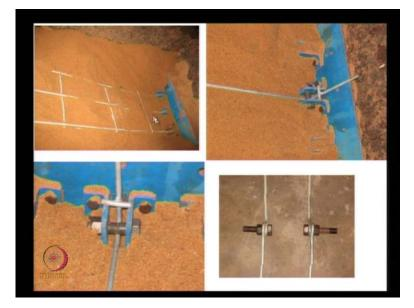
And here, we see number of test configuration. So, this the steel ladder and is connected the backend to stimulate the connection to the facing and here, we have this steel rod and that is connected by means of a crossbar, like this and in some cases we can have bolted connection or we can have a steel rod running across.
