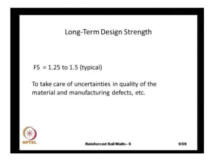
And the from this index strength we can extrapolate the long term design strength, by applying different factors of safety. This FS is the last factor of safety that we have, is typically 1.25 to 1.5 and this is mainly to take care of any uncertainty in the quality control of the material. And then there could be some manufacturing defects, over and above all the factors that we normally consider in our procedures.
