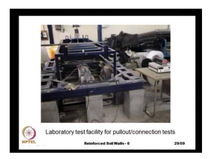
The apparatus at IIT madras is shown here, is actually this is a test tank, which is nearly 1 meter wide and 1.5 meters long and we have the actuated, the hydraulic actuator that runs on hydraulic pressure and the speed can be controlled anywhere from 1 millimeter per minute to 20 millimeters per minute and these are, all the instrumentation associated with it the load cell and then the LVDT the displacement indicator.
