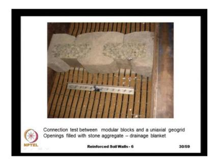
And here, we see a test as specimen being prepared, to determine the junction strength sorry the connection strength between a uniaxial geo grid and then the modular blocks and the in filled material that we use inside these, modular blocks during the test should correspond to the type of aggregate that is used in the site, in this particular case the stone aggregate is the drainage blanket.
