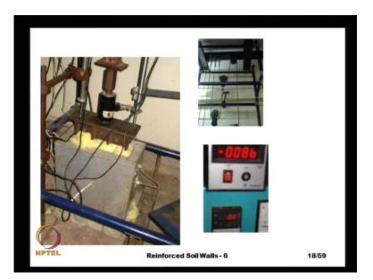
Wherein, we apply a constant tensile load, but then we subject the geo synthetic to some temperature increments, in steps of about 12 degrees to 12 to 15 degree centigrade depending on the type of polymer that we have. And here, we see an apparatus this is the
