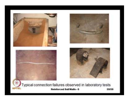
Is actually here we can see, this loop has just simply the toggle that was provided they just simply broke and in one case, the panel itself just simply broke open because it did not have adequate structural reinforcement and in some cases, if our cross rod is not of sufficient diameter it will just simply bend, like this or we have seen another examples of this bent bar.
