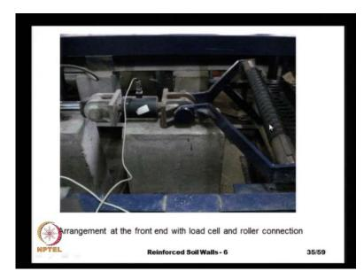
And this is the front connection, can see the roller that is used. So, that we have a good grip and this is the load cell, that we use for measuring the loads.
