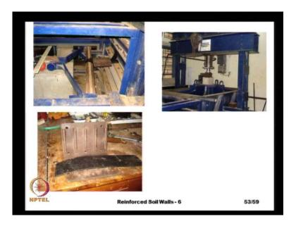
And we can do these pullout tests, on different type of reinforcements and one type of reinforcement that is commonly used is the polymer strip, which has a width of about 60 mm and it can be placed for any length because it comes in rolls and here we, see some pictures, is actually when we do some testing on this type of strips.
