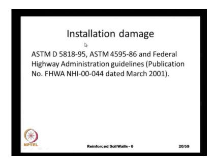
The other factor that we have is the installation damage, the ASTM D 5818 it describes the installation damage test and the federal highway administration guideline NHI 44 also talks about the installation damage test.
