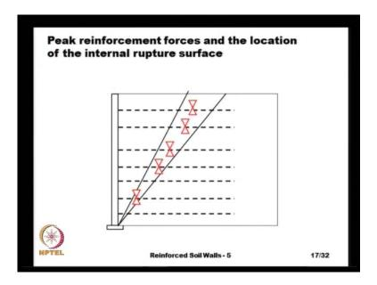
And for the purpose of calculations of the pullout capacity, we need to know where this the wedge stops. And we assume that, we have the Rankine active wedge by drawing a line at the bottom surface at an angle of pi by 4 plus phi by 2. And this particular result is also confirmed by so many other independent testing laboratories.
