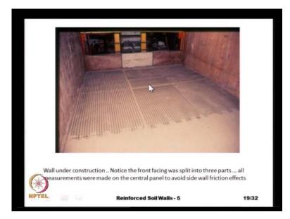
And here, in this slide, you see a large scale laboratory testing on the reinforced soil retaining walls wherein, the height of this wall is 3 meters whereas, the width is 2.4 meters. And the full scale test was done the reinforced soil retaining wall at the Royal Military College of Canada under the guidance of professor Richard Brethurst and this particular picture is from those tests.
