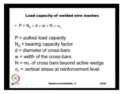
And the pullout load capacity of the welded wire meshes is estimated using this type of formulas, N q times d times w times N times sigma v where, N q is our bearing capacity factor, very similar to our bearing capacity equations. And the d is the diameter of the cross bars and w is the width of the cross bars, N is the number of cross bars with beyond the active wedge that is, within the stable soil zone and sigma v is the vertical stress that is acting at the reinforcement level.
