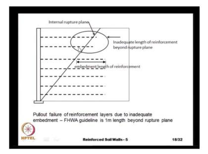
And the purpose for knowing this line is to be able to estimate the embedment length that is, the embedment length is the length of the reinforcement beyond our rupture surface. That is just a simple planar surface for the case of flexible reinforcements and for inextensible type reinforcements, we will see a bit later on. And our federal highway guideline is that, we should have a minimum embedment length of 1 meter beyond our rupture surface.
