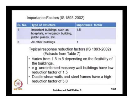
The importance factor is once again given in this IS code and this is given with respect to the structural applications. For example, depending on the type of the structure, whether it is an important building or any public place like hospital building or emergency buildings or a school building like that. And these structures, they will have an importance factor 1.5 and all other buildings will have an importance factor of 1 and we can probably extrapolate this at the soil structures.
