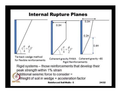
And all these results, they were compiled and put in the recommendation in different codal provisions. There are two methods of analysis, one is called as the tie back wedge method of analysis for flexible reinforcements wherein, our rupture surface is assumed to be a planar surface like this, our Rankine active surface. And so this is our active wedge
