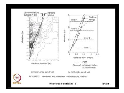
And that comparison is shown here, this straight line is the Rankine active wedge, that is drawn based on the friction angle of the soil and this is the observed failure surface from
