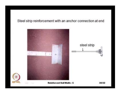
And a typical picture of a steel strip reinforcement with anchor is shown here, the reason why we use an anchor for steel strips is, as you know the steel has very high yield strength and compared to the pullout capacity is very low. To increase the pullout capacity, we can add an anchor element here, in this particular case, the anchor element is made up of a L angles, L sections and it is directly connected to the steel strip like this.
