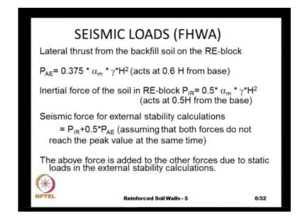
And this the acceleration coefficient, that we calculate can be used for estimating our additional loads on the reinforced soil structures. And once again, this procedure is given by a federal highway administration and there are two components to the seismic loads. One is because of the inertial forces, that are acting within the reinforced soil block and the other one is the lateral thrust, that is exerted by the back fill soil on the reinforced soil fill.
