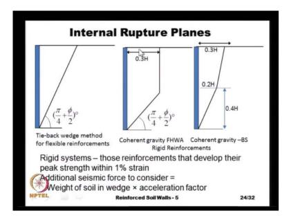
For example, for the tie back wedge method of analysis, this is the weight of the soil that we consider within this triangular wedge. And if there is any permanent surcharge that is acting on this wedge, we also take that as part of our inertial loads, and for the coherent gravity method, the weight of the soil within this bilinear wedge and then the surcharge that is acting on this some height of 0.3 H.
