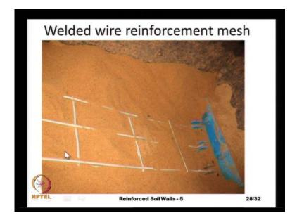
And the welded wire mesh, typical welded wire mesh is as shown here, we have length and then we have this cross members, against which some passive force can be developed. (Refer Slide Time: 41:31)
