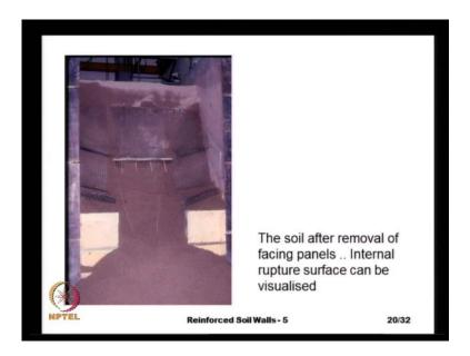
And here, we see the internal rupture surface so at the end of the test, if we remove the front panels and the soil just simply collapses the soil within the active wedge because it is already deformed sufficiently, that it just simply slides down. Whereas, the soil in the passive wedge or in the resistance zone is still standing and if we draw this line, we can complete that with the active wedge, that we get from the Rankine's theory.
