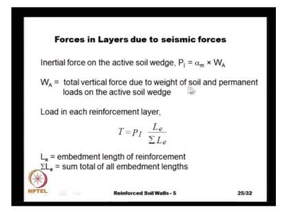
So, the forces that we consider in different layers due to the seismic inertial forces like this, the total inertial force that is acting on the soil wedge is P I that is, alpha m multiplied by W A. Where, W A is the total vertical force due to the weight of the soil within the failure wedge and then the permanent loads that are acting on the active soil wedge.
