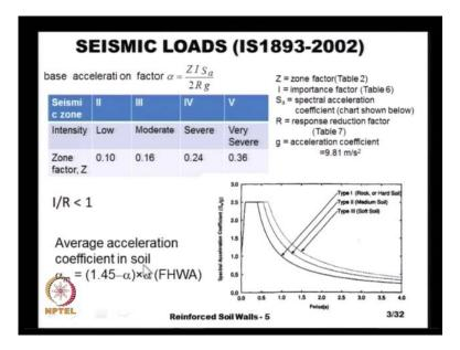
And once we can substitute all the different parameters in this equation and get our base acceleration factor. And then once we have this, we can calculate the average acceleration coefficient within the soil.
