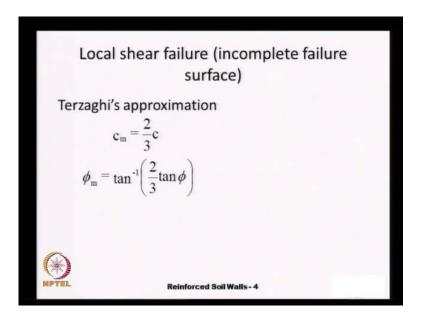
And when we have a local bearing failure, local shear failure of the above formulas that we have these are not valid manly, because those formulas are derived for a case where our rapture surface is completely developed.
