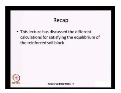
And just a recap we have discussed the different steps that are involved in calculating the length of the reinforced block to satisfy all the of the different external stability requirements, that is the sliding, overturning, bearing capacity failure, of the settlements and then the slip circle failure.
