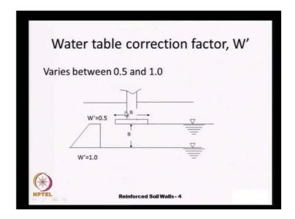
And the final correction that we apply is the w prime is actually, that is there only for the n gamma that is cause the gamma here is gamma bulk.
