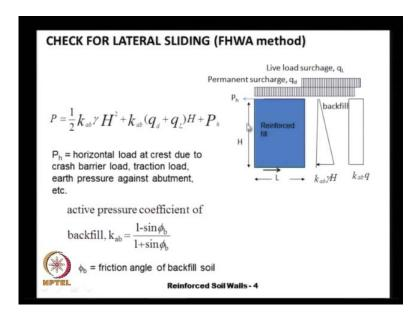
That is gamma h l is the gamma is the unit weight of the retained soil fill multiplied by height and l and all the calculations are done per unit length perpendicular to the plane of the analysis, just as how we did in the regular geotechnique engineering courses either the design of the retaining walls or the design of slopes and so on. (Refer Slide Time: 12:31)
