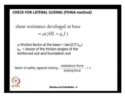
So, our gamma h l is the weight of the soil within the reinforced block plus the q d that is the permanent surcharge multiplied by the length l multiplied by one unit length in the perpendicular direction will give us the magnitude of the preeminent load. That multiplied by mu is the frication factor that is acting at the base, and in case of any lack of data of the foundation soil.
