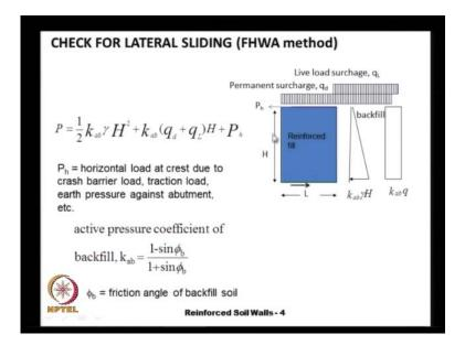
So, now let us see how we can check for the lateral stability of the wall, and the federal highway administration method is the simpler one, where as the BS code method the British code 8006 is a bit more complicated, but ultimately both of them are equivalent. Let us consider a reinforced soil wall like this, having a block length of 1 and height of h and for simplicity lets you consider only horizontal back fill, because the principles are the same.
