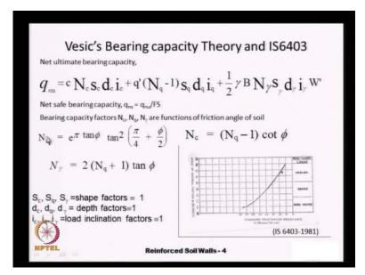
And once you have the c and m phi m we can go back and substitute the phi m in place of phi to calculate our bearing capacity factors N q, N c and N gamma and c m in place of c here.
