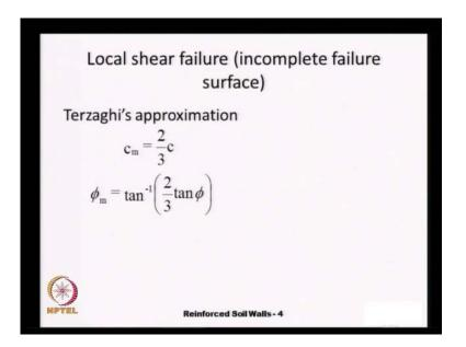
And Terzaghi being very highly practical person, he suggested that the shear strength properties can be slightly adjusted the account for local shear failure, and he suggested that the modified cohesive strength is two thirds of c, and the phi modified tan inverse of two third tan phi.
