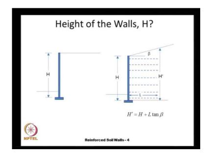
So, for the design purposes we need to calculate the height of the retaining wall, and the height of the retaining wall is defined like this, when you have a horizontal back fill. The height of the wall is always calculated as the height measured from the top of the leveling pad up to the top of the back fill soil, this is the height and we neglect the soil that is their in front of the wall, because that is liable to escalated for maintenance purpose and so on.
