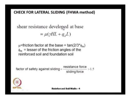
And shear resistance that is developed at the base is the mu that is the friction factor that is developed at the base of the retaining wall multiplied by gamma h l.
