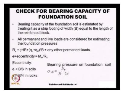
And this q n is noting, but this sigma v b that we calculate as the bearing pressure on the foundation soil.
