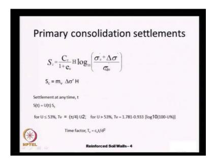
The primary consolidation settlements they are estimated either in terms of the compression index C c are the coefficient of volume compressibility m v depending on the data that we have. If we are within the normally consolidated rains we apply the first formula C c and if we are in the over consolidated rains we apply the m v, and the different factors here.
