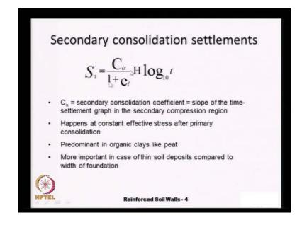
The other type of settlement that we have is the secondary consolidation settlements, that is the S is c alpha by 1 plus c f h times log t the secondary consolidation settlements are time dependent, they are not dependent on the pressure. Whereas, the primary consolidation settlements they depend on the pressure increments, see here we have the pressures whereas, here we do not have the pressure, but we have only the time.
