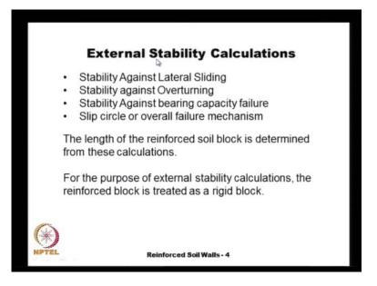
Just give a brief outline as we discussed in the previous lecture, there are a different calculations we need to do to satisfy the external stability conditions. The first one is the stability against lateral sliding, because our retain wall is retaining the soil at an angle stepper than it is shown the angular free pose there is tremendous lateral pressure that is acting on the wall.
