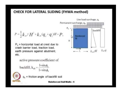
The overturning moment is once again, because of the triangular distribution and the rectangular distribution and we realize that the center of gravity of the triangular is that one third of the height whereas, the rectangle is one half of the height.
