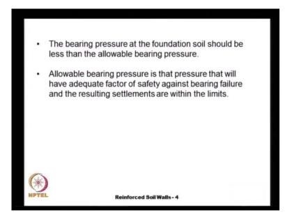
And the allowable bearing pressure itself is defined as that pressure, that we can apply that will not cause any foundation failure due to the bearing capacity exceed, the bearing pressure exceeding the bearing capacity by certain factor are the settlements exceeding our permissible limits, so that is called as the allowable bearing pressure.
