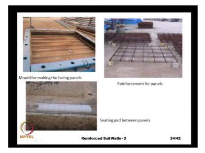
And these are the details of the facing panels made, this is the mould and the top left side is the mould for making the panels, and we can give different finishes, and this particular company uses very simple pattern the longitudinal strips. And here we see this um the strips in the mould, and we have to give some small reinforcement in these panels, because they are very heavy and they are handled by means of some cranes.
