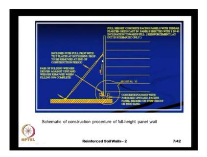
And here we see the a cross section of the full height panel wall a schematic sketch, it needs to be supported by means of some external props, and during the construction what we do is here at the bottom we have the leveling pad, we place it carefully. And we give some inward batter all these walls they are given some inward battle, that is their incline into the soil, the reason is as they are inclined into the soil and when the during the construction the soil is placed in layers.
