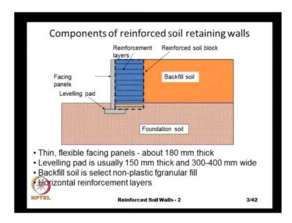
Just recap reinforce or retaining all consists of facing panel and then number of horizontal reinforcement layers that could be their geosynthetic that is polymeric or metallic in the form of steel. And then we have good granular re back fill that we have within the reinforce block then the back fill and the foundation then of course, leveling pad to maintain our levels.
