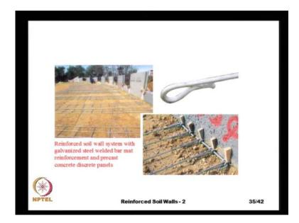
Here we can see this, the black color seating pads and here we see a picture of the reinforcement that is made of steel wires welded wire meshes, here these are the longitudinal elements and these are the cross bars. And these cross bars they can be at different distances and once again the distance that we that we give that depends on the amount of tensile force, that particular layer of reinforcement has to carry.
