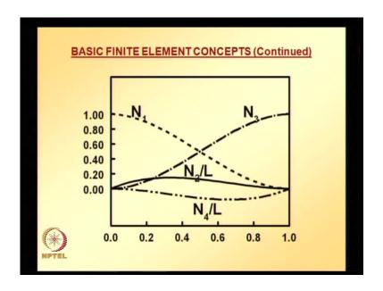
This plot shows how shape functions vary with respect to s; that is, s going from 0 to 1. You can easily observe that N 1 is equal to 1 at s is equal to 0; N 3 is equal to 1 at s is equal to 1; N 2, N 4 are normalized with respect to L. We learnt that the trail solution v, now, can be written as N 1 v 1 plus N 2 theta 1 plus N 3 v 2 plus N 4 theta 2.
