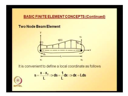
A simplest element, which is a two node beam element has 2 degrees of freedom per node. A two node straight beam element is shown here in this figure. Here EI is assumed to be constant over the entire length of the beam element and also, applied load along the element length is uniformly distributed. So, q is uniformly distributed and EI is assumed to be constant. We will be using these conditions at the end, when we are trying to simplify the stiffness equation and also load vector.
