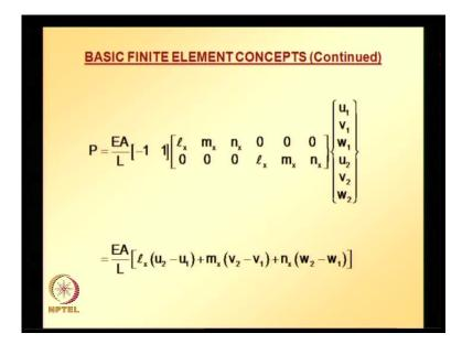
So, once we get the global displacements, we can calculate local displacements; once we get local displacements, we can calculate strains and then stresses and using those values, we can calculate the forces in a truss element 3-D truss element. The equation is given here and this equation in terms of direction cosines after manipulating the first equation is shown there.
