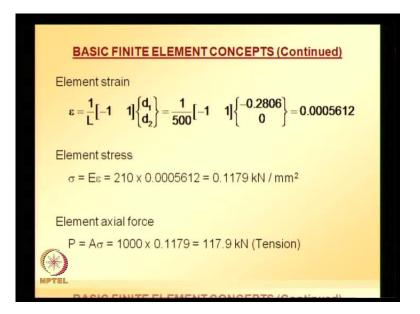
So, using these values and also for element 1, we know, what is cos alpha sine alpha? So, we can find what the local displacements and using the local displacements, we can calculate the element strains and element stress and axial force and axial force turns out to be positive.
