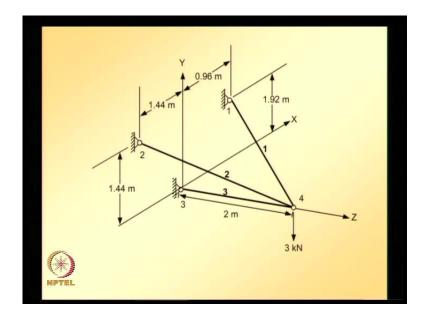
And now again here for simplicity, the element equations are directly written in terms of global degrees of freedom while, taking into consideration, the boundary conditions the unknown reactions at ith node corresponding to 0 displacements are identified as R xi, R yi, R zi i takes values 1 2 3.
