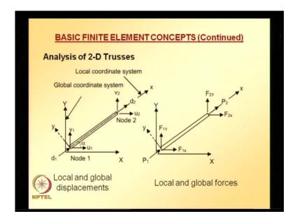
Analysis of 2-D and 3-D trusses, we will be looking in this lecture. And before we look at the derivation details, let us see what truss members are? Trusses are structural frame works, in which individual members are designed to resist axial forces only. They are commonly found in roof structures and bridges. The equations for these elements are well known in a structural engineering field and usually, are covered in traditional courses on matrix structural analysis.
