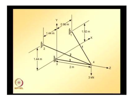
So, we can directly write the global equations corresponding, these degrees of freedom. So, this is what I just mentioned nodes 1, 2, 3 are fixed so, the corresponding degrees of
