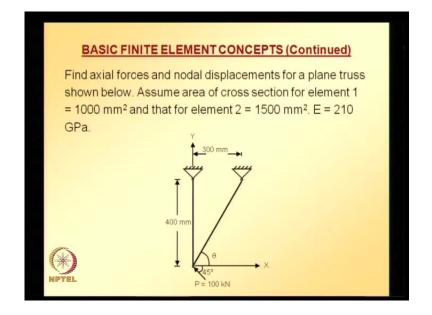
So, now we can solve an example. We can solve an example to understand the concepts, which we learnt now. Find axial forces and nodal displacements for a plane truss, shown below. And assume cross section area of cross section of element 1 to be 1000 millimeter
