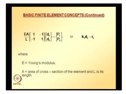
Similarly, the force the local coordinate system consists of 2 components: capital P 1, capital P 2. In the global coordinate system, the force vector consists of 4 components: F 1x, F 1y, F 2x, F 2y. And now, let us see the element equations for axial deformation element, which we already learnt in the last lecture, EA over L 1 minus 1 minus 1 1 and d 1 d 2 is a local displacement vector; capital P 1 capital P 2 is local force vector.
