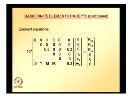
And now we are ready to assemble the global equation system, but since at each node, we have 3 degrees of freedom and there are 4 nodes. So, global equation system will be 3 times 4 that is, 12 by 12 and it is very cumbersome to write a big 12 by 12 equation system instead of that with a reasoning that since, node 1, 2, 3 are fixed and the corresponding degrees of freedom are 0 and we have seen from the 2-D truss problem.
