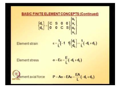
So, this is the relation between local displacement vector and global displacement vector. So, using the values of u 1 v 1 u 2 v 2, we can back calculate what is d 1 d 2 using this relation? Once, we get d 1 d 2; we can calculate element strain and once we get element strain, we can calculate element stress and we can calculate element axial force.
