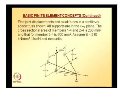
So, to understand these concepts, let us solve a 3-D truss problem. Find joint displacement and axial forces in a cantilever space truss shown. All supports are in x, y
