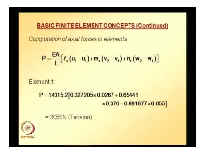
So, computation of axial forces can be calculated using this equation. For element 1: applying this equation and noting that for element 1, local node 1 is same as global node 1 and local node 2 is same as global node 4 and with that understanding, the axial force in element 1 is given by this and it turns out this element is in tension.
