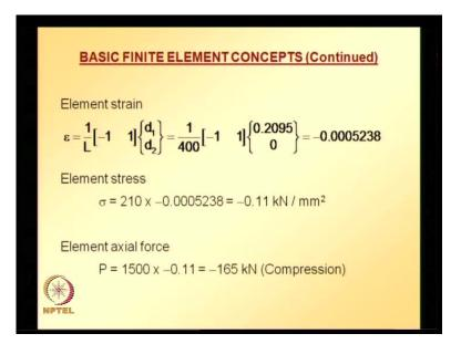
So, the local displacements can be obtained in this manner. Once we get local displacements, we can calculate strains, element strains, using this relation element stress and it turns out that element strain is negative quantity, that is, compressive and element stress also turns out to be negative and element axial force turns out to be negative. So, it is compressive force so, the member is in compression.
