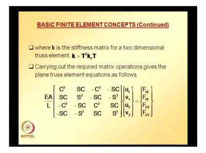
So, where k is the stiffness matrix for 2 dimensional truss element. So, carrying out the multiplication; carrying out the required matrix operations, we get for the plane truss element the equation system in this manner. So, once we know the ends, the spatial coordinates of ends of a plane truss element, we can easily assemble. When once we know the material properties and geometric properties, we can easily assemble the element equations for a truss element using this equation system.
