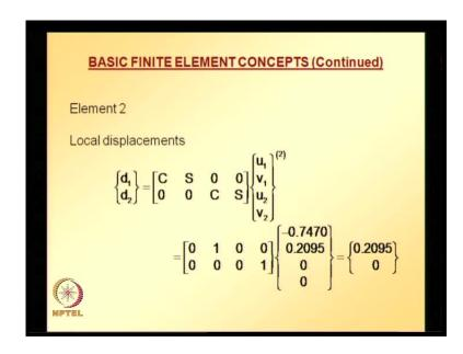
So, it is tensile force. Similarly, for element 2, local displacements can be obtained using global displacements u 1 v 1; u 1 v 1 just we calculated and the values that we calculated using though they are nothing, but u 1 v 1; u 2 v 2 global displacements u 2 v 2 for element 2 corresponds to u 3 v 3 which are 0.
