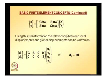
And please note, that local displacements gets transformed in the same manner as coordinates spatial coordinates. So, we know that the transformation between local X axis Y axis and global X axis Y axis. So, this d 1, which is a local displacement at node 1 in the X direction is related to the global displacements u 1, u 2 in the capital X capital Y direction in the same manner as, small x is related to capital X capital Y, that is d 1 is equal to cos alpha u 1 plus sine alpha v 1.
