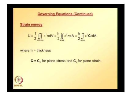
Now, let us look at how strain energy is defined. Strain energy is given by this; half integral over the entire volume of the structure or particular object, that we are looking at epsilon times epsilon transpose sigma. We need to integrate that over the entire volume and if the thickness is constant; if thickness of that particular component is constant, we can pull thickness how; h is thickness here; h is pulled out.
