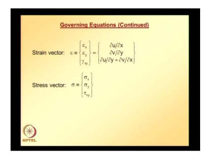
And this is stress and strain, sigma and epsilon involves three components. So, this is how, strain energy U is defined.
