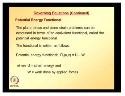
Potential energy functional: The plane stress, plane strain problems can be expressed in terms of equivalent functional called potential energy functional and the functional is written as follows. pi, this functional is going to be function of displacement in the x direction and displacement in the y direction. This functional is denoted with letter pi; potential energy functional is equal to U minus W, where U is nothing but strain energy and W is work done by the applied forces.
