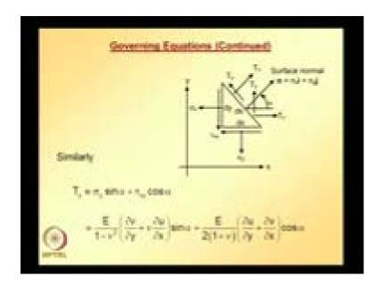
Similarly, starting with the second equilibrium equation or writing equilibrium equation for this differential element in the y direction and again expressing stresses in terms of strain and strain in terms of displacements, we get this equation.
