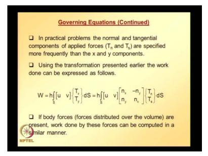
It is very simple. We know the relationship between T x, T y and T n, T s. So, we can use that and rewrite or re express this in terms of T n, T s using direction cosines of outer normal to the outer normal to the surface over which, tractions are specified. If body forces are present, work done by these forces can be computed in a similar manner. So, now this is how, the potential energy functional is defined; strain energy minus work done by forces applied forces.
