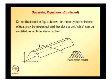
Let us look at a figure, this this plane strain conditions are illustrated in the figure below. The dam is shown here. For these systems end effects may be neglected and therefore, unit slice can be modeled as plane strain problem. Actually, this is a three-dimensional problem. But for computational simplification, we are taking it as a plane strain model; since one of the dimensions is much longer than the other dimensions.
