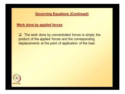
So, now let us look at work done by applied forces, W. If the forces that are applied are concentrated forces, work done by the concentrated forces is simply product of applied forces and corresponding displacements at the point of application of load.
