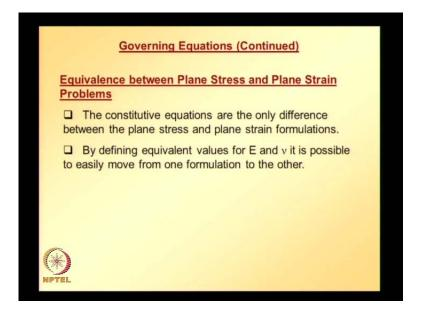
Equivalence between plane stress and plane strain problems. The constitutive equations are only difference between plane stress and plane strain formulations. By defining equivalent values of young's modulus and poison's ratio, it is possible to easily move from one formulation to other.
