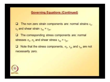
The nonzero strain components are normal strains and shear strains. The corresponding stress components are normal stresses and shear stress. Again out of plane strain
