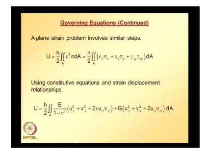
And now, let us say assume that the problem is plane strain problem. And this is how, strain energy is defined. Substituting epsilon and sigma, all the components and performing epsilon transpose sigma, we get this. Now, expressing using constitutive equations and strain displacement relations, we can express this equation in terms of displacements. Finally, strain energy in terms of displacements looks like this. And now,
