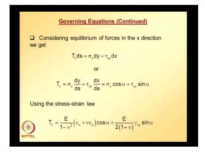
Considering equilibrium forces in x direction, we get this and dividing this equation on both sides with d s, we get this. So, this gives us relationship between traction component in the x direction and internal stress components sigma x, tau x y or tau y x. And now using stress strain law, we can express this in terms of strains and using strain displacement relation, we can express this in terms of displacements.
