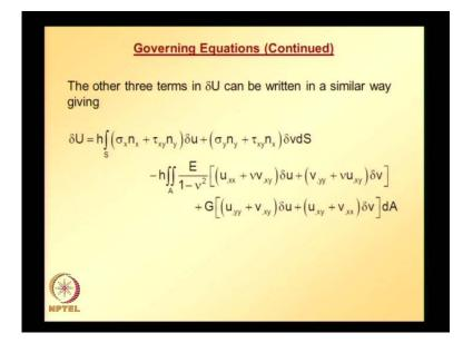
Other terms also can be written in a similar way and then finally, variation of strain energy is given by this one. Now, we need to find variation of work done by the applied forces. As I mentioned, forces can be different kind of forces, concentrated forces, distributed forces and body forces. But for generality, let us assume that the forces are distributed.
