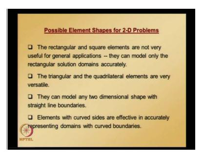
Possible element shapes for 2 - D problems the rectangular, and square elements are not very useful for general applications, they can model only rectangular solution domains accurately. The triangular and quadrilateral elements are very versatile, they can model any two dimensional shape with straight line boundaries. Elements with curved sides are effective in accurately representing domains with curved boundaries.
