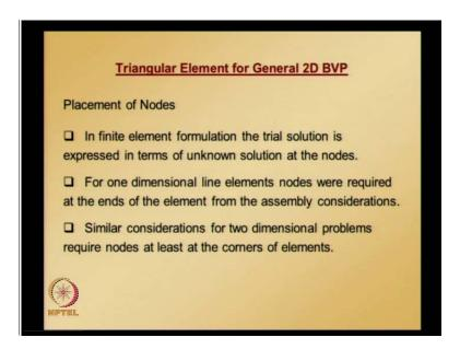
Triangular element for general two-dimensional boundary value problem, placement of nodes in finite element formulation the trial solution is expressed in terms of unknown solutions at the nodes, and this is what we also observed when we are looking at one dimensional problems.
