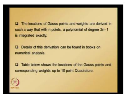
The locations of Gauss points and weights are derived in such a way that N points with N points a polynomial of degree 2 N minus 1 is integrated exactly. So, the locations values of Gauss points that is x i and w i a derived based on this condition that using N points we can or when we are deriving this. It automatically follows that if we adopt N points, we can integrate polynomial of degree 2 N minus 1 accurately.
