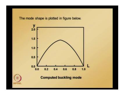
Once we have these two equations which represent how the mode shape is changing over element 1 and element 2, we can plot this and get the mode shape for the entire domain going from 0 to L.
