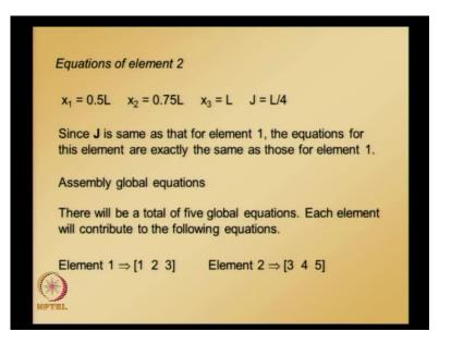
So, these are the element equations for element 1. We obtained K k and K p and now, element equations for element 2 are going to be similar. Since the nodal spacing is same and also material properties are constant for both elements, since J is same as that for element 1, equations for this element are exactly the same as those for element 1.
