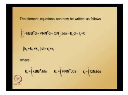
The equation can be written as: K k plus K p plus k alpha times d is equal to r q plus r beta, where each of the terms are defined like this. You can see here in K k you have B trans B B transpose and K p N N transpose is present.
