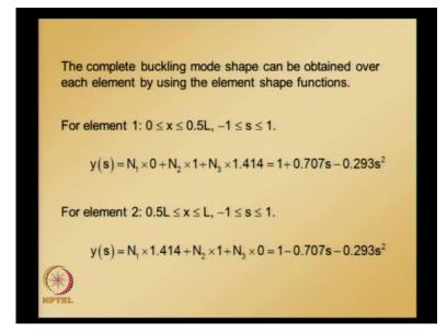
So, buckling mode shape is given by this nodal values and the complete buckling shape can be obtained over each element by using element shape functions. Once we got, once we get the nodal values that is y 1 y 2 y 3 y 4 y 5, we can do interpolation using finite element shape functions and get the complete buckling mode shape.
