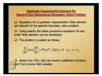
In today's class we will continue; so, what we will be doing in today's class is we will be deriving element equations using quadratic element for general one-dimensional boundary value problem which we already did earlier, using 2 node linear element. So, equations for a quadratic isoparametric finite element are derived for general boundary value problem using exactly the same procedure. Equations for any higher order finite element can be developed.
