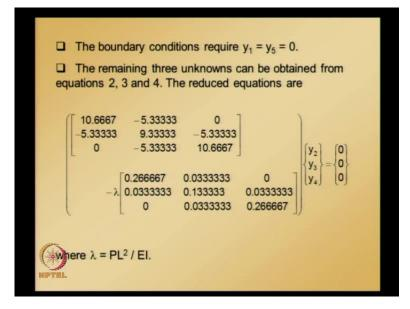
So, these are the boundary conditions y 1 y 5 is equal to 0 because, essential boundary conditions for this problem or y evaluated at x is equal to 0 0, y evaluated at x is equal to L is 0.
