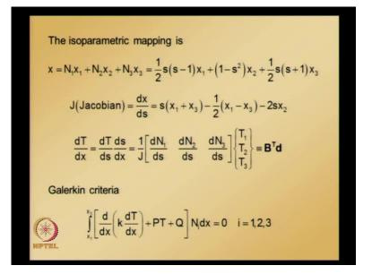
So, Galerkin criteria given differential equation, we need to multiply with weight function integrate over the problem domain and equated to 0 and here, when we are use adopting finite element weight function is same as shape function.
