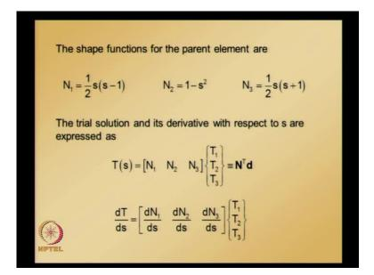
The shape functions for parent element also we have derived in the last class and they are reproduced here. Shape functions for parent element or these are the shape functions by substituting s is equal to 1, we can notice that N 1 is equal to 1 and N 2 N 3 are equal to 0. Similarly, similar kind of check can also be made by substituting s is equal to 0 in N 2 and also s is equal to minus 1 in N 3.
