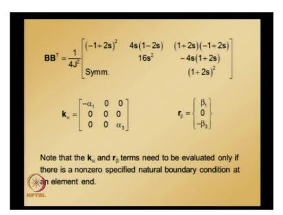
So, once we know all these values we can easily write the element equations for a quadratic element for this particular general one dimensional boundary value problem. And, please note that here, this k alpha and r beta shows up only if non-zero specified natural boundary conditions are present. Note that k alpha and r beta terms needs to be evaluated only if there is a non-zero specified natural boundary condition at an element end.
