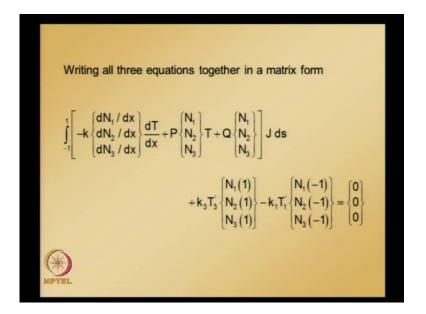
Now, I take values 1 2 3; so, expanding this, that is writing all the equations all 3 equations together in a matrix form, we are going to get this. Please note that here shape function N 1 is going to be 1 when it is evaluated at s is equal to minus 1 and shape function N 3 is going to be 1 when it is evaluated at s is equal to 1 and N 2 is going to be 0 for s is equal to minus both for s is equal to minus 1 and s is equal to 1.
