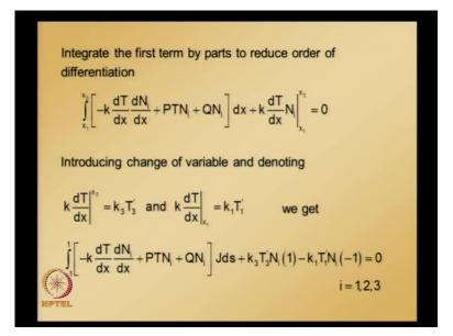
We have seen this kind of procedure earlier and we are solving problems using Galerkin criteria. So, same procedure you can adopt to do this integration by parts. Now, introducing change of variables because we need to change the limits of integration from  $x \ 1$  to  $x \ 2$  to minus 1 to 1.
