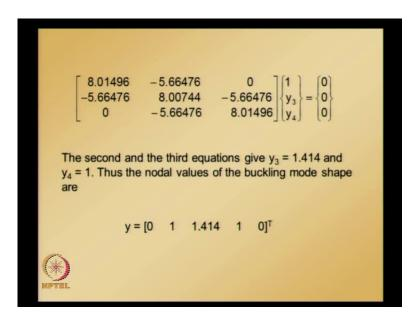
So, following the same procedure setting y 1 is equal 1 and solving for y 3 y 2 sorry, setting y 2 is equal to 0; y 2 is equal to 1. Solving for y 3 and y 4, we get the buckling mode shape. So, second and third equations give y 3 and y 4; thus, the nodal values of buckling mode shape are y 1 is equal to 0 which is essential boundary condition. y 2 is arbitrarily equated to 1 and we solved for y 3 and y 4 which happen to be 1.414 and 1 and y 5 is again 0.
