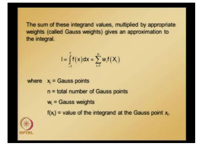
That is the reason why Gaussian quadrature is so popular in finite element method or in fact, in any other numerical technique like boundary element method. In Gaussian quadrature, the integrand is evaluated at predefined points called Gauss points and sum of these integrand values multiplied by appropriate weight called Gauss weight, gives an approximation to the integral.
