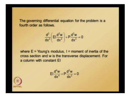
So, the governing differential equation for this simply supported column buckling problem, is a fourth order differential equation subjected to the boundary conditions. Here E is Young's modulus, I is moment of inertia of cross section, w is transverse displacement and for a column with constant EI.
