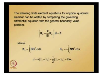
Before we proceed further, we can make a comparison of both equations. Comparing this equation with general form, we see that the corresponding variables we can identify and once we identify the corresponding variables, we can write the element equations. The following finite element equations for a typical quadratic element, can be written by comparing the governing differential equation with general boundary value problem.
