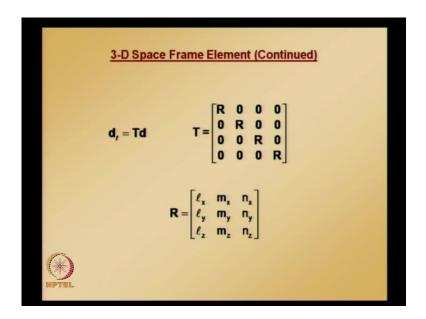
This is the transformation for the displacement vector in the local coordinate system, with the displacement vector in the global coordinate system, where R here is the rotation matrix - 3 by 3 rotation matrix - and 0 is also 3 by 3 null vector. So, transformation matrix is going to be 12 by 12 matrix and this rotation matrix comprises of all the direction cosines - L x m x n x L y m y n y L z m z n z.
