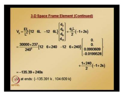
So, for element 1 axial force is obtained using this; all units are in f p s units and shear we need to apply the fixed end correction corresponding to distributed load and this is going to be function of s.
