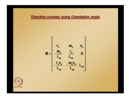
This is r matrix and this is the formula for obtaining direction cosines using orientation angle method. For the case in which a local x axis lies in the same plane as global xy,
