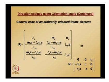
This what we saw in the last class; the last case is general case of arbitrarily oriented frame element; in this case, first thing what we need to do is we need to rotate the given frame element about local x axis such that local y axis is parallel to the global y axis.
