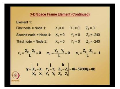
Now, we need to assemble the element equations for each of these elements, for that we need to get the rotation matrix; we will start element 1 node 1 the coordinate values; node 2 coordinate values; and, we identify what is node 3 for third node for element 1 that is node 2; the values of coordinates are given, so using this we can calculate  $L \ge m \ge n \ge n \ge n \ge n \ge \infty$ .
