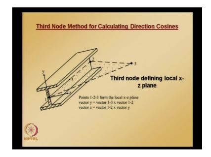
Schematically, it can be explained using this figure; here, an arbitrarily oriented space frame element is shown in which local x axis is in such a way that it is a vector going from node 1 to node 2 and local z axis and local y axis are also shown; in addition, a third node is also shown in the figure to define x z plane.
