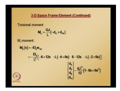
Using these formulas we can calculate axial force components of shear and torsional moment; here, in the formulas we have the nodal values d 1 to d 12 and these have the same meaning as what we have seen in the last class - they comprise of all the 3 translation degrees of freedom at node 1; 3 rotational degrees of freedom at node 1; again 3 translational degrees of freedom at node 2; 3 rotational degrees of freedom at node 2.
