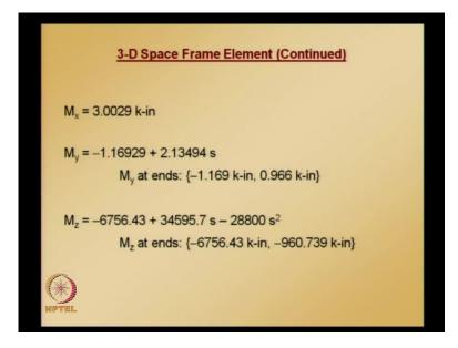
Similarly, m z component - simplification of that gives us m z component in terms of s so by substituting s is equal to 0 and s is equal to 1 we get m z values at nodes 1 and 4 and torsional moment m x, and these are the axial forces, shear moment and torsional moment for element 1; similar calculations can be repeated for element 2. Details are not given here - final values are given; this is a torsional moment M x M y M z.
