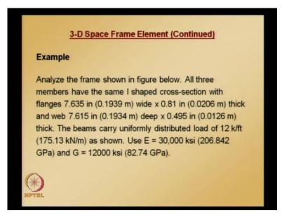
This is the procedure; now, let us take a numerical example: analyze the frame shown in figure - figure will be shown in the next slide - all members have same I shaped cross section and the flange dimensions web dimensions and depth are given both in f p s units and s i units and beam carries uniformly distributed load which is shown in the figure and material properties are also given.
