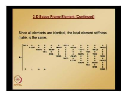
From the dimensions and cross section properties we can get these values that are given, and from this we can calculate what are the coefficients - a 1 a 2 a 3 a 4, for each of the members; but, in this particular problem all the members are identical and since all elements are identical local elements stiffness matrix for all elements is same, which is
