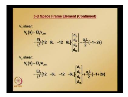
Shear - v y capital V is used to denote shear as a function of s again s is equal to 0 corresponds to node 1 s is equal to 1 corresponds to node 2 is given by this; and, you can see the second part in in this equation it is correction term for fixed end solution; here, the correction term that is I have shown in the slide is corresponding to uniformly distributed load case.
