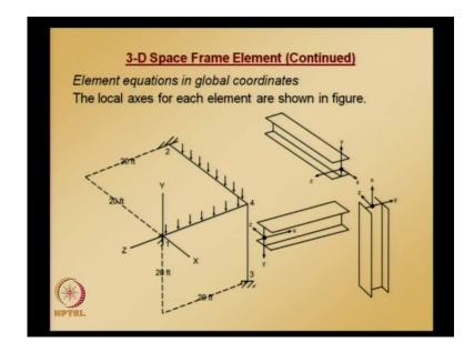
Now, element equations in global coordinates - we obtained element equation in local coordinate system; to get element equations in the global coordinate system we need to apply transformation method.
