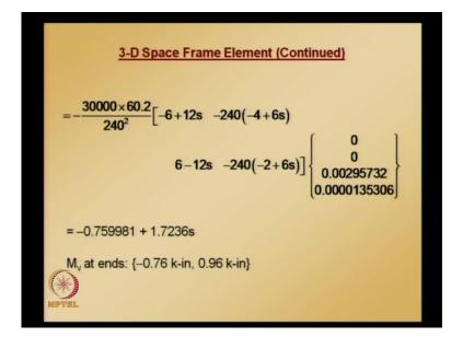
Similarly, the other shear component V z and its constan,t and moment m y with fixed end solution correction; simplification of that gives in terms of s, s is equal to 0 corresponds to node 1 s is equal to one corresponds to global node 4 m y value at these nodes 1 and 4.
