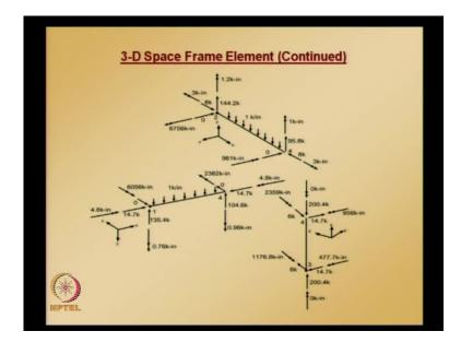
Similarly, for element 3 axial force, shear components, moments; once we obtained axial forces, shears, moments we can draw free body diagram - the forces can be shown on element free body diagram like this and we can check the equilibrium of each of these elements for numerical accuracy, and also we need to make sure that all the elements put together are in equilibrium.
