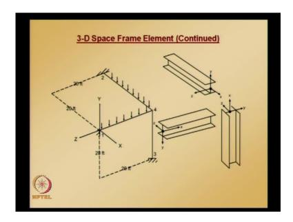
Using this information we can find - and once we know the coordinates of nodes 2 and 4 you can easily find what is this rotation matrix; similarly, for node 3 - so for element 3 which is connecting nodes 3 and 4, the orientation angle is 1.5 times pi, that is, 3 pi by 2 radiance or 270 degrees.
