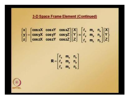
We require that in addition to the coordinates of the n points of the space frame element; so, this is the data that is required for orientation angle method. Now, let us briefly look at that method - this rotation matrix consists of direction cosines, these are coming from the coordinate transformation from the local x y z to global x y z consisting of all direction cosines.
