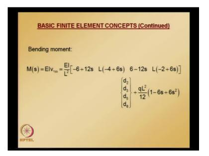
Similarly, we can also calculate bending moment where also, we need to apply fixed end solution correction. So, this is the procedure for solving frame problems to illustrate this procedure; let us take an example.
