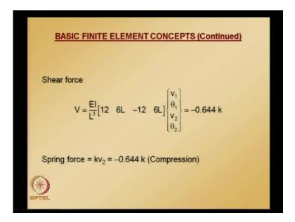
So no shear for shear force node correction, because of the temperature affects is required and the shear force is given by this formula using the third derivative of shear functions, finite element shear functions for beam element and using the nodal values we get this shear force value.
