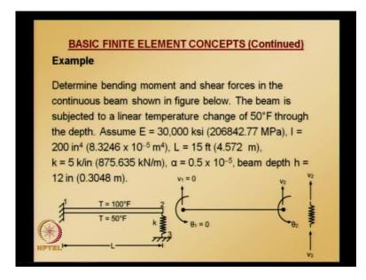
Determine bending moment and shear force in the continuous beam shown in the figure. And, the beam is actually, it is a beam and a spring combination is there. The beam is subjected to linear temperature change and all units are given in both FPS and SI units, since the numbers given in FPS units are round numbers.
