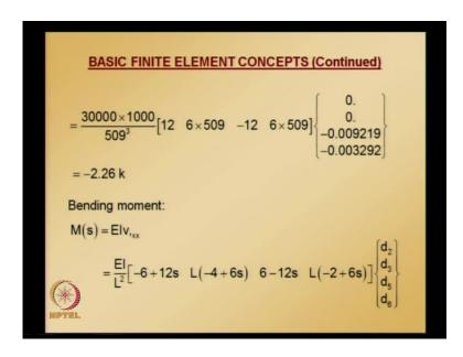
Substituting these values d 2 d 3 d 5 d 6, we get shear and bending moment is given by this using the transverse displacement values and rotations. Please note that when we are calculating either shear force or bending moment, we are not applying any fixed end solution correction because, element 1 is not subjected to any distributed load.
