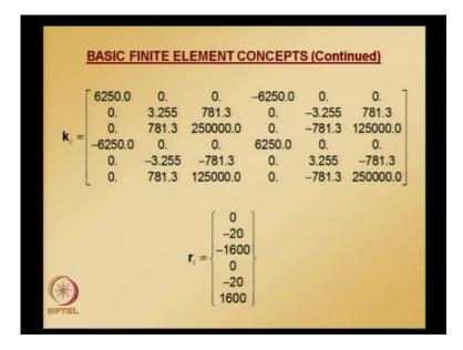
Please note that this element is oriented along the direction of a global x axis. So, local x axis and global x axis are in the same direction. Transformation matrix is going to be identity matrix; so local the stiffness matrix for element 2 in the local coordinate system will be same as stiffness matrix for element 2 in the global coordinate system. So, now this is a load vector for element 2 in the local coordinate system.
