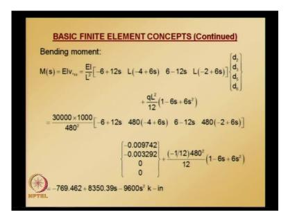
So, the first part of this calculation is coming directly from the nodal values and finite element interpolation and the second term is fixed end solution correction and substituting the numerical values we are going to get shear which is linearly varying. Shear force at node 2 is given by substituting s is equal to 0. Shear force at node 3 is obtained by substituting s is equal to 1 in this, so shear force at the ends.
