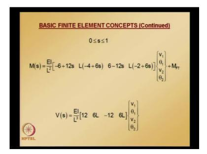
Now, moments similarly, correction term is there, in addition to the finite element interpolated values and please note, that there is no shear because of these thermal stresses and fixed end condition. So, there is no correction term for shear force to get clear idea about how to approach a problem using all these concepts; let us take an example.
