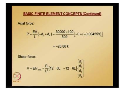
So, nodal solution in the local coordinate system because, we require when we are calculating axial force shear force and bending moment, we require local nodal values nodal values in the local coordinate system and once we get the local displacement vector or the displacement vector in the local coordinate system, we can apply the formula for axial force.
