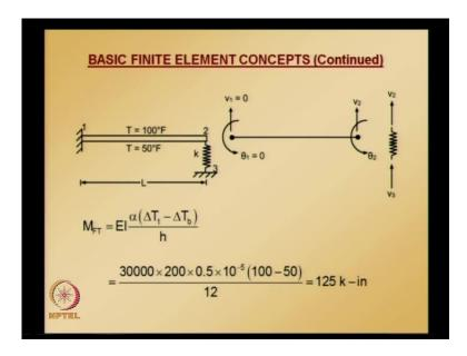
So, using these values we can calculate what is M FT and this is what is shown here. Please note, that we are working out in FPS units and we got M FT. Following the sign conventions for applied moments and shears and putting the fixed end solution in a vector form and reversing this sign, we are going to get equivalent nodal vector for beam element.
