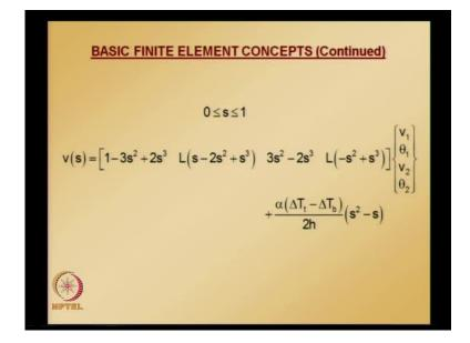
Let us see in detail all the steps by taking an example. Once, we get the nodal values we get, we can interpolate by using this equation displacements and this is what I mentioned. The first term is finite element interpolation; interpolation using finite element shear functions and second term is the correction term which is obtained by integrating the curvature; that is expressed by the beam element twice.
