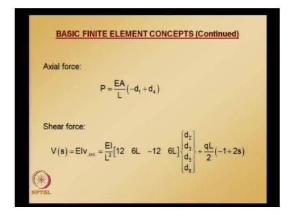
For that kind of element axial degrees of using the computed degrees of freedom, we can find axial force in frame element and also shear force. Since this frame element is subjected to distributed load, we need to apply fixed end correction and s goes from 0 to 1 s, 0 s is equal to 0, corresponds to node 1 s is equal to node 1 corresponds to node 2.
