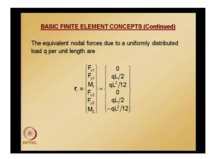
Now, what are the equivalent nodal force vector forces due to the uniformly distributed load applied on the frame element? That is shown in the figure when we started out this
