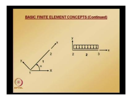
So, now by choosing arbitrarily, element 1 goes from node 1 to node 2 and element 2 goes from node 2 to node 3. The local coordinate system for each element shown here: x axis is oriented along the axis of the member and y axis is at 90 degrees with respect to x axis in the counter clockwise direction.
