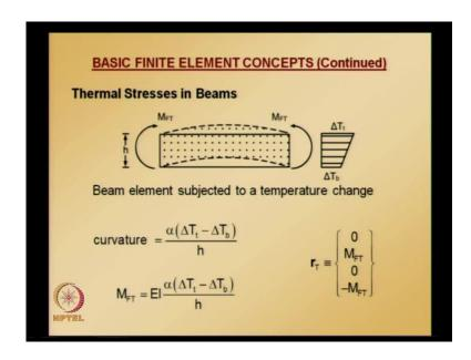
Considering a beam element which is subjected to a linearly varying temperature over its depth, we developed the equations and this is the beam element subjected to a temperature change at delta capital T subscript t, is the change in the top surface temperature delta capital T subscript b is the change in the bottom surface temperature; h is the depth of the beam.
