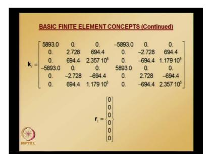
Stiffness matrix for element 1 in the global coordinate system is given by T transpose k l T. Please note that this element 1 contribution goes into the locations and at node 1, you have, or at each node you have 3 degrees of freedom. So, element frame element 1 is connecting nodes 1 and 2; so the contribution goes into 1 2 3 4 5 6 rows and columns of the global equation system.
