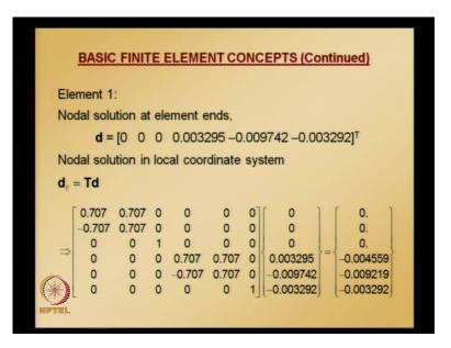
Element 1, the nodal solution that we get, that we obtained just now is written here. That is, u 1 v 1 theta 1, u 2 v 2 theta 2 values. This is the global displacement vector and we need to find local displacement vector using the relation coming from transformation matrix; that is d l is equal to T times d.
