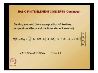
So bending moment here, we need to apply the fixed end solution correction. That is what is done; bending moment from superposition of fixed end temperature affects in finite element solution.
