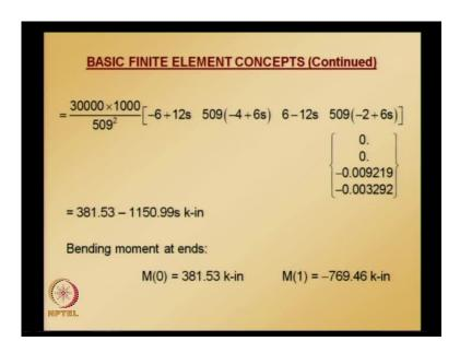
Substituting the numerical values, we get moment and we can calculate from this what is the bending moment value. Shear is constant whereas, bending moment is having linear variation. So, bending moment value at node 1 is obtained by substituting s is equal to 0; bending moment at node 2 is obtained by substituting s is equal to 1.
