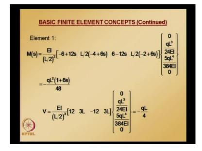
So, using these nodal values - element, bending moments and shears can be calculated for element 1 and element 2. And also you can see these values that we calculated that is, theta 1 v 2 theta 2 and theta 3 all match exactly with the exact solution which is already shown to you.
