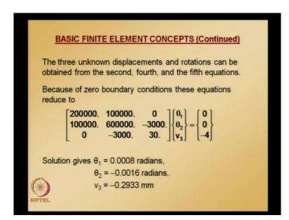
So, we can eliminate 1, 3 and 6 rows and columns and get the reduced equation system. So, we get solving this equations system - reduced equation system - we get theta 1, theta 2 and vertical or transverse displacements at node 3. The solution of this equation system gives us these values; please note that rotations are in radians.
