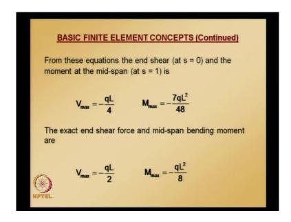
So, from this equation the shear at the left end, that is, s is equal to 0 and moment at midspan at s is equal to 1 or these values. And the exact values exact shear end shear force and midspan bending moment are these values.
