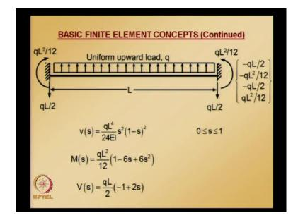
So, now, for example, if we take a fixed end beam subjected to uniform upward load, the displacement, bending moment and shear at any point along the span are given by these formulas, where s goes from 0 to 1, s is equal to 0 corresponds to the left end; s is equal to 1 corresponds to the right end.
