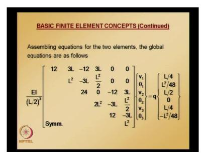
So, that is simplified form of each element equation. Assembling equations of two elements, global equations are obtained as follows. And now, for the 2 element model that we have taken, node 1 is at the left support and node 3 is at the right support. So, v 1 and v 3 are going to be 0, because we have supports at node 1 and node 3.
