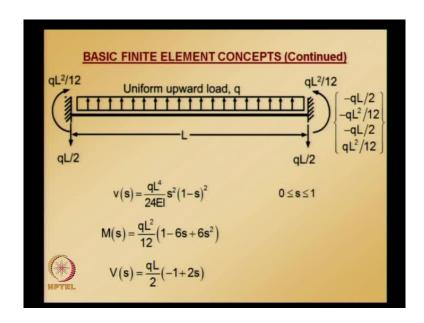
So, for example, for the case of uniformly distributed load using exact fixed end solution what we can do is, these are the exact fixed end beam solutions that is for transverse displacement, movement and shear.
