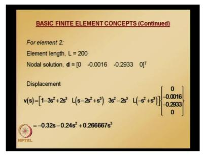
Similarly, we can repeat the process for element 2. Element 2 length and the nodal solution that is v 2 theta 2, v 3 theta 3 are given here and using this displacement at any point along the length of the second element can be obtained by substituting these values and this equation gives you displacement that is transverse displacement at any point along length of element 2.
