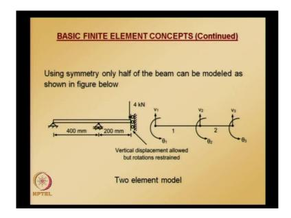
So, here, this if you see this three span continuous beam, it is symmetric about the midpoint; so using symmetry, only half of the beam can be modeled. Taking symmetry into account, the given problem can be solved using half model like this, and here this soft model is discretized using two elements - element 1 having degrees of freedom of v 1 theta 1 v 2 theta 2; element 2 having degrees of freedom v 2 theta 2, v 3 and theta 3.
