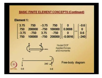
So, how we get bending moment and shear at element ends? We go to the element 1 equations, we substitute in those equation system, we substitute what is v 1 theta 1, v 2 theta 2, and calculate the bending moment and shear at x 1 and at x 2, that is node 1 and
