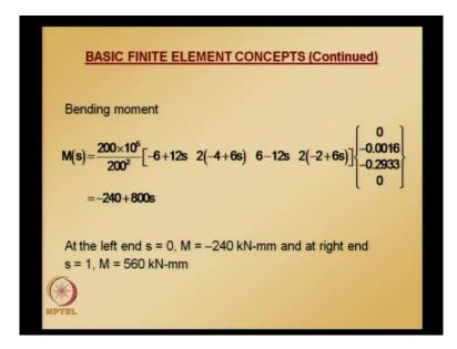
And similarly, bending moment - substituting the nodal values corresponding to element 2, we get bending moment. And again substituting s is equal to 0 we get what is the
