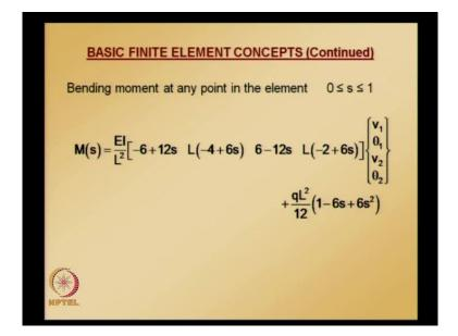
So, the correction factor is shown, whatever is shown the second term is a correction factor, which is coming from fixed end solution. And bending moment at any point, once we get the nodal values as usual we can calculate bending moment at any point along the beam length and to that we add fixed ends solution.
