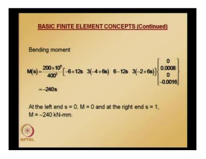
So, in this equation you substitute what is v 1 theta 1, v 2 theta 2 and by sweeping s from 0 to 1, we get the displacement values at any point along the length of the element 1. (Refer Slide Time: 14:33)
