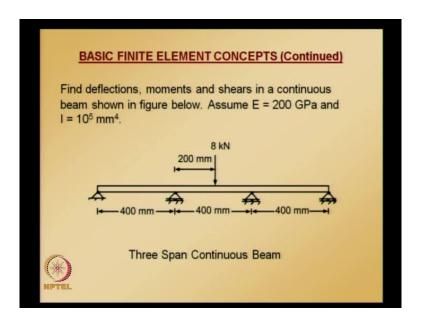
So, now, we are ready to solve an example. Let us take a simple example, find the deflection moments and shears in continuous beam shown in figure below, material properties and geometrical properties of the section of the beam are given. These are three span continuous beams and each span is of length 400 millimeters and in the central span 8 kilonetwon point load is applied at the center of the midspan.
