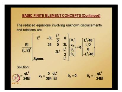
So, we get reduced equation system and which we can solve for theta 1 v 2 theta 2 and theta 3 and if you solve, this is the reduced equation system and if you solve this equation system using any of the symbolic computations or the software which can do symbolic computations, if you can solve this equation system, we get solution for theta 1 v 2 theta 2 v 3.
