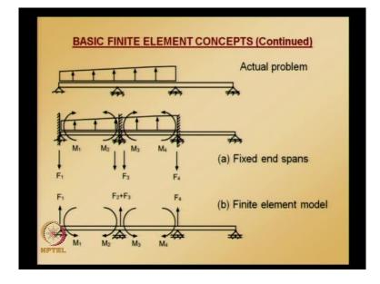
So, let us assume, the first figure shows the actual problem and regardless of actual supports in the first problem, the element ends are assumed to be fixed against any displacement or rotation such as structure will experience moments and shears in the loaded span alone and that is, each loaded span is independent, fixed end beam. Exact solutions for these fixed end beam problems are easily available in elementary mechanics of material books.
