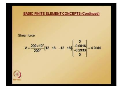
And now, shear force is again constant over entire length of element 2. And now, please note that, whatever shear and bending moment that we calculated, they are all internal shear and internal moment values. So, we need to whenever we try to draw this or put this in a form of plot, we need to follow sign conventions corresponding to the internal moment and internal shear that we already started out with.
