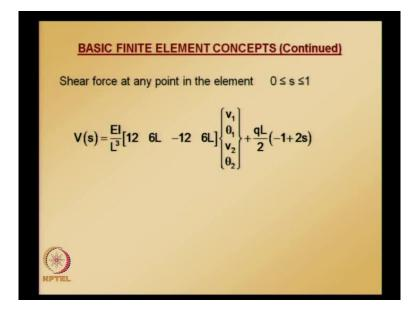
Please note that here, this fixed end solution corresponds to uniformly distributed load and if you have some other load, then we need to add fixed end solution corresponding to that particular load. And shear, we need to add the correction factor, which is the second term in this equation.
