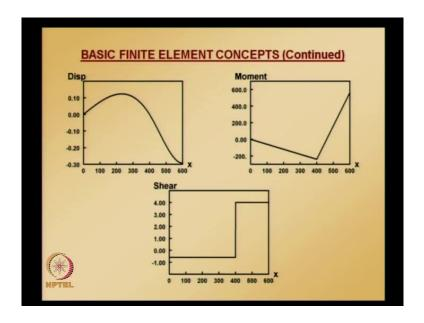
So, using these we can plot. So, the plot of displacement moment and shear looks like this. And if you are concerned, whether this, the values that you computed are correct or not, there is always a check for verifying the results and to do that it is instructive to draw free body diagrams using bending moment and shear at element ends.
