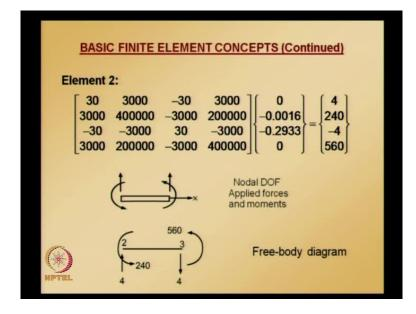
Similarly, for element 2, substituting the values of v 2 theta 2, v 3 theta 3, we get what are the bending moment and shear forces at the ends of element 2 and it turns out after doing this calculation it turns out that this values are given there 4, 240, minus 4, 560.
