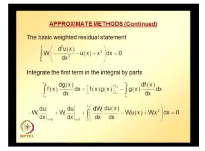
So, now applying the Galerkin criteria, basic Galerkin criteria over this weight function times the difference between the left hand side and right hand side or the residual integrated over the problem domain equated to zero. Since, this is the basic Galerkin criteria and here the demand on the starting trial solution we want to reduce it.
