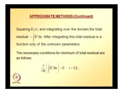
So, squaring residual and integrating over the domain, total residual is going to be integral zero to one residual square d x. After integrating this total residual it is going to
