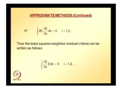
So, this is the necessary condition. And this necessary condition can further be simplified by noting that integration and differentiation are interchangeable and taking differentiation inside we get this equation and here u is sorry two is can be cancelled out on both sides and we get this equation. So, weighted least square weighted residual criteria can be written like integral zero to one partial derivative of a with respect to a times e d x is equal to zero.
