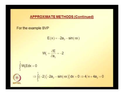
So, applying this to the problem that we are looking at for the boundary value problem that we had looking at residual is given by this. So, weight function is partial derivative of this residual with respect to the unknown coefficient a 2 it gives us minus 2. So, once we have this weight function or weight w 2, we can take this w 2 and multiply with the residual and integrate over the problem domain between zero and one equated to zero here residual is a function of a 2.
