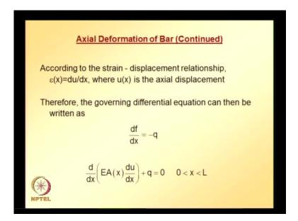
We know that according to strain-displacement relationship, strain epsilon is derivative of u or derivative of displacement with respect to x, where u is axial displacement and so substituting all this that is f is equal to stress times area of cross section. Stress is given by young's modulus time strain.
