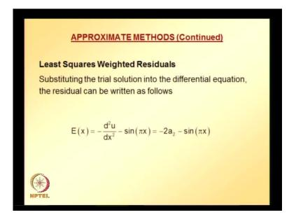
So, once we have this, we can actually substitute into the residual in least square weighted residual method substituting trial solution into the differential equation residual can be written as follows. And as you can see, here residual is having only one unknown coefficient need that needs to be determine a 2 and in least square weighted residual method weight function is residual itself.
