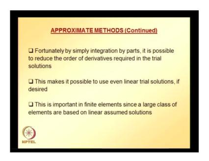
So, is there a way that we can reduce this demand on the starting trial solution, that is, the question and there is an answer to that also fortunately by simple integration by parts it is possible to reduce the order of derivatives required in the trial solution. And this makes it possible to even use linear trial solution if desired. And this is very important in
