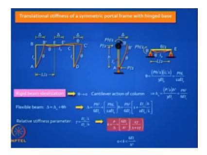
Take the rigid beam idealization. Do you agree to this? Cantilever action of the moment of the column. You get  $delta_0$  equal to this quantity, which we just derived.
