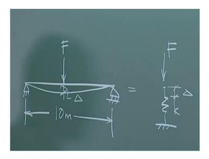
Both of them are simply supported beams. What is a span of the beam?
