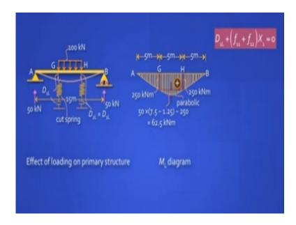
You need to now find out  $D_{1L}$ ,  $F_{11}$ , and  $F_{12}$ . First thing is you need the bending moment diagram when  $X_1$  and  $X_2$  are 0, in the primary structure. That is easy to do. You have a UDL, you have a parabola in the middle, and you have two straight lines. Those areas are easy to compute.
