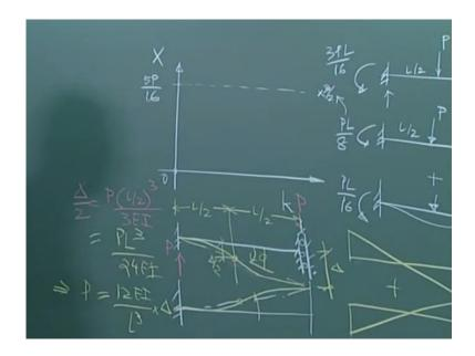
P into L by 2 the whole cube by? It is a small cantilever and I can cut it there by 3 EI. It is a clever way of solving the problem. So, this turns out to be... Remember this. This is PL cube by 24 EI, or you can say P is equal to 12 EI by L cubed into delta. So, you have a relationship between this delta and this P. It is very important to remember this relationship. Now, what is your moment? You get a moment here. (Refer Slide Time: 47:50)
