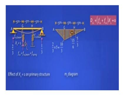
Then, you apply  $X_1$  equal to 1. That means, you pull that spring down by  $X_1$  equal to 1 and you have a force in the spring, but you also have a bending moment in the beam.
