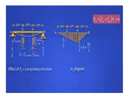
Then, you pull the other spring down with the unit load you have  $m_2$  diagram, which is the same as the  $m_1$ , but laterally inverted. So, you have these diagrams.
