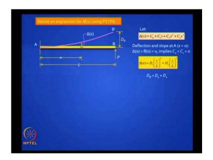
Let us demonstrate how you do this. Take that same cantilever beam problem. Let us derive an expression for bending moment, not using the conventional direct equilibrium, but we go the long winded way through energy formulation, assuming a displacement profile and figuring out what could be an expression for bending moment.
