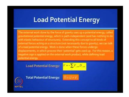
There is a term invoked in energy methods called Load Potential Energy. That is a concept which you need to understand. It is given here that, the external work done by the force of gravity uses a potential energy, called gravitational potential energy, which is path-independent and has nothing to do with the elastic behavior of structures. Every body subjected to the force of gravity has the potential to do work - that is gravitational potential energy.
