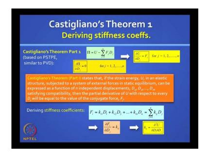
The more popular use of this is Castigliano's Theorem, which can be derived from this principle. So, Pi can be written as U plus V. V is written as minus sigma  $F_j D_j$ . When you invoke the principle of minimum total potential energy, you will find that this will reduce to dou U by dou  $D_j$ , which is equal to  $F_j$ . In this form, it is known as Castigliano's Theorem - Part I. It is similar to a principle of virtual displacement.
