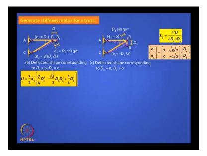
Let us demonstrate this with a simple example. Here are two bar truss. It has two degrees of freedom. Joint D can move horizontally, it can also move vertically, and the elongations  $e_1$  and  $e_2$  can be expressed in terms of  $D_1$  and  $D_2$ . We can easily prove this.  $e_1$  is equal to  $D_2$  and  $e_2$  is equal to  $D_2 \cos 30$  degree.
