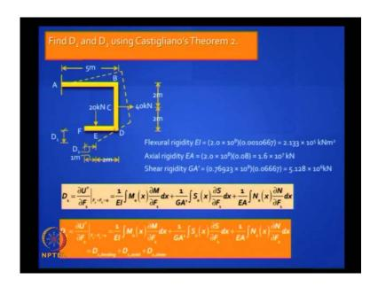
That is called the theorem of least work. Let us demonstrate this with a problem. You remember we did this problem, finding  $D_1$  and  $D_2$  using unit load method. Here, let us make it more complex by including actual deformation and shear deformations. I will go through it fast. You can find it using Castigliano's Theorem.
