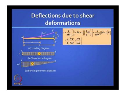
We can see that the shear force diagram, shows a constant shear force P and the bending moment diagram. In this case, it is a sagging bending moment diagram, linearly varying. If you want to find the strain energy in this system, it is easy. You can use that formula, but now we will include shear strain energy as well.
