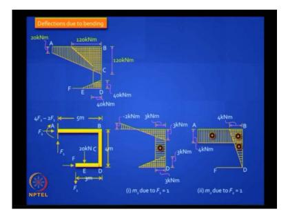
First, find the deflections due to bending. You have a bending moment diagram. To find  $D_1$ , you apply  $F_1$  equal to 1. You will get the unit load bending moment diagram  $m_1$ . To
