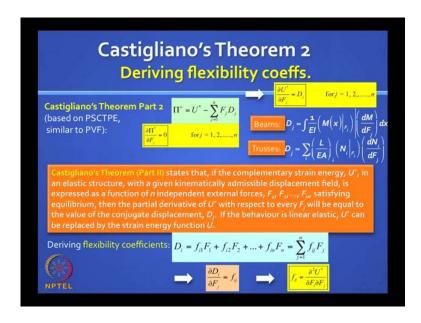
You can do the same thing using Castigliano's Theorem, part II. Here again, you can prove using a similar procedure, dou U star by dou  $F_j$  equal to  $D_j$ , for 1 to n. Here, you
