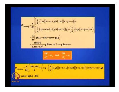
You can work out the same method. It resembles a unit load method and you can find that the deflection caused by bending is 5.61 at point one and if you want at  $D_2$ , it is something. You can also find deflection caused by shear using these similar expressions.
