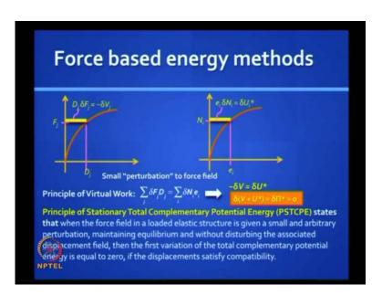
The principle in this form states that when the force field in a loaded elastic structure is given a small and arbitrary perturbation, maintaining equilibrium and without disturbing the associated displacement field, then the first variation of the total complementary potential energy is equal to 0, if the displacements satisfy compatibility.
