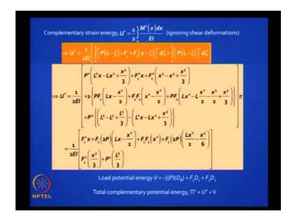
You can expand this by ignoring shear deformation. Write an expression for U star can be generated easily. This is U star -- the full form of U star. This U star is a function of not only p, but  $F_1$  and  $F_2$ .
