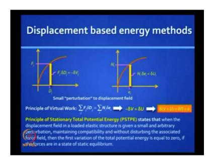
The Principle of Stationary Total Potential Energy (PSTPE) states that when the displacement field in a loaded elastic structure is given a small and arbitrary perturbation, maintaining compatibility and without disturbing the associated force field, then the first variation delta pi, first variation of the total potential energy is equal to 0, if the forces are in a state of static equilibrium.
