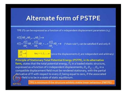
In this form, that same theorem says that when Pi is expressed as a function of independent displacements  $D_1$ ,  $D_2$ , etcetera in a compatible displacement field, it must be rendered stationary, with the partial derivative of Pi with respect to every  $D_j$  being equal to 0. This happens if the associated force field is to be in a state of static equilibrium.
