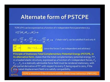
Expression of compatibility - you can go through the same procedure and can find the alternative form, which reduces to dou Pi star by dou  $F_j$  equal to 0. Earlier, it was dou Pi by dou  $D_j$  equal to 0. That one equation, that is, the first variation of  $P_i$  star equal to 0, now multiplies into n number of equations, depending on the number of independent forces that you get.
