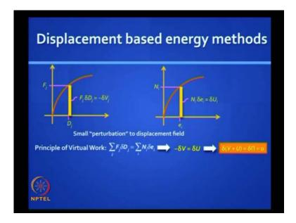
The principle of virtual work says sigma  $F_j$  delta  $D_j$  must be equal to sigma  $N_i$  delta  $e_i$ , where  $N_i e_i$  graph - the non-linear picture, may look like this and that incremental strain energy is delta  $U_i$ . First, we look at the principle of virtual work. It says sigma  $F_j$  delta  $D_j$  is equal to sigma  $N_i$  delta  $e_i$ .
