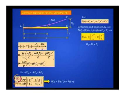
You can also derive an expression for curvature by taking the second derivative of delta x. Using this expression for curvature, you can get an expression for strain energy.
