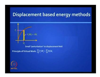
We will first look at the displacement based energy methods. So, let us take, for example, a truss. To generalize, let us assume that all the elements are elastic, but not necessarily linearly elastic. So, if the elements exhibit non-linear elastic material behavior, then the loads, the deflections that happen at the joint locations are called external component of force field and displacement field, will also show corresponding non-linear behavior.
