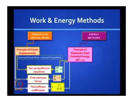
From this set of theorems, you have noticed that we finished the use of displacement based theorems. You can use it to set up equilibrium equations dou Pi by dou  $D_j$  equal to 0. You can use it to find unknown forces at Castigliano's first theorem dou U by dou  $D_j$
