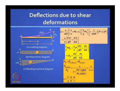
Let us try to see what is the relative contribution of shear deflection? We can take the ratio of deflection due to shear divided by total deflection and you can get this expression, which can be written in this form -  $D_B$  shear by  $D_B$  is equal to this.
