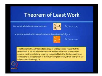
We will end with this theorem of least work, which I have already explained. For a statically indeterminate structure, dou U star by dou  $X_j$  is equal to  $D_j$ . In general, when support movements are involved,  $D_j$  is zero. This is even true for internal indeterminacy.
