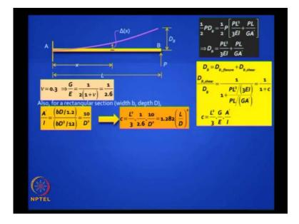
Now let us take a simple example of a rectangular section. For a rectangular section of material like steel, where Poisson's Ratio is 0.3 - that expression for C will reduce to something like 1.282 into L by D, the whole square. So, you will find that L by D span to overall depth ratio actually dictates the contribution of shear deformations to the overall deflection, to the overall energy.
