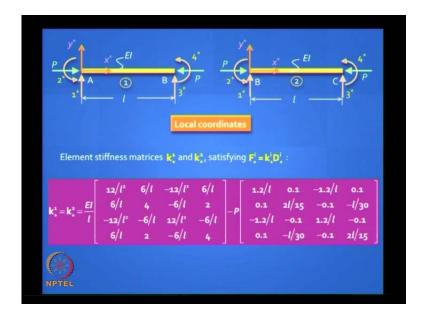
Well, that is a standard beam element. Except that, we are having a constant axial force P; it is the same P in both of them; it is the same P because it is a single column, and we write down the stiffness matrix which has the first order component which is the standard stiffness matrix, and we put a minus P to bring in the geometric stiffness part. Is it clear? So, this we know. These two matrices we have derived.
