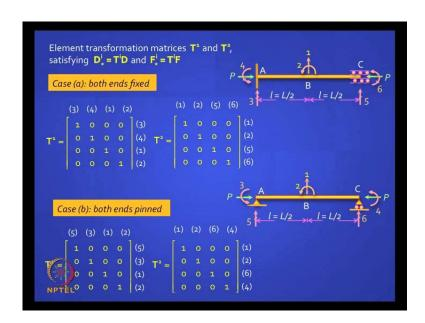
So, how do we generate the stiffness matrix for the structure? Well, first, you need the transformation matrices and they are simple. We have done this before. They are identity matrices. You have to correctly put the linking coordinates very clearly; it is 3 4 1 2 for the first element, and 1 2 5 6 for the second element, in case a. In case b, what will happen? The same T 1 T 2, but the linking coordinates will be... you have to be careful. It should be a written as 5 3 1 2.
