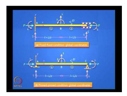
So, this is the first case. I have put it horizontally; does not matter. The column can be made horizontal. I have put a node in the middle. So, 1 and 2 active, and then, of course, I have restrained coordinates 3, 4, 5, and 6; does this is this clear?
