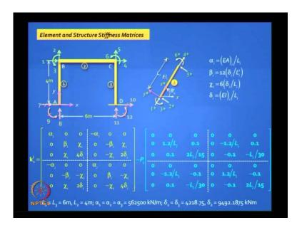
We have done this before - 3 elements, but now, when you write down the stiffness matrix, you have to make a small correction for P, but do you know P? Yes. We know one is P; there is a P for element 1 which is 2 P, and for element 3, it is P. What about element 2? Will it have any force at the point of buckling? In the deflected shape, you may get some force.
