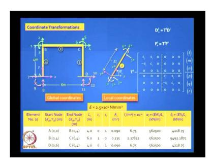
So, you write down. This is a slide; I am picking it from what we did when we did portal frames without any beam column effect, without any P delta effect. So, this is straight. From that, you have 6 degrees of freedom which are active and 6 which are restraint. You can generate the T i matrix for all of them.
