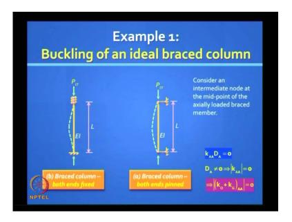
Let us apply it to very easy problems to test out this method. We know the solutions for these. We know the Euler buckling load for these two cases. They are ideal braced columns; case a - both the ends are fully fixed against translation and rotation; case b - they are fixed against translation, but they are free to rotate; it is a pinned condition.
