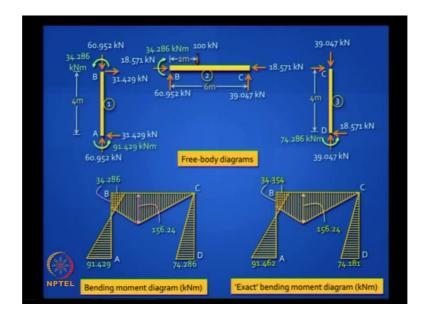
Draw the free body diagrams, bending moment diagram. Final comparison, some minor error, but certainly, No. No major error; is it clear? So, with this, we have covered reduced element stiffness method as applied to frames. Clear? Thank you.
