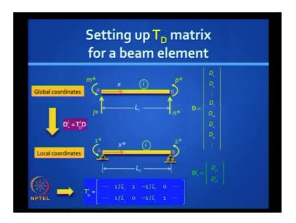
You are also familiar with what you do for a continuous beam. And if you have chord rotations, relative supports settlements, then you have to use this chord rotation which is given by 1 by L, and clockwise chord rotations are treated as negative, but the equivalent beam and flexural rotations which is 1 by L, will turn out to be positive. So, you are familiar with these two; if you put them together, then you get what you need to do for a plane frame element with 3 degrees of freedom.
