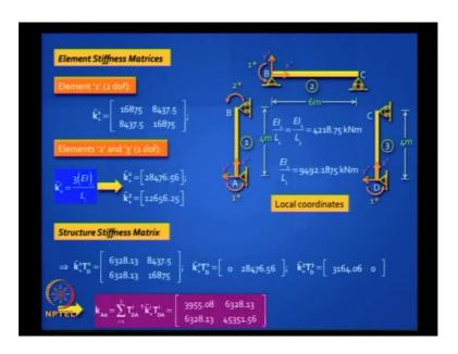
For element 1, no change. You have the same 2 degree of freedom. Elements 2 and 3; the change is 3EI by L. right So, you do that 3EI by L. Write down these values. It is a 1 by 1 matrix; very easy to calculate structure stiffness matrix you can generate; it is a 2 by 2 structure stiffness matrix right because you have only 2 degrees of freedom. Find the displacements.
