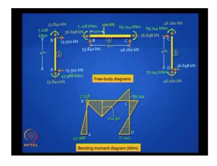
So the member end shear forces are not directly obtainable as in conventional stiffness method, but can be easily computed from the free bodies, applying equilibrium equations. So, let see how to do that. So, this is what you get from those vectors. You got the two end moments for each of the elements and you got the axial forces. If it is plus, it means extension; if is minus, it means it is compression.
