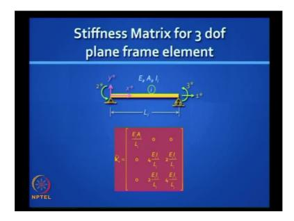
So, we are now going to use a 3 degree of freedom system, and it is very easy to write down; at this stage, you should find it very easy to write down the element stiffness matrix. You can do it from first principles.
