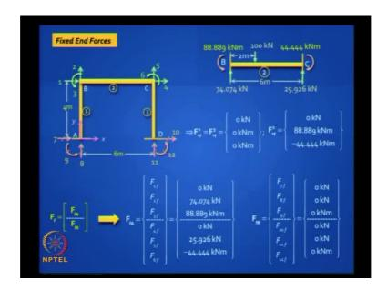
Now, what do we do? Now, we take this element alone as non-zero fixed end force vectors, and when you want to put it on to that structure, you have to do it by inspection; use a shortcut method; reduce element stiffness method; you cannot do T D transpose and get it.
