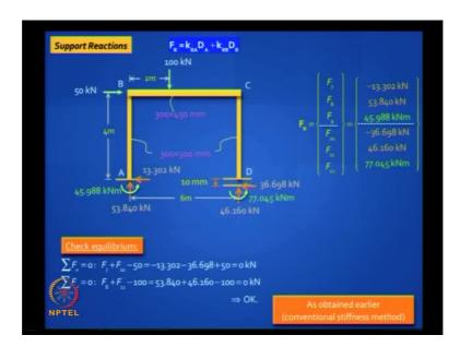
A support reaction also is identical. So, these two steps are common to both reduced element stiffness method and the conventional stiffness method. And so, you can check
