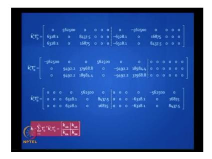
What do you do next? You generate the structure stiffness matrix. You do it in two phases; first you do this k i T D i for the three elements; all these can be done by matrix
