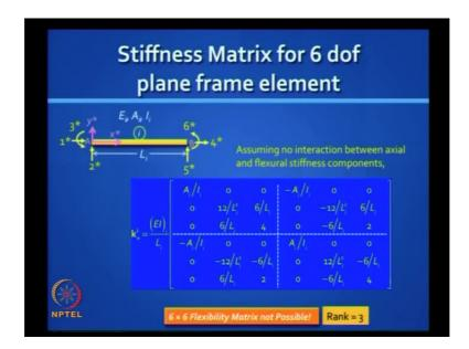
You can also do it from the 6 by 6 element stiffness matrix. how Just talk of the irrelevant rows and columns; there are 3 dependent rows and columns. If you make it simply supported, you will find that the first row is important; the second is not because we do not want the shear degrees; just delete the shear degrees of freedom, and you do
