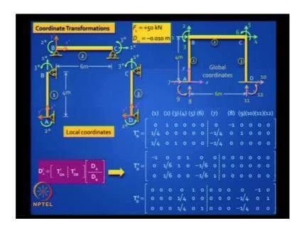
So, first, we will do the coordinate transformations. In this portal frame, we will use 6 degrees of freedom for the same 6 active degrees of freedom, which we did earlier, and 6 restrain degrees of freedom; the loading input is the same; F 1 is 50 kilo newton and D 11 is minus 0.10 kilo newton. Remember, we did the same frame with and without an internal hinge. We will also do the internal hinge in this case, and show you that you can solve the problem.
