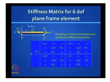
If you recall, this is the 6 degree of freedom plane frame element that we used for the conventional stiffness method. This is a large matrix and it is a singular matrix. What is the rank of this matrix? 3, and one way of understanding why the rank is 3, is because you have, mathematically, you have 3 dependent rows or columns, but physically, what does it mean? Physically For a stiffness matrix to be non-singular, what you have to make it is, you have to make the element stable.
