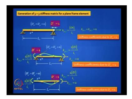
right You can also derive from first principles. You apply a unit displacement, one at a time, and you can generate these. This diagram will be very familiar to you now. It is not difficult; you can generate the element stiffness matrix.
