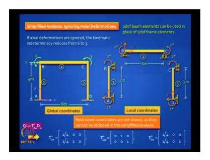
Now, is a interesting step; why should we work so hard with even that matrix? What is the advantage of ignoring axial deformations? The plane element reduces to a beam element. So, you can work with beam elements, throw away the axial deformation, and one way to check the answer is put EA tending to infinity in the problem because then it becomes actually rigid and you should get the same result, but your effort required is much less in this method.
