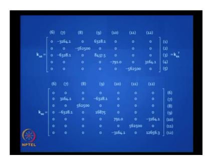
And we have to assemble the structure stiffness matrix exactly the way we did in the last class. I have explained this earlier. So you get  $k_{AA}$ . But note,  $k_{AA}$  has a size 5 by 5. Without the internal hinge, it was 6 by 6, and then  $k_{AR}$  and  $k_{RR}$  can be worked out. Please note  $k_{RR}$  will be now having a size 7 by 7. That is it.
