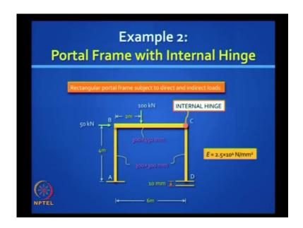
You do not need to inverse the  $k_{AA}$  matrix with the 0. Diagonal element in it moment you have a release. It will have a 0 diagonal element. So we conveniently pass it on to the restrained coordinate and it does not really matter. We do this by means of an imaginary clamp. We have done this for the beam. We are just repeating this idea for a frame.
