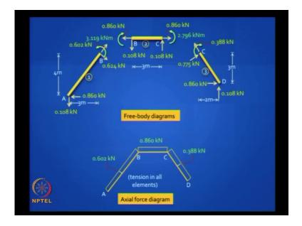
These are your final diagrams. You got axial force diagram, shear force diagram and bending moment diagram. The axial force diagram is more critical among these and you will find that they are very small.
