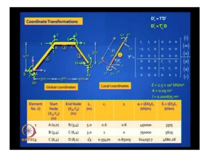
Most of these elements in the matrix will be 0s, except where you have the degree of freedom, which is active. Let us see, take the first column in these two matrices for  $T_{D1}$  and  $T_{D2}$ . The first column actually corresponds to  $D_1$  equal to 1.
