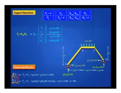
Then, you can find your support reactions solving the second equation, interpret those results, check equilibrium. The least you can do is check force equilibrium, so sigma  $F_y$  should add up to 0. Those two vertical reactions should add up to total load of 120 kilo Newton and the horizontal reactions must cancel out. It makes sense.
