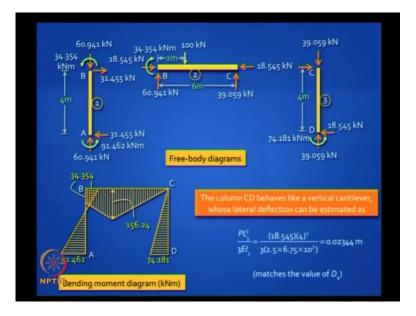
Member end forces again. The method is the same you find out for the three elements and you draw the free body diagram. What you do next? Well, the most important diagram for a frame or a beam is the bending moment diagram, but you can draw all the diagrams.
