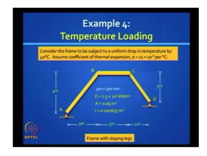
Let us go back. All the members have cross section 300 by 300, so the area is 0.09 meter squared, material has elastic modulus of 2.5 into 10 raise to 7 kilo Newton by meter square.
