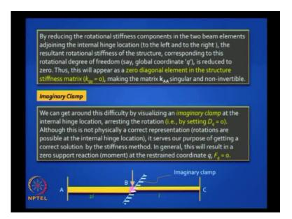
Finally, we said that we need to deal with the fact that we will end up with zero stiffness in corresponding to the degree of freedom, where we have the moment release. Because how we deal with the moment release is – we are going to shifts that global coordinates from active category to restrained category.
