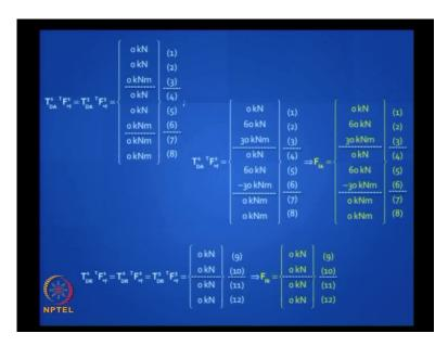
$T_D$  transpose, so that contragradient principle works. And you can sum up for do one element at a time and sum it up for the three elements. This is something you can work out for all the elements -- you get  $F_{fA}$  and  $F_{fR}$ .
