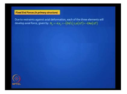
First, as you rightly said, we will find the fixed end forces in the primary structure and that is simply the axial stiffness  $k_i$ .  $N_{if}$  is  $k_i$  into E naught i. We put a minus sign in general because normally you have a rise in temperature and E naught is an extension. But in this case, E naught will turn negative, so when you substitute the results you should get a tension.
