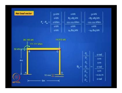
Get the net load vector or the resultant load vector. How do we do that? We do it by  $T_i$ , transpose  $F_*$ . We are just repeating what we did earlier, except that the force vector is changed slightly, and we get  $F_{fA}$  and  $F_{fR}$ , and we get the net load vector.
