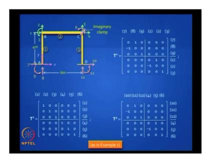
So, how do we deal with this problem, with the internal hinge? Do we need to make any changes for the transformation matrices? Absolutely no change, because it matters little whether the global coordinate is active or restrained.
