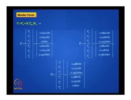
You can find the member end forces. Now you get shear forces and bending moments in addition to axial forces. But they are of small (( )). You see that value which we got 0.9 for the second element. The exact answer is 0.86, which is close to 0.9
