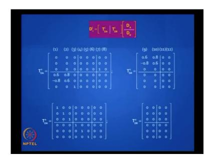
If you apply  $D_1$  equal to 1, it is going to affect elements 1 and 2. It is at the tail end of element 1 and at the beginning of element 2. So basically, you have to use this transformation matrices and fill up at the appropriate column. You see the tail end gets filled in element 1 and the start end gets filled in the element 2. It is only 1. Is it clear? I hope you know how to fill up this.
