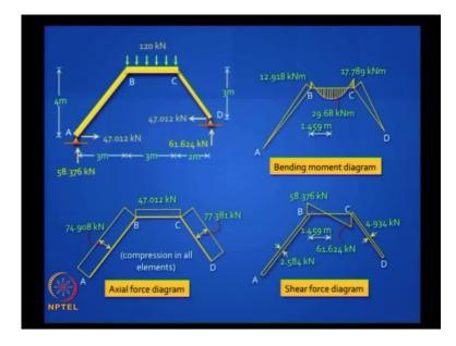
Last step is to find the member forces by using the  $T_D$  matrix and draw the free body diagrams, and draw the bending moment diagram, draw the axial force diagram, shear force diagram.
