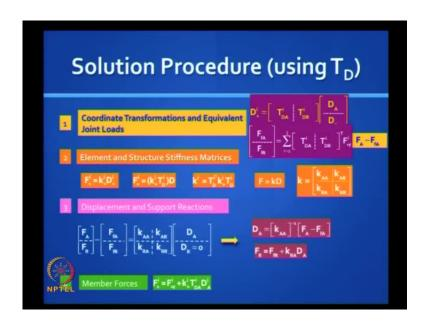
The method of analysis is identical to the previous problem, except here luckily we do not have any support settlements. Also, we are going to use a slightly different technique of generating the stiffness matrix and the fixed end force vector. We will use  $T_D$ , instead of the  $T_1$ .
