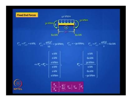
Similarly, for the third element, you can fill up now the fixed end forces. It is very easy to calculate in this case of the three elements. Only the second element is loaded. It has a UDL. so you can find the end moments and the vertical forces, write it in a vector form.
