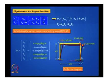
Then you solve for the unknown equations. The method is the same. You will notice that the deflections have increased substantially as compared to the previous problem. Now, you have a sway of 23.4 mm. That is how you interpret the DA vector.  $D_1$  is the sway you get at B, which is shown in yellow, and  $D_4$  is the sway you get at C.
