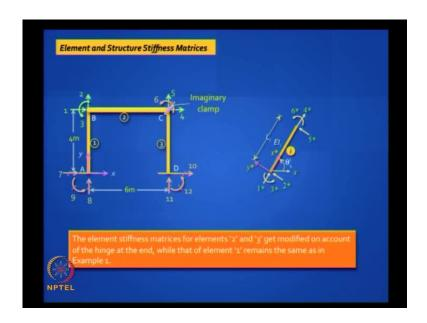
Then, we need to generate the element and structure stiffness matrices. What changes we need to do now? For element 1, any change? No, so you are right. We need to bring changes only for elements 2 and 3. Can you write them down? Can you write down the stiffness matrices for elements 2 and 3?
