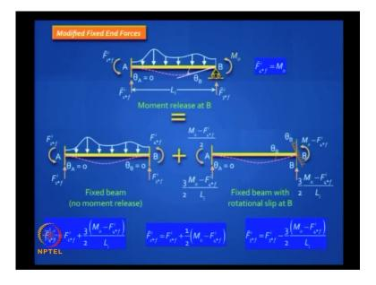
We also know that we need to modify the fixed-end forces, where you have a moment release. Essentially, the fixed beam will become like a propped cantilever and you need to modify the fixed-end moments.
