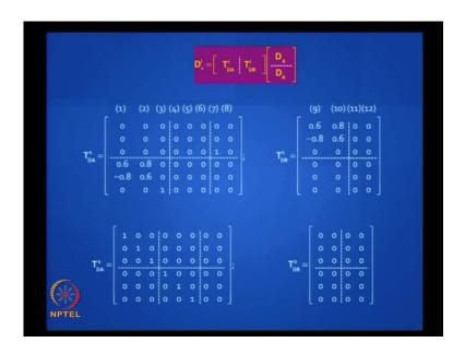
It is convenient to separate out the active degrees of freedom from the restrained. So actually the  $T_D$  matrix for each element will have a size 6 into 12, which you can partition into 6 into 8 for  $T_{DA}$  for active degrees of freedom, and 6 into 4 for restrained degrees of freedom.
