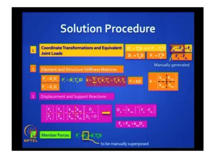
The solution procedure is exactly as we have done for all the problems till now. As you do not have any support settlements, so the steps are straightforward. We are using the reduced element stiffness method.
