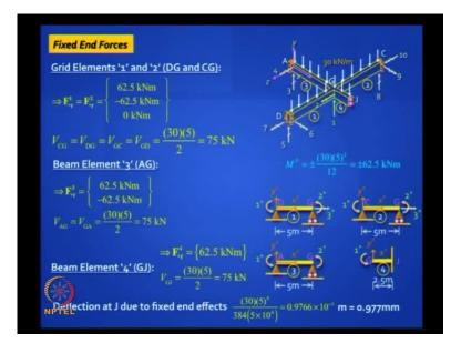
Next is fixed end forces. Luckily for you, all the beams are having a span of 5 meter and the loading is the same -30 kilo Newton per meter. So the fixed end moment is plus or minus 13 into 5 squared by 12. It is turns out to be 62.5 kilo Newton meter.
