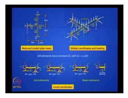
You must first visualize the physics of the problem. You can cut the beam at J. What is the boundary condition you will put there? You will put a guided roller because it can deflect but the slope is 0, so you can fix it against rotation and there is no twist there because it is a point of symmetry.
