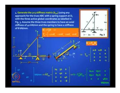
Last problem. Again simple. It is a truss. All you needed to do is to generate the stiffness matrix, nothing more, by just multiplying some matrices. This is the problem. You know how to write the T D matrix, it will look like that. You have four elements. Do not forget this. Spring is also an axial element, so it is very easy to write down. It is 4 by 3 matrix. Your k\* matrix is child's play.
