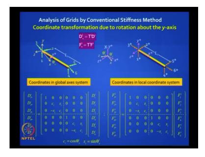
Let us see how to deal with the lack of alignment between the local coordinates and global coordinates? You have a difference between x star and x, and it is easy to write down because you remember, we have done this earlier, in the case of a truss.
