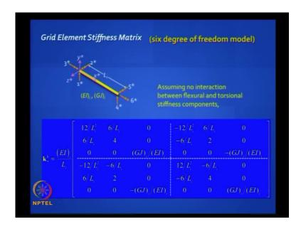
Let us look at this more carefully. We look first at the conventional stiffness method. This is the element we were talking about. The element stiffness matrix is simple if we make a basic assumption that the torsional stiffness component and the flexural stiffness components have no inter-dependents.
