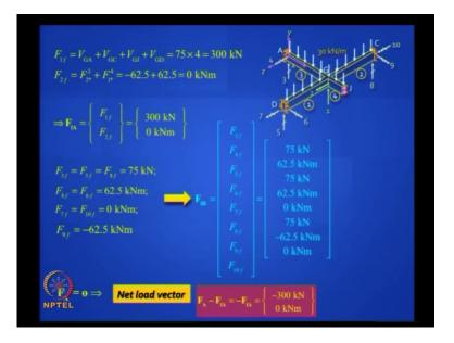
You can add up all the vertical reactions and find the equivalent force vector F A 75 into 4 is 300 kilo Newton. It is acting upward, so that is your fixed end force for F 1. F 2 gets cancelled out because minus 62.5 and plus 62.5 neutralize each other. Similarly, you can get the fixed in force vectors at the restrained coordinates. It is easy to compute.
