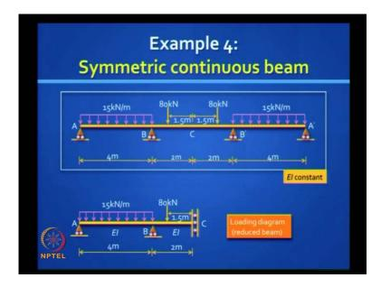
We have done this example earlier, remember, it is a symmetric continuous beam; we can take advantage of symmetry; we cut the beam at the middle at C and and insert, what kind of support, do we insert there and guided fixed, guided roller support, as shown here. And let us see, how to analyze this.
