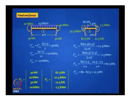
Under constrained load, the formula is minus, not minus, because now it is plus minus-since- you are dealing with the conventional stiffness method, where anticlockwise is positive. So, it is W a b squared by L squared, you know that formula, you can apply all that and you can get the fixed end force vectors.
