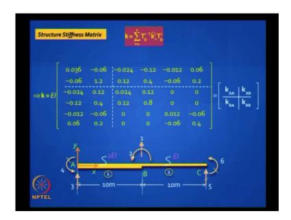
Then find the net load vector, from now on, its same as conventional stiffness method. Because, you you got beyond the element, so this part is common and of course the element stiffness matrix derivation, you have to do carefully.
