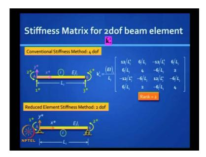
Here also, you arrested, when you have a simply supported beam. So, from now on, in the reduced element stiffness method; this is the the this is the element, that we will use for the element.
