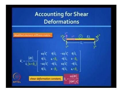
One last topic, before we move onto, reduced element stiffness method. Sometimes, it becomes necessary, to account for, shear deformations. when When do you think, you need to count for, shear deformations?
