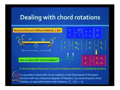
So, it is a clever trick. If you have an anticlockwise chord rotation, just, recognize that the effect it has, is that of a clockwise flexural rotation at the both the ends.
