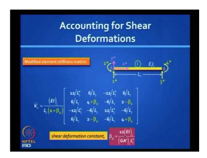
So, you have EI and you have G A dash, I, A dash. G is the shear modulus, which is related to the elastic modulus, through the Poisson's ratio. You know that.
