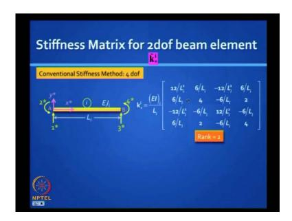
Now, we will look at the reduced element stiffness method. In this reduced.... In the conventional stiffness method, we have this stiffness matrix. I am not including shear deformations.
