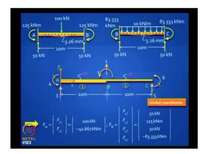
You can put,  $T_i$  transpose. Here, you cannot do that. Here, you have to do it manually, that means you draw these sketches and then you figure out. I want to find out  $F_1$ . So,  $F_1$  will be 50 plus 50, 100. Is it clear? I want to find out  $F_2$ .  $F_2$ , is this coordinate that will be, 83.33 minus 125. So, minus 46.
