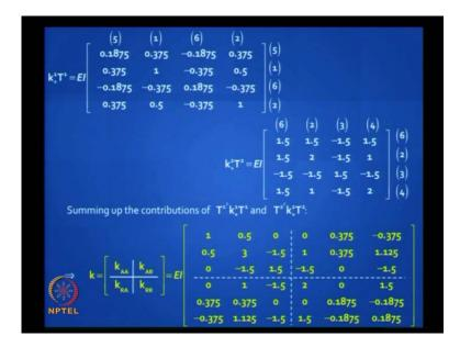
What do we do, next? We have to assemble, the Structure stiffness matrix. To do that, we have to convert, from the local axis system, to the global axis system, through the transformation-  $T_i$  transpose  $k_{\text{star}}$  into  $T_i$ .
