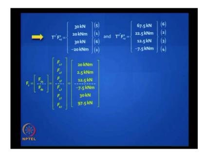
So, you are pre-multiplying by an identity matrix but you get along with it the linking coordinates and then you just you have done the slotting; you just assemble them properly. You have six degrees of freedom: three are active, three are restrained. Corresponding to one- you have 20 kilonewton meter, corresponding to two- you have minus 20 and plus 22.5, which add up, 2.5 five and so on and so forth. So, this is this can be easily assembled. Is it clear?
