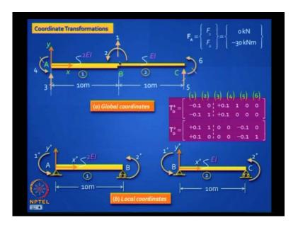
We will demonstrate this and the other rest of the procedure same, fixed end forces is only, manually supreme force or generally....So, coordinate transformation, if you look at global coordinates, these are the same coordinates; we used in conventional stiffness method; we are not changing here. Same coordinates and local coordinates are what we have just discussed two degrees of freedom, write down the transformation matrix.
