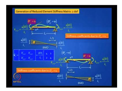
So, what do you normally do, to get the first column? You apply D 1 star equal to 1 and the moment link with that is 4 EI by L, you have a carryover moment at the other end, which is 2 EI by L. That is all, you need to worry about. Do not worry, about the reactions.
