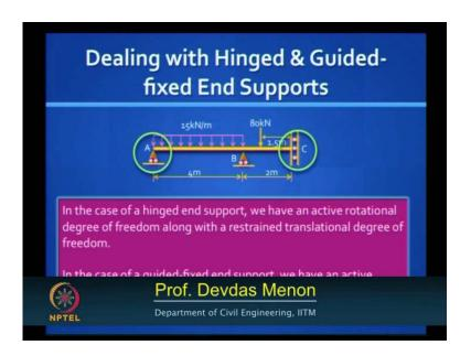
In the case of a hinged end support, as you see at the end A in this example, we have an active rotational degree of freedom, along with a restrained translational deflection degree of freedom. At support C, guided fixed end support, we have an active translational degree of freedom, along with a restrained rotational degree of freedom.
