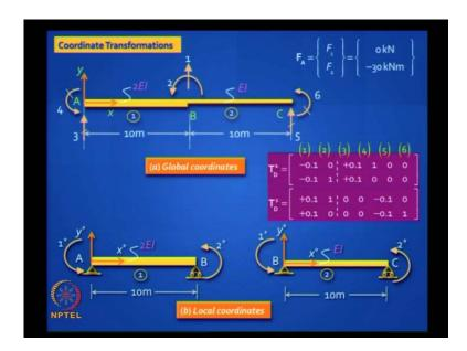
Write down the transformation, there are two matrices; you have to write  $T_D1$  and  $T_D2$ . You can to put altogether, also.
