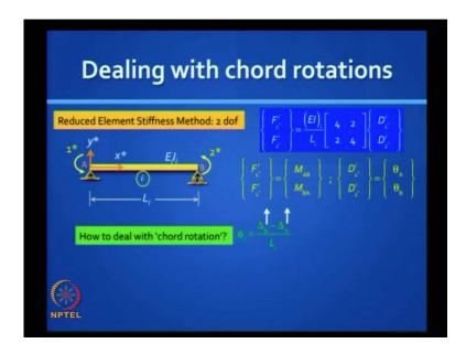
How do we, How did we manage in slope deflection and moment distribution method? Chord rotation. That is right, we use chord rotation. Normally, if you do not have chord rotation, your interpretation in this element AB is, MAB is  $F_{star}1$ , MBA is  $F_{star}2$ , theta A is  $D_{star}1$  and theta B is  $D_{star}2$ : these are flexural rotations.
