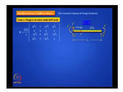
So, let us take the first one. You have got a beam, the hinge can be at one end, left end, right end or both ends, you can have 2 hinges inside a structure, so let us handle all possible. For example, the balance cantilever bridge has 2 hinges, internal hinges in the suspended span region.
