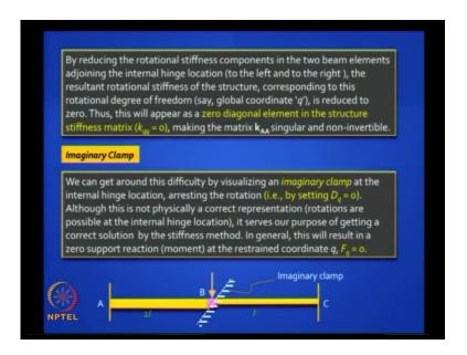
By reducing the rotational stiffness components in the 2 beam elements adjoining the internal hinge location, to the left and to the right, the resultant rotational stiffness of the structure, corresponding to this rotational degree of freedom, let us say some global coordinate q, in this example it is coordinate number 2, is reduced to 0, agreed.
