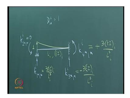
This is a hinge, this is fixed and we want to apply D i 1 star equal to 1. So, what would be the deflected shape? If I let this go up by 1, this must come back here, what will be the deflected shape? It will be like this, like a cantilever and the force I need to apply here to lift it up will be, how much this is? What I call k the ith element 1 star 1 star, what I get here is always permanently, this is k i 2 star 1 star this will always be 0 because of that hinge.
