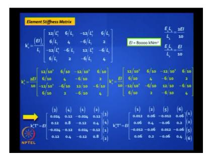
Element stiffness matrix, we know the formula, we have derived it, just plug in the values. In this case, both spans are 10 meter only, the EI value is changing, EI value for one is 2 times the other. So, can, you can write down these 2, k 1 star and k 2 star are cleanly obtainable from the formulas, both are prismatic only, EI is changing, so the inside part is the same and the outside 2 EI by 10 and EI by 10.
