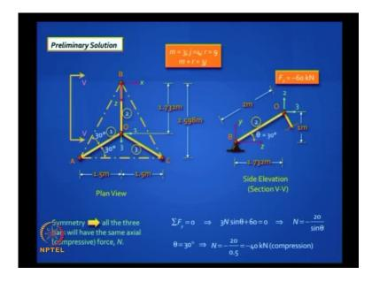
Here is a plan view. I have done the work for you. Here is a side elevation say section V-V. Can you understand what is going on? It is a triangle on the base; it is arrested here; arrested here; arrested here. They are pinned supports. This O is 1 meter above. A, B and C are restrained and I forget about the restrain coordinates. So, I have only three active degrees of freedom. Let me call them 1, 2 and 3. Does it make sense? The tripod 1 up, 2 along the x axis, and 3 along the z axis.
