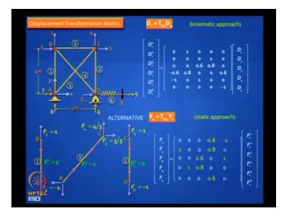
It took a while for you to get the idea of getting the T D A matrix using the kinematic approach. Finally, we got this. You remember? We did it step-by-step. This is actually a very efficient way of doing it because you can program it. You do not have to think. It will do it automatically provided you are clear about the start node, the end node, and the correct value of theta I x.
