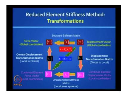
Remember this diagram. This is one way of saying the big picture, global coordinates, local coordinates, structure stiffness matrix, element stiffness matrix and the two transformations. In the stiffness method especially the reduced element stiffness method, your first task is to get the T D matrix correct. You remember that we had some difficulty when we did in the plane truss. Today, I will show you an alternative way of doing it.
