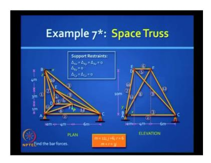
Now, this is a reading exercise. I put a star there. This is a complicated space truss. The triangle D E F is horizontal, but at this height 10 meter above ground. The triangle A B C
