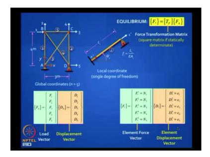
So you can uniquely define t f only for a statically determinate structure because you have a unique statically admissible solution for a statically indeterminate structure you cannot uniquely define t f please note that demonstrate with an example very familiar example this is plane truss you identify the active degrees of freedom there only five of them right one two three four five ah
