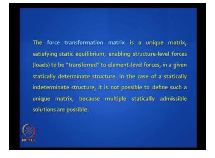
So this is the meaning of force transfer coefficient right the force transformation matrix is a unique matrix satisfying static equilibrium enabling structure level forces or loads to be transferred in inverted commas to element level forces in a given statically determinate structure in the case of a statically indeterminate structure remember it is not possible to define such a unique matrix because multiple statical admissible solutions are possible.
