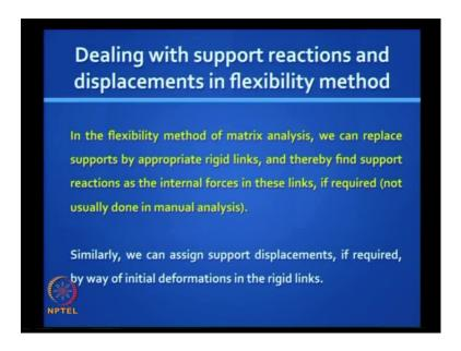
Next point if you want to find support reactions you can do it we will see it later in the flexibility method of matrix analysis we can replace supports by appropriate rigid links so the force in a
