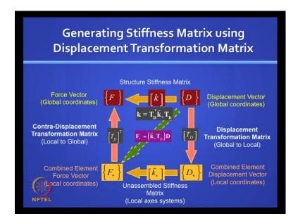
We will see examples of this in trusses later now you got you got the stiffness matrix at the element level you got the t d matrix which relates the element level displacements to the structure level displacements our job is to find the structure stiffness matrix.
