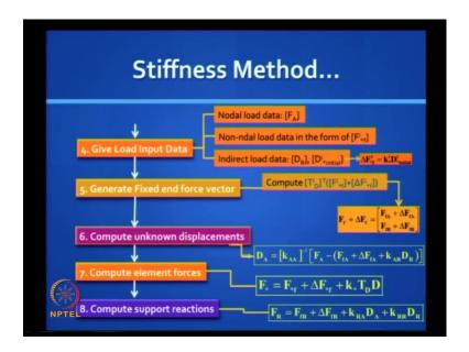
So you will find repeatedly this kind of pattern in merging you have to premultiply the stiffness matrix whether it is a regular stiffness matrix or the conventional stiffness matrix by the transpose of some transformation matrix in this case t d and also post multiply with t d so that is that is what you do when you do this you will get the full stiffness matrix without any effect so that is to sum of the reduced element stiffness method we will go through the details later it
