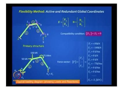
So we are now set to move on to last topic which is the flexibility method the first problem you are notice the main [dis/difference] difference between flexibility and stiffness methods this you
