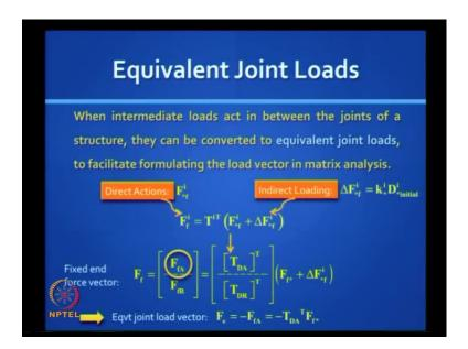
So do you agree i can write down a set of initial displacements either contraction or elongation in a truss and if i just multiplied with the elements stiffness of that i get the fixed end forces we will see this in detail later so you got the local fixed end force vectors for all the elements either cause by direct actions that is intermediate loads or by indirect loading.
