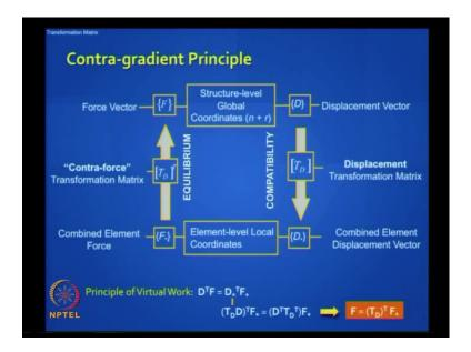
Ah now let us look at the contra gradient principle i have shown this earlier but, here at the lower level i put the element level forces the combined element force vector f star which actually refers in a case of a truss to all the axial forces in the truss the combined element displacement vector d star which are the bar elongations in the truss the structure level displacement vector which are the joint displacement in the in the truss and the structure level force vector f ok.
