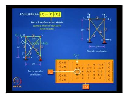
So this is nothing but, the bar force and the internal d one star is nothing but, the bar elongation do you understand what this means everything make sense now we need to generate the t f matrix so let us do that so let us take that matrix apply f one equal to one can we quickly analyze this other any zero bar forces here by inspection tell me which bar force ah.
