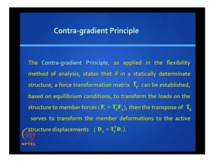
The contra gradient principle as applied in the flexibility method of analysis states that if in a statically determinate structure a force transformation matrix t f can be established based on
