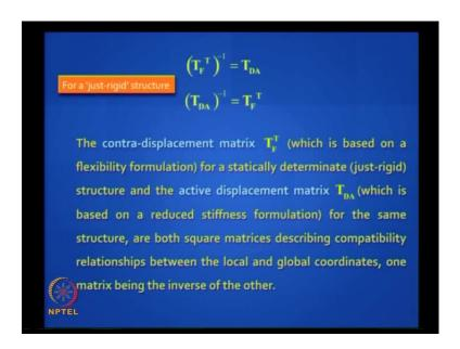
So if you compare now the two transformations you get another interesting result for a statically determinate structure t f transpose inverses t d a and t d a inverse is t f transpose so you can get a potential question in the exam where i give you one of them and ask you to figure out the other you have to bring the same.
