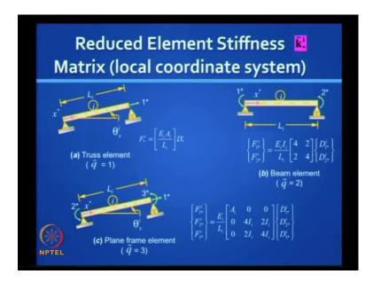
If you recall we know why we in can take advantage of these reduce element stiffness method because the rank of the element the conventional stiffness matrix at the element level is less than full so you can reduce it to the minimum to full rank and we've already discuss three types of elements we will see other types later but, this is elementary so we looked at the truss element you have only one degree of freedom reduced.
