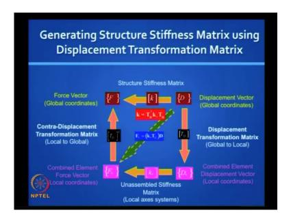
So, let me put it in a different way. If I want to generate the structure stiffness matrix using this approach, the displacement transformation matrix. First, I create this relationship at the element level putting all of them together, so it is unassembled. Is it clear? Exactly, what I have shown on the board.
