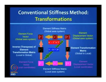
You will recall in the last class, we gave a big picture view ah this picture really shows how you can do various transformations to finely arrive at the arrive at what what is the end result of this? You will get the element stiffness matrix of every element aligned along the global axis ok.
