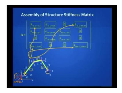
So, all you have to look at is, connectivity. Let me help you, take the first element, the first element is connected to nodes 10, 11, 12 and 1, 2, 3 so all you have to do is, to pick up the appropriate boxes and put them into the slots as shown here, does this make sense? It fills up only those four slots.
