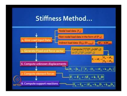
Next, you put in the load data ok and this we will see later you generate the fixed end force vector, you find the unknown displacements by using the inverted K A matrix, compute the element level forces, compute the support reactions, you got everything and all this happens in a jiffy at the press of a button but, inside the black box ah, we are trying to see what is inside the black box and how is it working?
