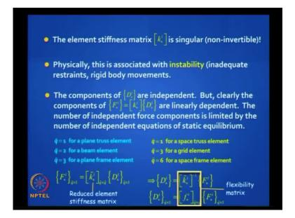
One is for the truss, its 3 ok why it is 3? You should figure out by, you can multiply you know they are all dependent, they are not independent ok. So, here is a summary of it, the element stiffness matrix is singular, non invertible. Physically, this is associated with instability, inadequate restraints, rigid body moments. The components of D i are independent but, clearly the components of F i star are linearly dependent. The number
