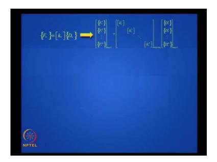
Ah before that, let me talk of this matrix K star, which is sometime refer to as the unassembled stiffness matrix ok. Ah let me give you a simple example: let us take a truss.
