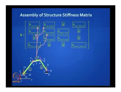
Ah element one has no contribution elsewhere in that big picture in that global, take element two, where do you think it will fit in? It will fit in that simple, the top corner because 1, 2, 3, 4, 5, 6 element coordinates match with, global structure coordinates 1, 2 so that is simple and the last one, last one will connect 4, 5, 6 and 7, 8, 9. Does it make sense?
