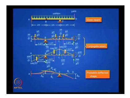
This is the given beam and this is the conjugate beam. In the conjugate beam, the boundary conditions are as shown. Now, instead of putting on that beam that big complicated diagram, it is good to separate out the curved parts from the straight-line parts, just for simplicity in calculation. If you do that and you do superposition, you can actually find out the centroids of the resultant forces and analyze it.
