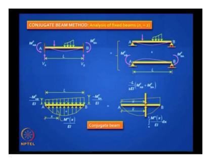
I think we are running out of time. Accidently, the conjugate beam method also gives a method for solving some types of indeterminate problems where the indeterminacy is not more than 2. For example, take this fixed beam. How do you find the fixed end moments in this beam? You can visualize this as a simply supported beam with the original loading plus the hogging fixed end moments. If you draw the conjugate beam for this,
