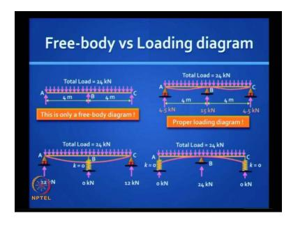
At this point, I want you to realize that when we draw diagrams like this, we tacitly assume that A, B, and C are support locations; that is, these are reactions, but this diagram does not reveal anything and it is necessary to know how to distinguish between a free-body diagram and a loading diagram. This is only a free-body diagram. If you want a loading diagram, then this would be the correct picture to draw (Refer Slide Time: 14:38).
