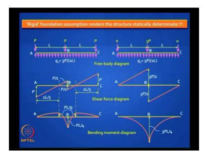
The answer is you do not need to have jumped into the assumption of a two-span continuous beam, because the moment you assumed the rigid foundation assumption, you have got a free body which is complete by itself. Can you not draw a shear force and bending moment diagram from the free body? This is the confusion that is there in many engineers. You mix up things – you mix up free body with loading diagram. Once you have got a free-body diagram that is all that you need; you have got the statics
