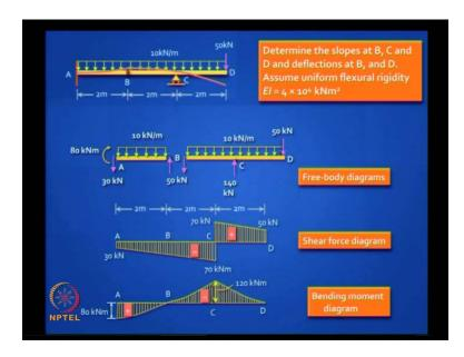
A little more complicated problem; here, I will quickly rush through it. It is little complicated because you have got propped cantilever with an internal hinge and you are ask to find the slopes at B, C, and D and deflections at B and D. It is difficult, but the easiest way you can solve such a difficult problem is the conjugate beam. Let us go through the steps.
