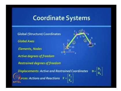
This is to refresh your memory. Please see what the real task for us is - we want to be able to make the digital computer do structural analysis. We want, first of all, to have a framework in which we show the structure geometrically, which means, we have to identify the elements and nodes with reference to some Cartesian coordinates.
