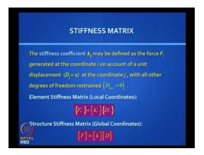
Now, we look at stiffness matrix. We already know the definition K ij; it is called the stiffness coefficient. It is the force F i generated at the coordinate i on account of a unit displacement D j equal to 1 at the coordinate j, with all other degrees of freedom restrained; you are very familiar with this definition.
