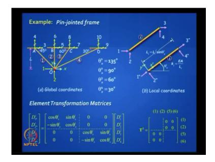
Let us give an example. This is a pin-jointed truss - pin-jointed frame. How many active degrees of freedom, do you think there are? It is a plane truss (Refer Slide Time 26:44).
