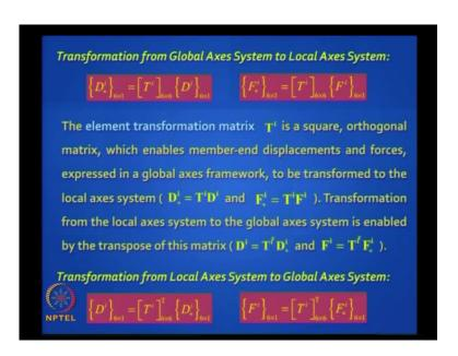
These are the fundamental transformations. The element transformation matrix T i is a square, orthogonal matrix, which enables member end displacements and forces, expressed in a global axes framework, to be transformed to the local axes system. Transformation from the local axes system to the global axes is enabled by the transpose of this matrix, which is equal to the inverse of the matrix; you can switch back and forth.
