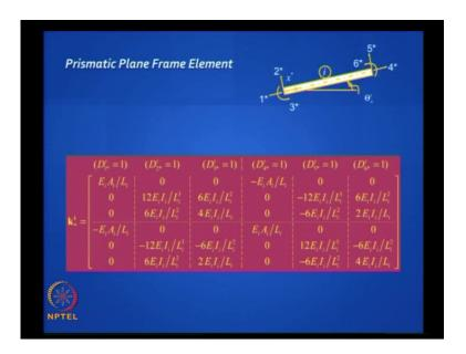
You can fill up this matrix. Here, it is a function of E I - remember 4 E I by L, 2 E I by L, 6 E I by L square, 12 E I by L cube - that is all that you can get. If you have a plane frame element, you will have a combination of the truss and the beam; we will see this later.
