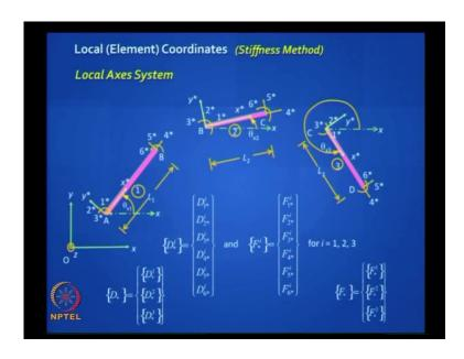
Next, you will recall, we defined the - local coordinate - local axes. In this particular plain frame, for example, you have three elements and we have the local coordinates - the local axes. You have 6 degrees of freedom per element, so you have the element displacement vector, the element force vector and we use some superscripts and subscripts to clarify.
