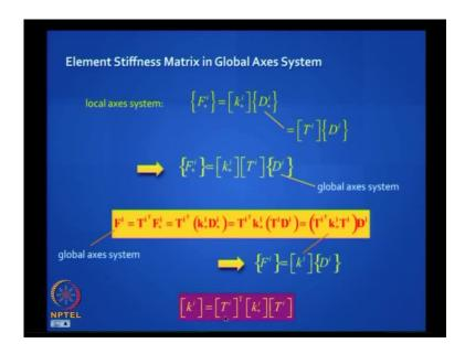
This is 6 by 6; right now it is an introduction, you should know that you have these elements stiffness matrices. Now the challenge for us is we have got the transformation matrix, we have got the elements stiffness matrix, they are properties of the dimensions of the element, length of the element and the E and A or E and I values, how do I get the elements stiffness matrix in the global axes system? Not for the structure, I am still sticking to the element.
